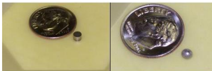
Tc/Zr sample before and after arc melting
