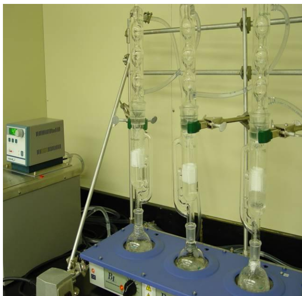
Soxhlet apparatus to compare corrosion resistance and to determine long-term behavior.
