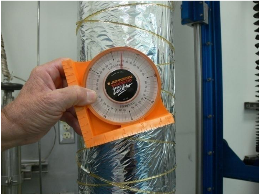
Figure 3-13. Design 1 test article with helically wrapped spacer rods.
