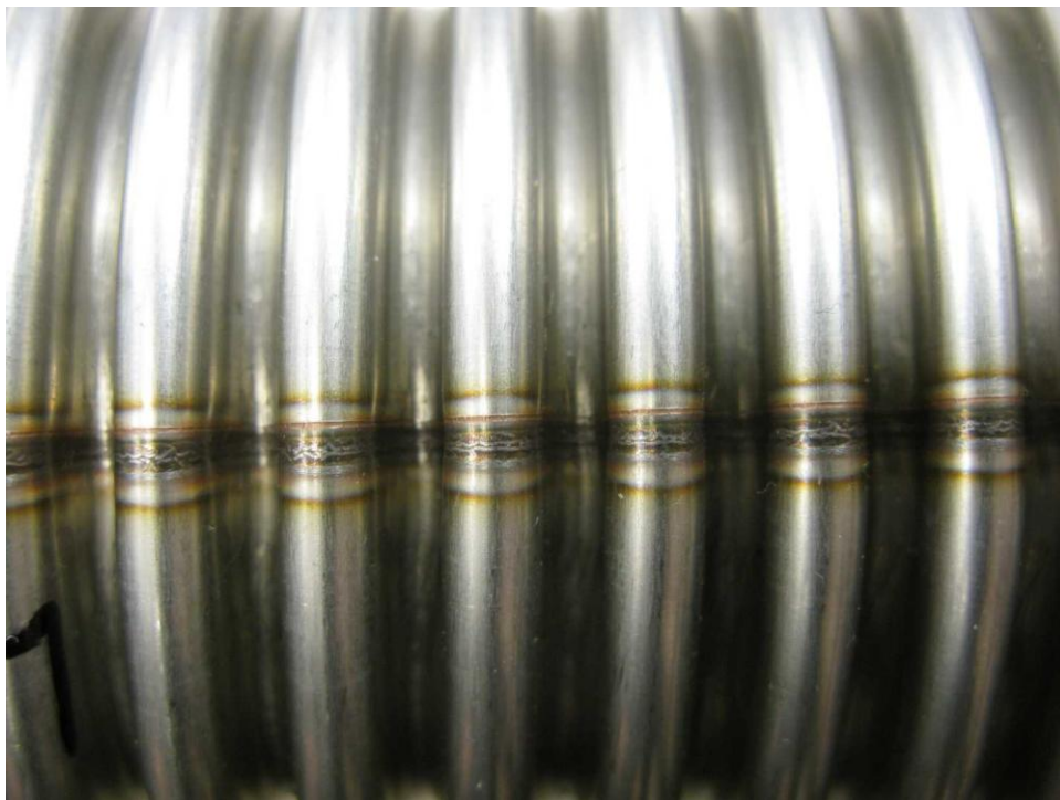
Figure 3-8. Flex pipe weld seam.
