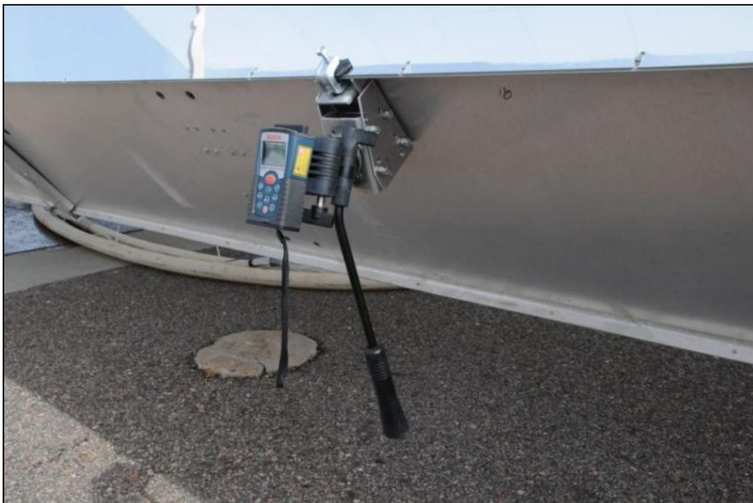
Figure 51: Laser Distance Meter used to conduct initial receiver tube alignment (Photo courtesy of NREL)
