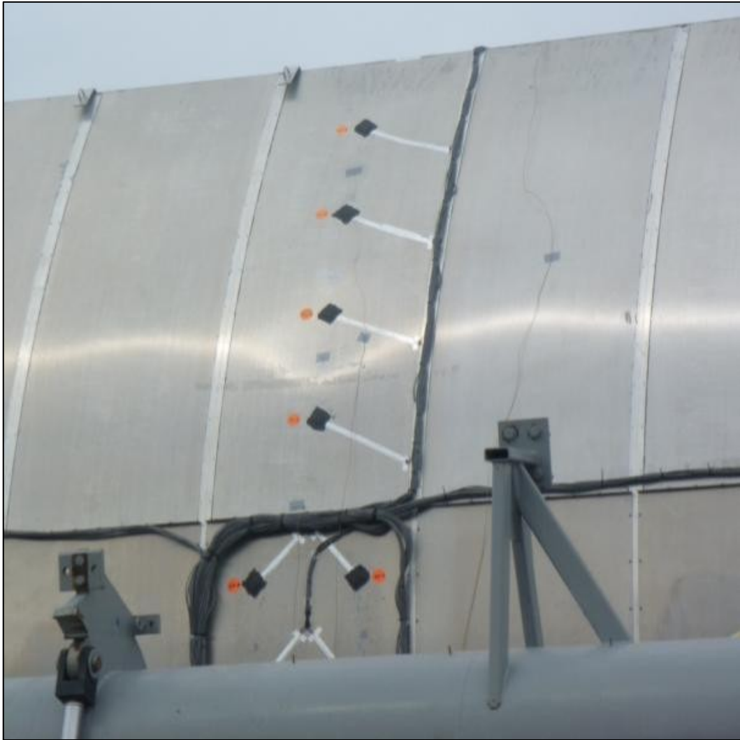
Figure 73: Strain Gauges Placed on Back of Trough
