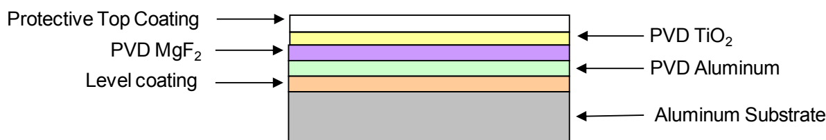
Figure 2: Cross-section of Thin Film Technology Option
