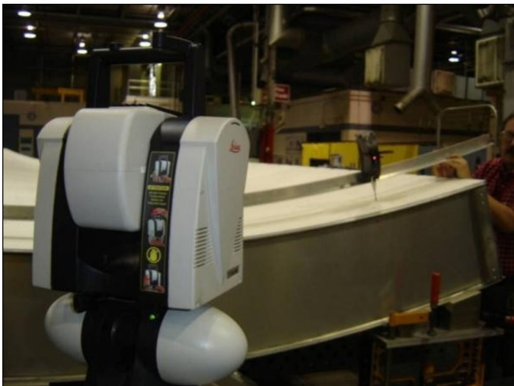
Figure 43: GD&T validation of trough half module assembly via laser tracker
