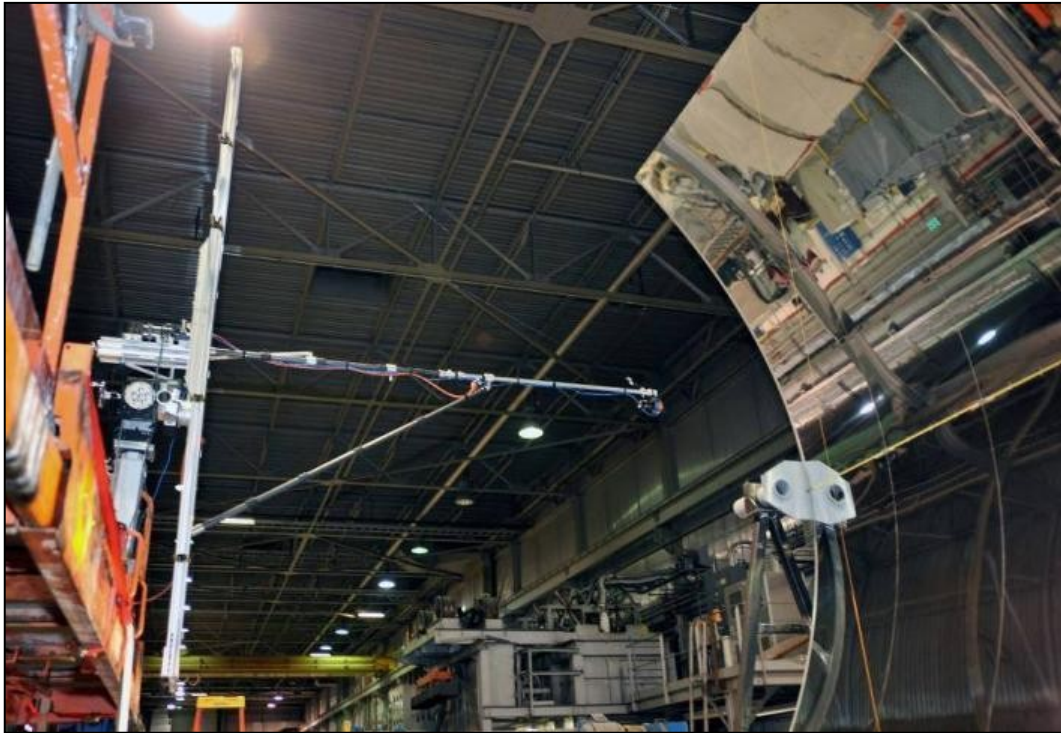
Figure 47: VSHOT testing of the whole trough at Alcoa
