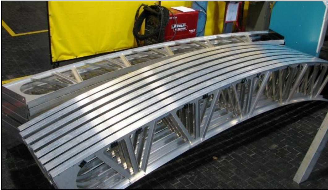
Figure 34: Rib sub-assemblies after final inspection
