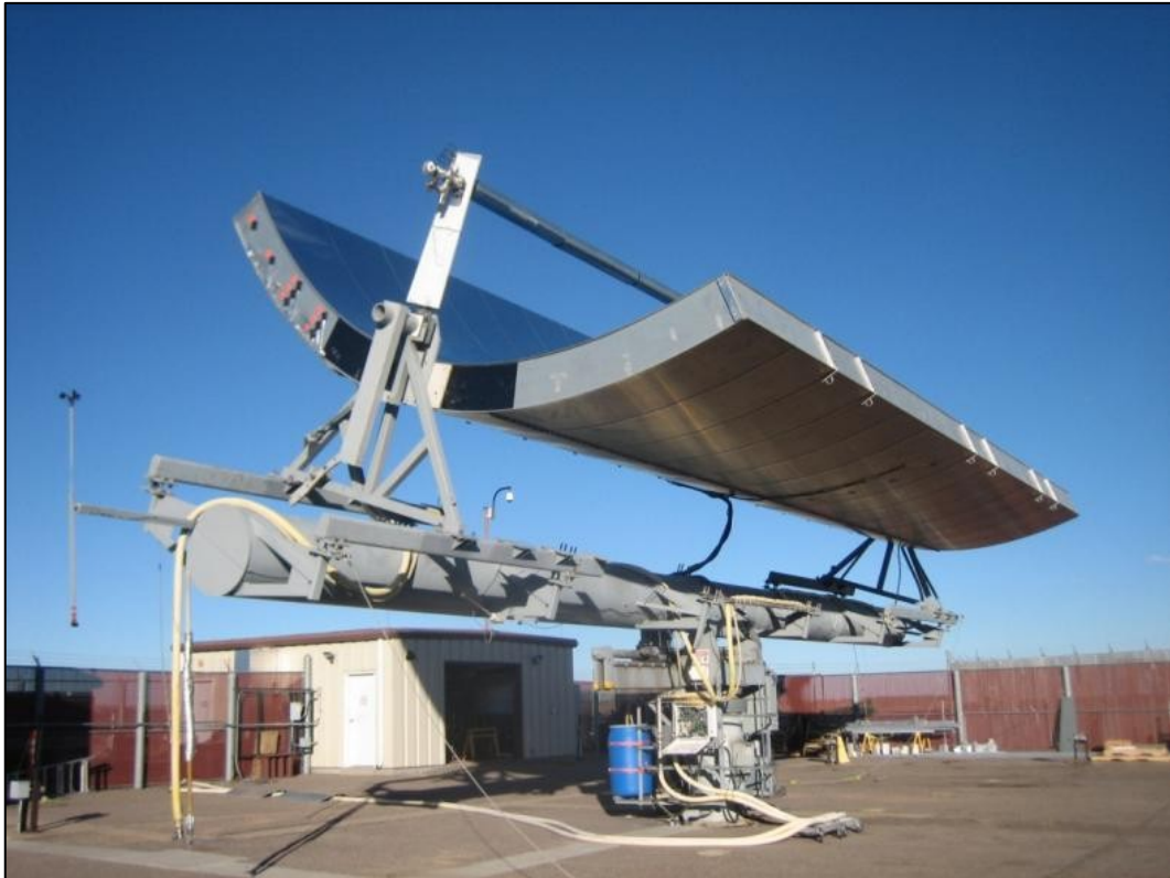
Figure 50: Trough mounted to NREL's two axis tracker
