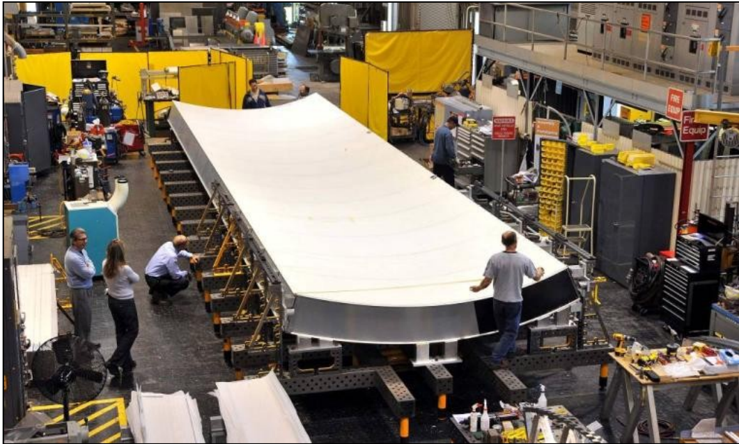
Figure 36: Half module fabrication at ATC
