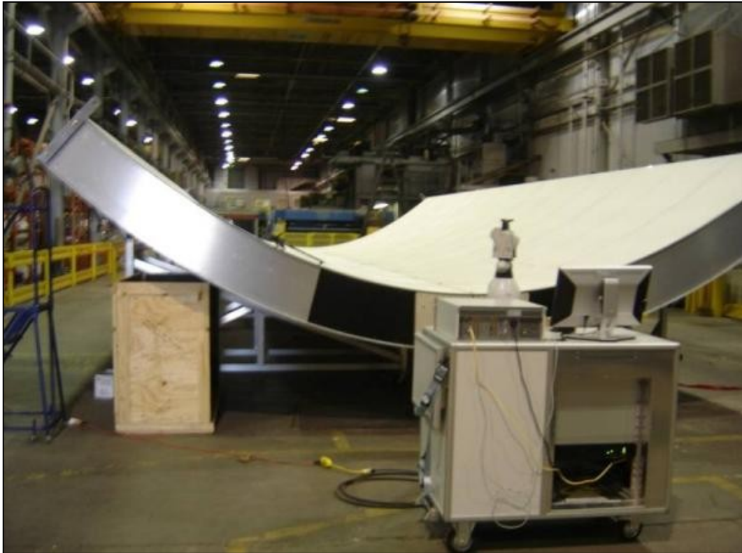
Figure 44: GD&T validation of trough via laser tracker
