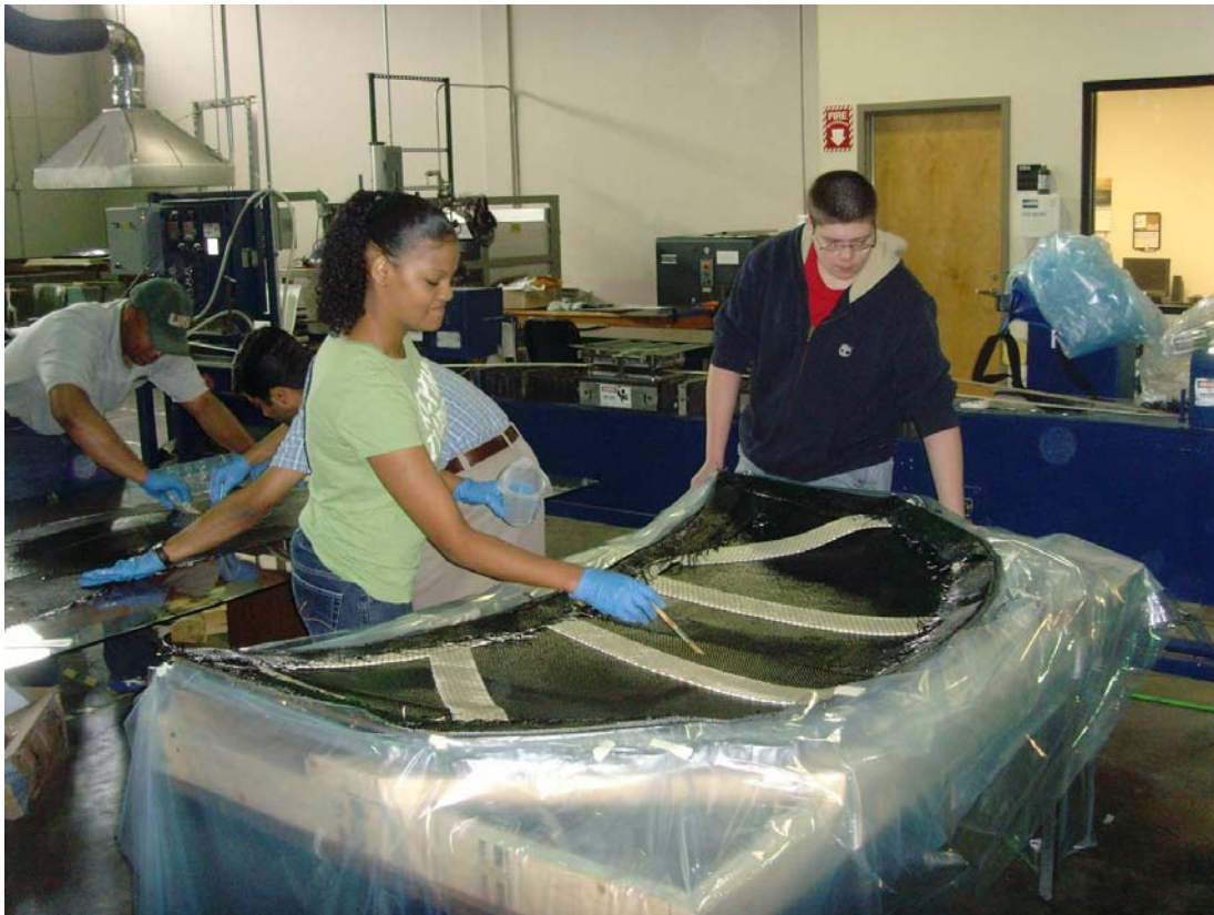
Figure 7. GATE researchers Hadeel Abdelmajeed and Daniel Kaliberov laying up the carbon fiber Odyssey hood at UAB.
