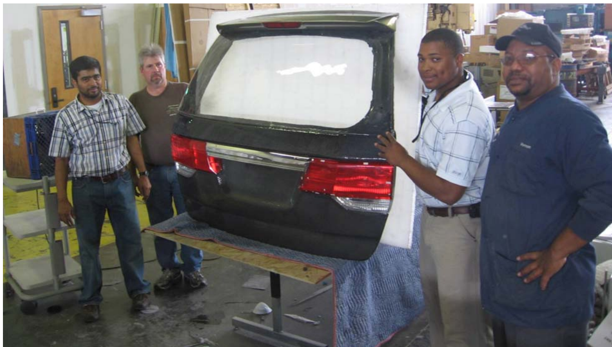
Figure 11. Carbon Fiber Tailgate – 44 lbs with all components (the metal tailgate weighs 74 lbs. GATE researcher Walter Malone and Krishan Thattai parthasarathy.
