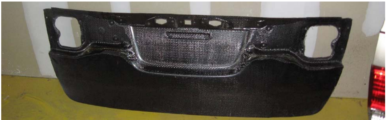
Figure 9. Honda Odyssey tailgate component fabricated using carbon fiber by the GATE fellows.
