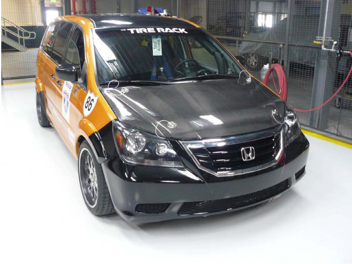
Figure 8. The UAB fabricated carbon fiber hood weighed 8 pounds as opposed to 28 pounds for the steel component it replaced.
