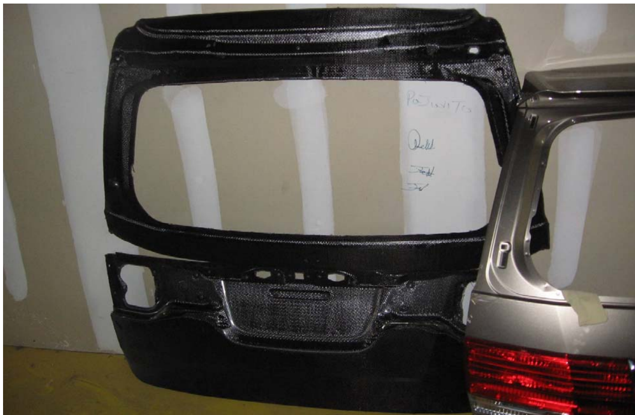
Figure 10. Carbon fiber components of the tailgate fabricated by UAB GATE fellows.
