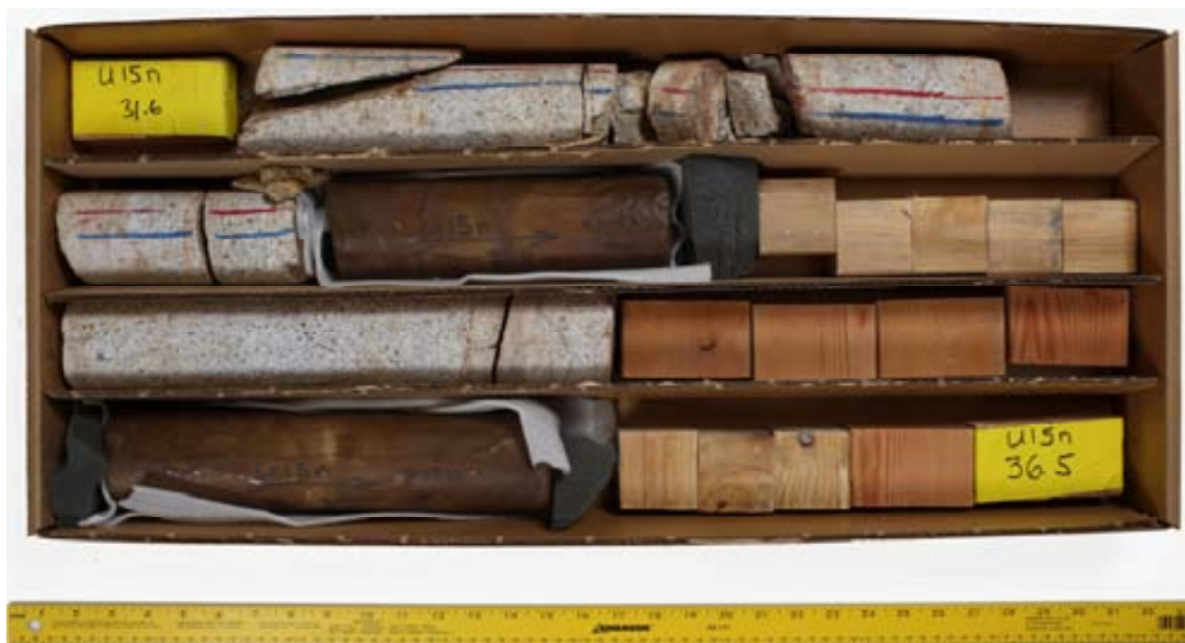
Depth interval 9.6 to 11.1 m (31.6 to 36.5 ft) below ground surface. Brown samples are preserved in beeswax.
