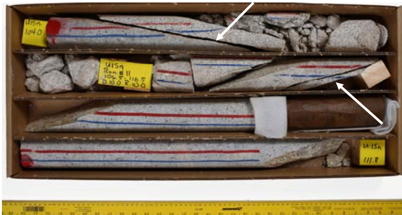
Depth interval 31.7 to 34.1 m (104.0 to 111.8 ft) below ground surface. Includes the lower fault zone (indicated by arrows)
