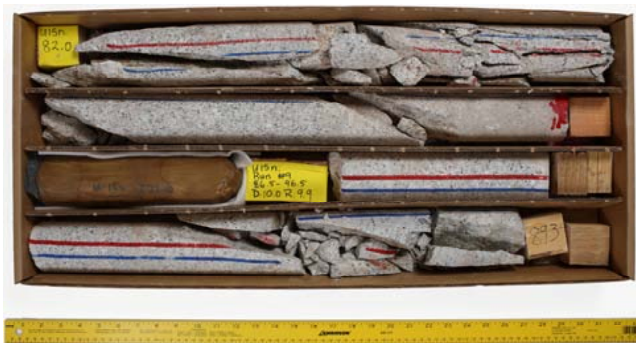
Depth interval 25.0 to 27.2 m (82.0 to 89.3 ft) below ground surface. Includes part of the upper fault zone.
