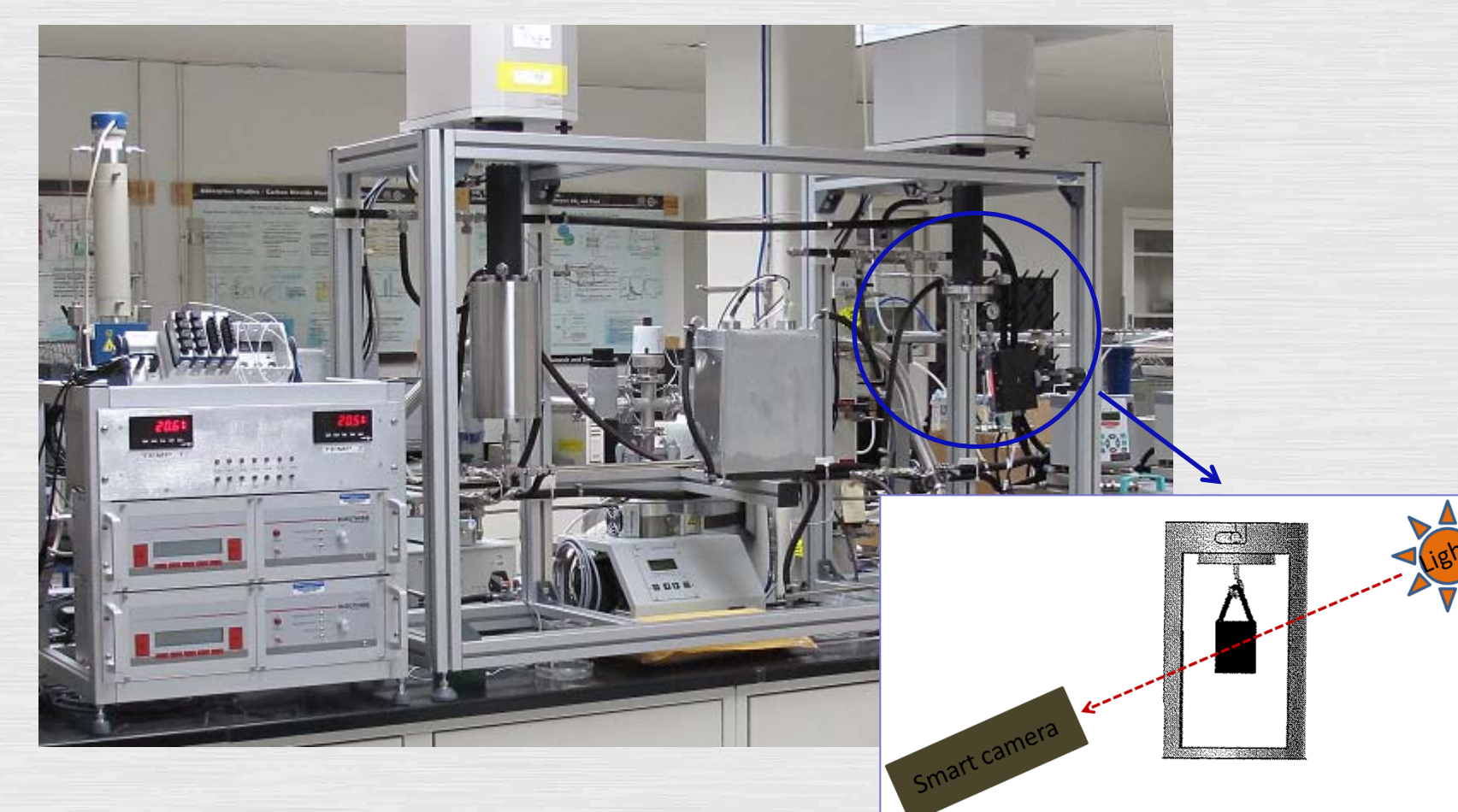
Fig.4. Constructing a gravimetric apparatus that has a visual window cell. It may improve an accuracy of sorption isotherms and provide feasibility for the observation of structural deformation of coal.
