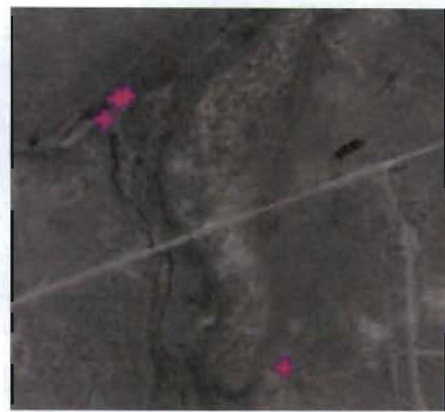
Figure 4. Examples of successful classification of the areas surrounding the detected corners as nonman-made areas. Detected corners are shown with magenta "+". No areas are highlighted because man-made areas were not detected. Image credit: ©Google Earth.
