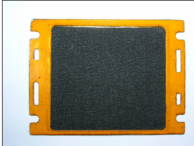
Figure 2.7 Membrane electrode assembly
