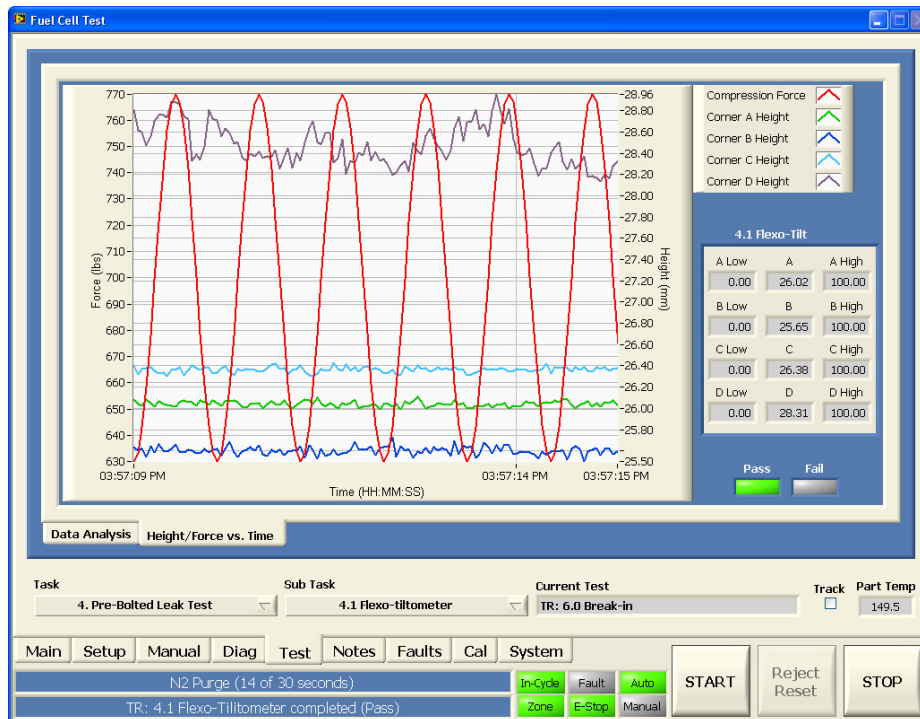
Figure 5.10 Test screen: Flexo-tiltometer test result
