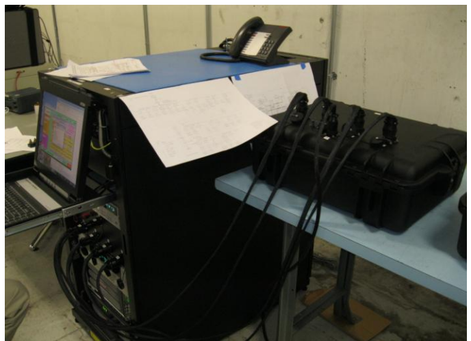
Figure 18 Completed Batteries Integrated with Slave BMU and Test Equipment
