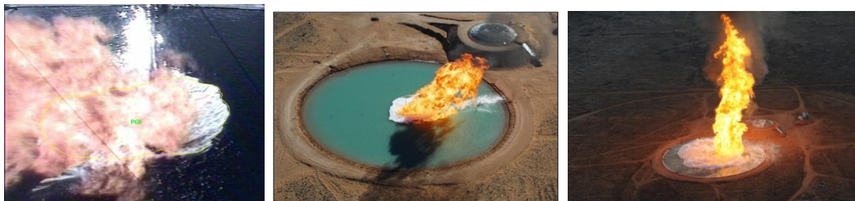
Figure 6: Occurrence of non-burning regions shown for the 10-m, 21-m, and 83-m pool (56 m fire) SNL tests.
