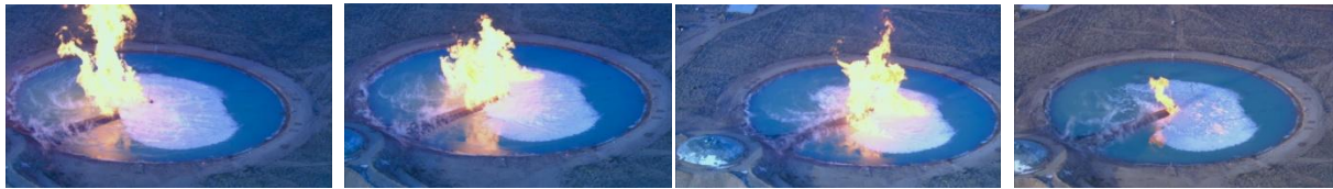
Figure 8: Sequence of late-time burning of the hydrates during the 83-m SNL test resulting in a 56-m fire.
