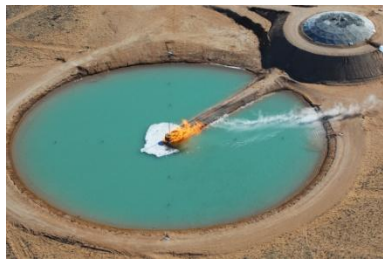
Figure 9: Post-test hydrate layer in the 21 m SNL test.
