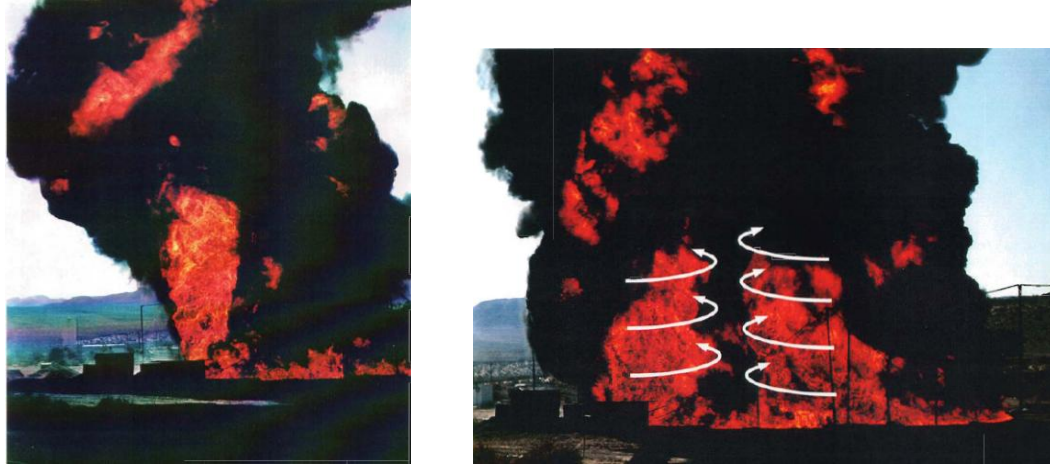
Figure 7: Fire whirls forming on the downwind edge of an 18.9 m JP-8 pool fire in a 2-4 m/s wind (Tieszen 1996).
