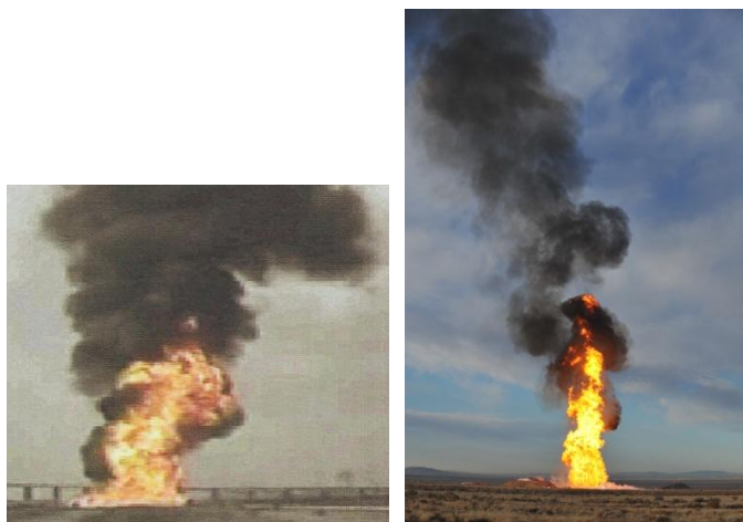
Figure 4: Montoir 35 m LNG pool fire on land (left) and SNL 56 m LNG pool fire on water (right).
