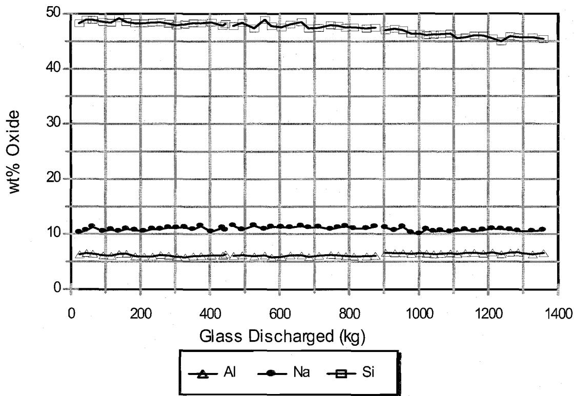
**Figure 10.b. Alumina, soda, and silica concentrations determined by XRF in glasses from Tests A, B and C.**
