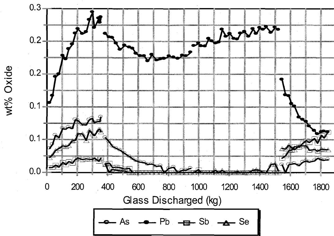
**Figure 12.a. Select toxic metals concentrations determined by XRF in glasses from Tests W, X, Y and Z.**
