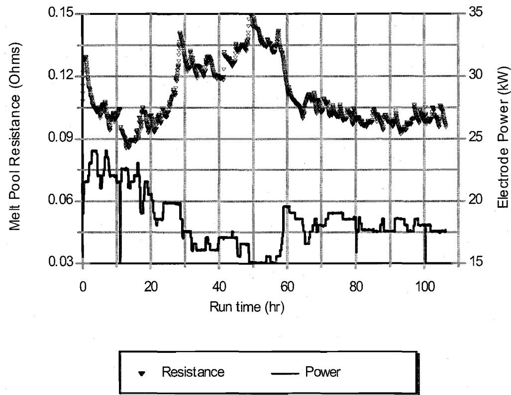
**Figure 8. Glass resistance and electrode power during DM100 Test W.**
