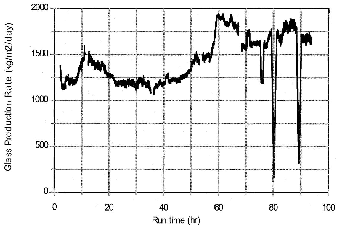
**Figure 2. Glass production rate (hourly averaged) during DM100 Test X.**
