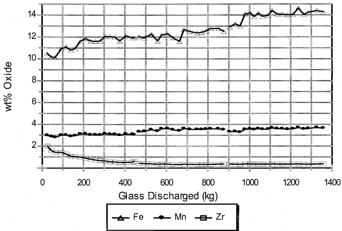
**Figure 11.b. Iron, manganese, and zirconium oxide concentrations determined by XRF in glasses from Tests A, B and C.**
