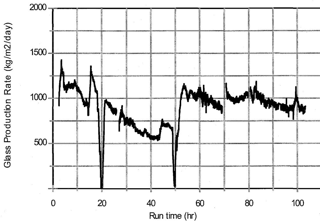
**Figure 4. Glass production rate (hourly averaged) during DM100 Test Z.**
