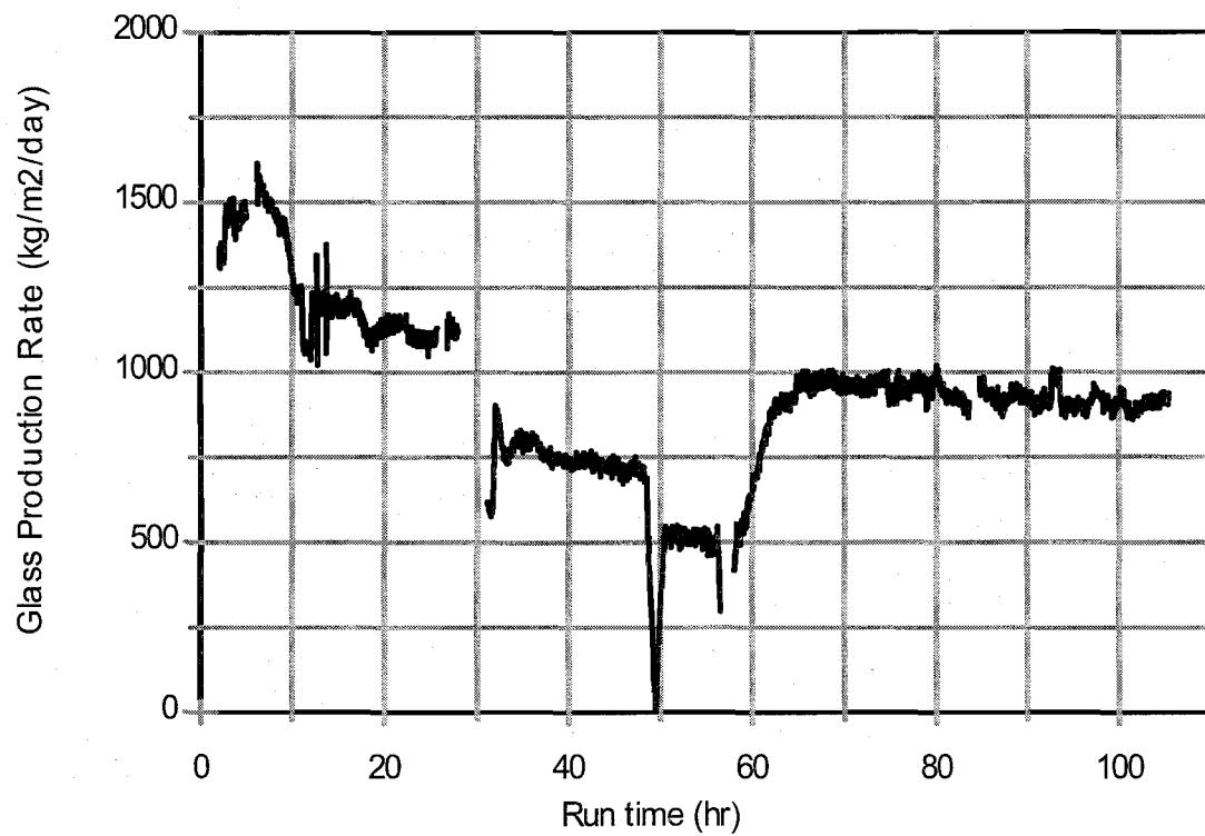
**Figure 1. Glass production rate (hourly averaged) during DM100 Test W.**
