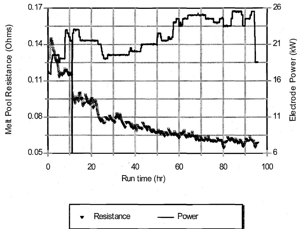
**Figure 9. Glass resistance and electrode power during DM100 Test X.**
