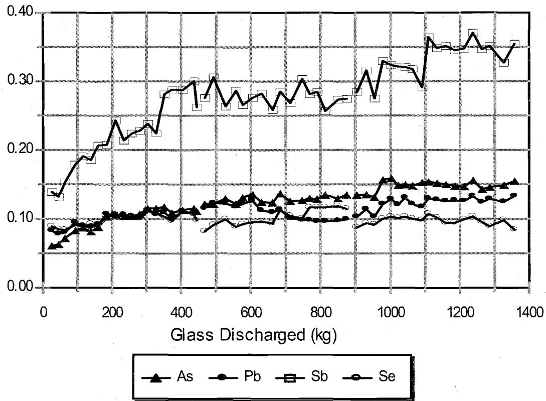
**Figure 12.b. Select toxic metals concentrations determined by XRF in glasses from Tests A, B, and C.**
