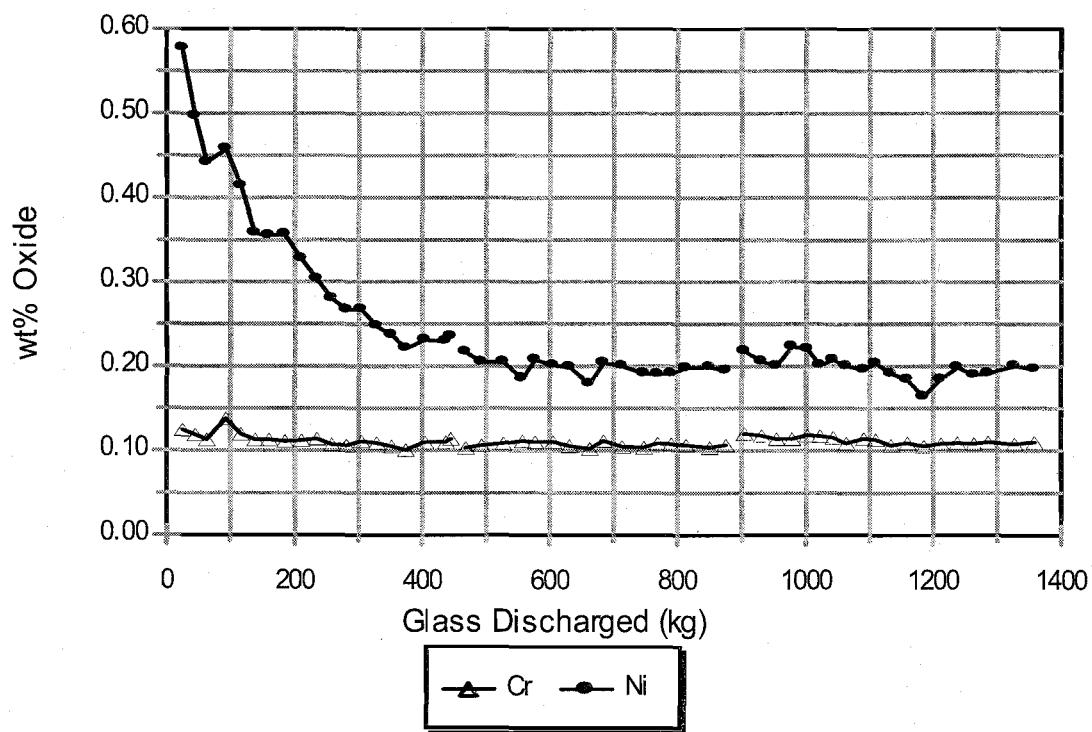
**Figure 13.b Chromium and nickel oxide concentrations determined by XRF in glasses from Tests A, B and C.**
