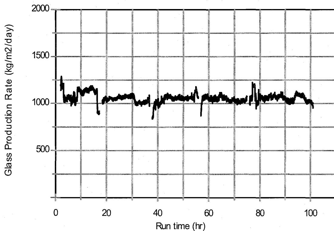
**Figure 7. Glass production rate (hourly averaged) during DM100 Test C.**
