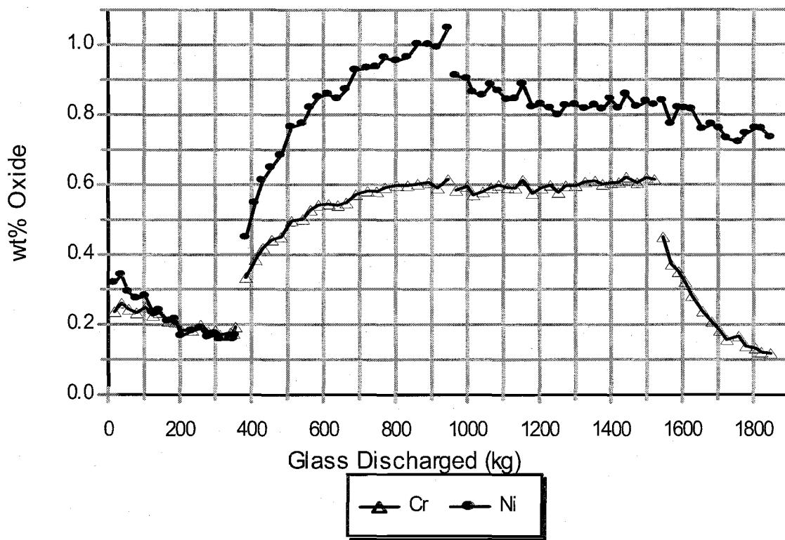
**Figure 13.a. Chromium and nickel oxide concentrations determined by XRF in glasses from Tests W, X, Y and Z.**
