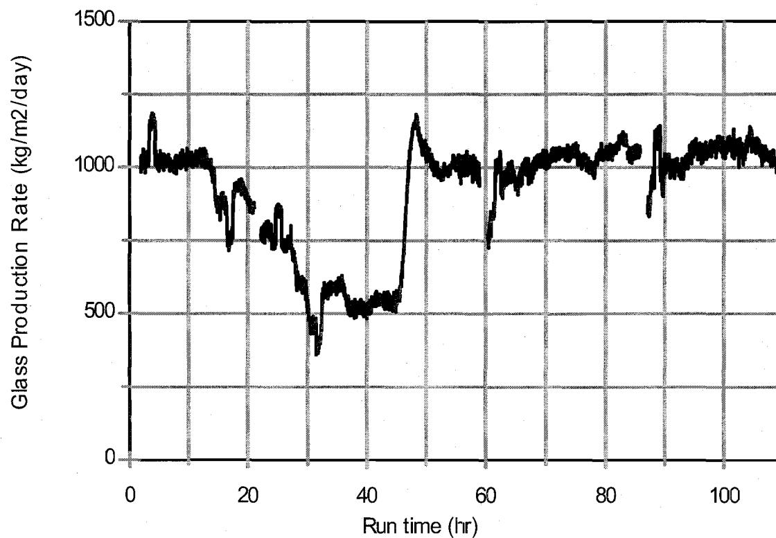
Figure 6. Glass production rate (hourly averaged) during DM100 Test B.
