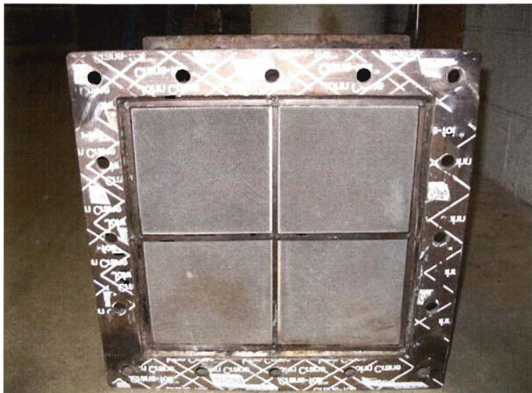
Figure 5.70. View of the outlet of used TCO catalyst section #2 after Test 1.
