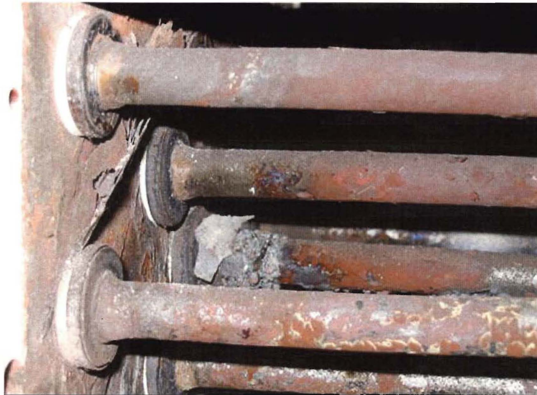
Figure 5.73. Close up of Heater 801 showing failed heating element after Test 1.
