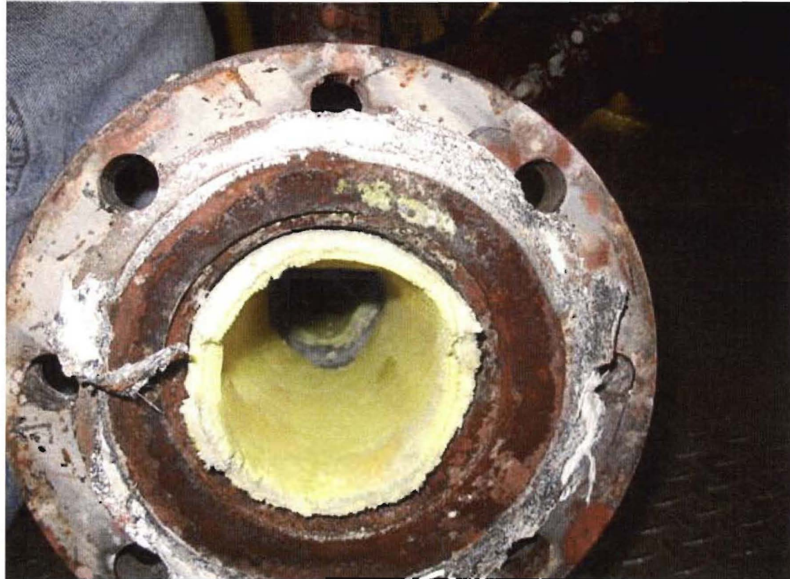
Figure 5.96. View of EOG piping/flange at melter connection after Test 2A.
