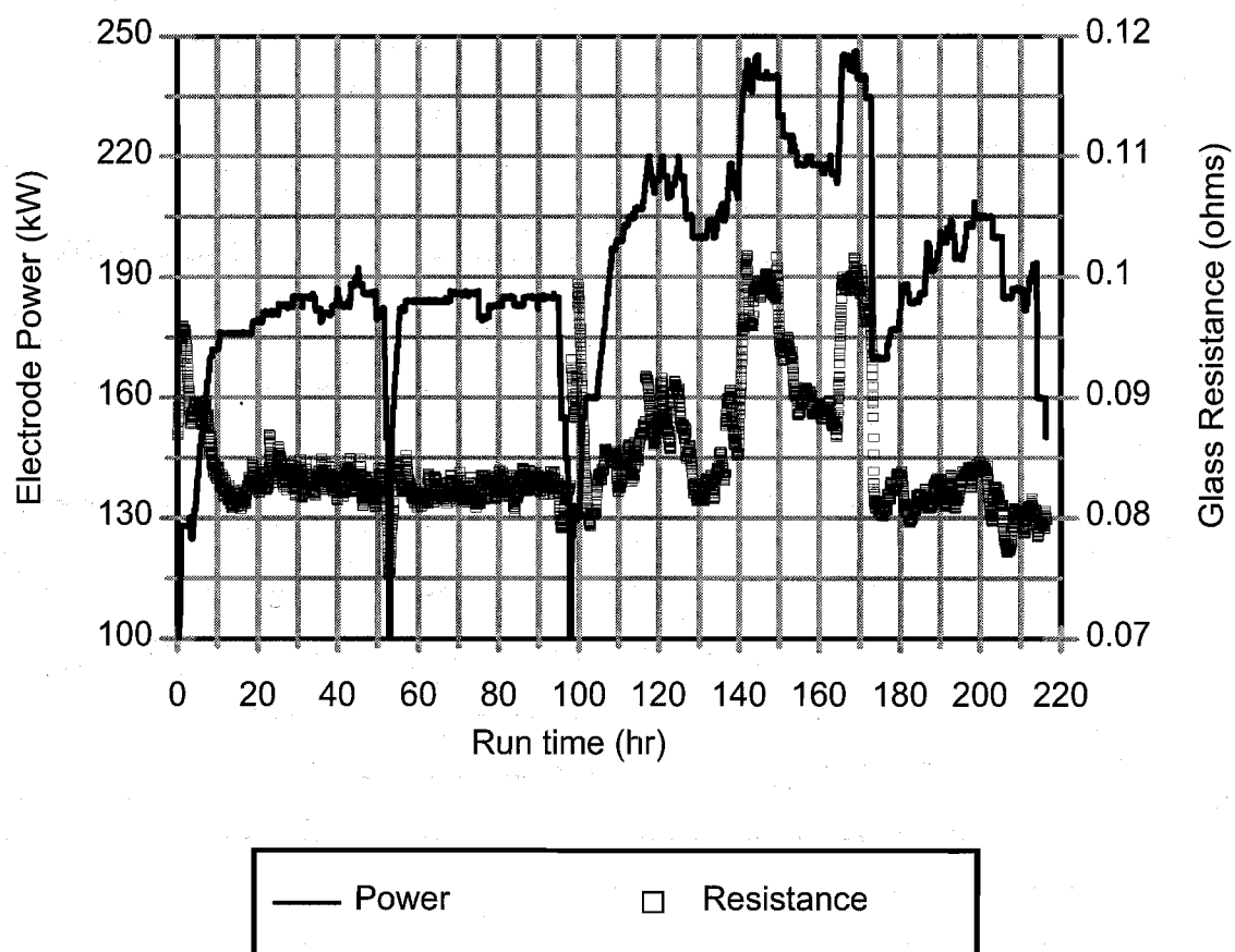
Figure 4.5.a. Electrode power and glass resistance for AZ-102 DM1200 Test (Test 1).
