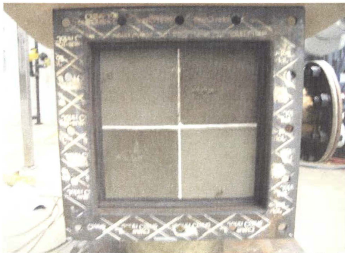
Figure 5.77. View of the inlet of TCO catalyst (Engelhard Corp. VOC CAT 300S 200 CPSI) section #1 before Test 2B.
