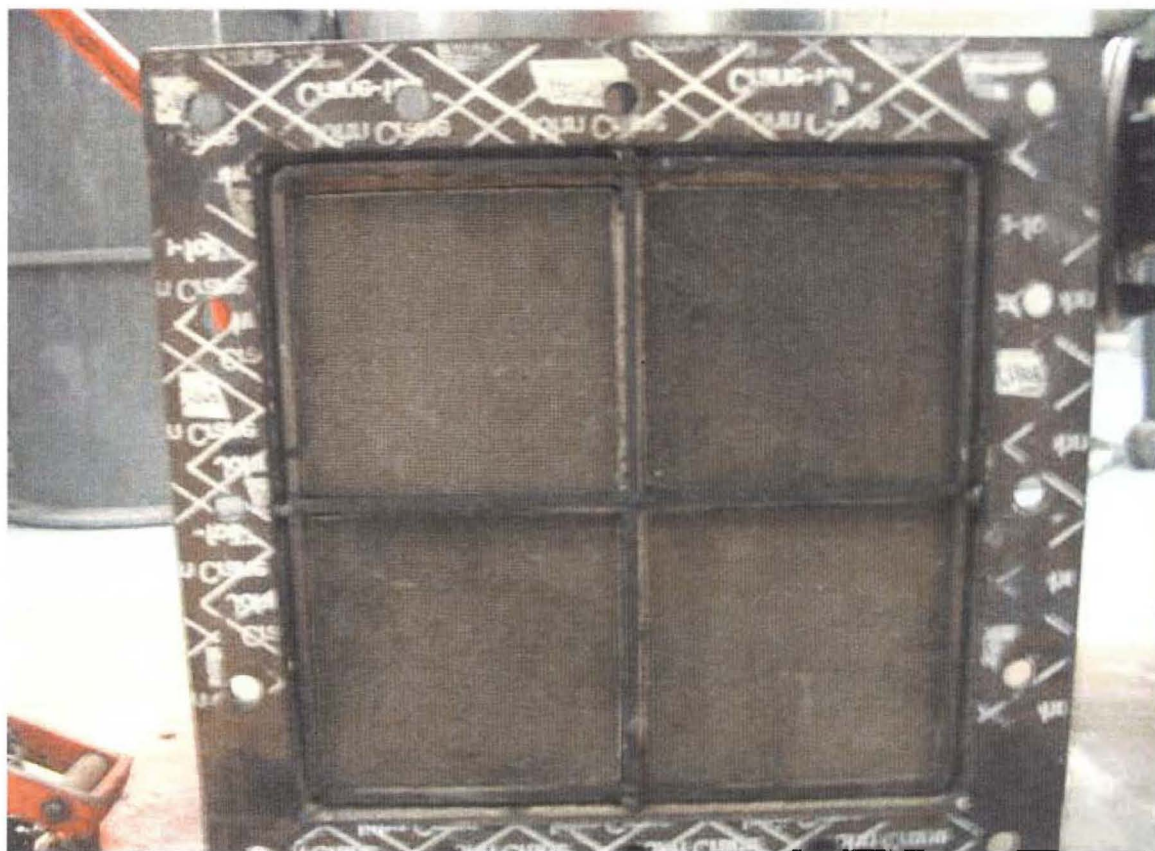
Figure 5.80. View of the outlet of TCO catalyst (Engelhard Corp. VOC CAT 300S 200 CPSI) section #2 before Test 2B.
