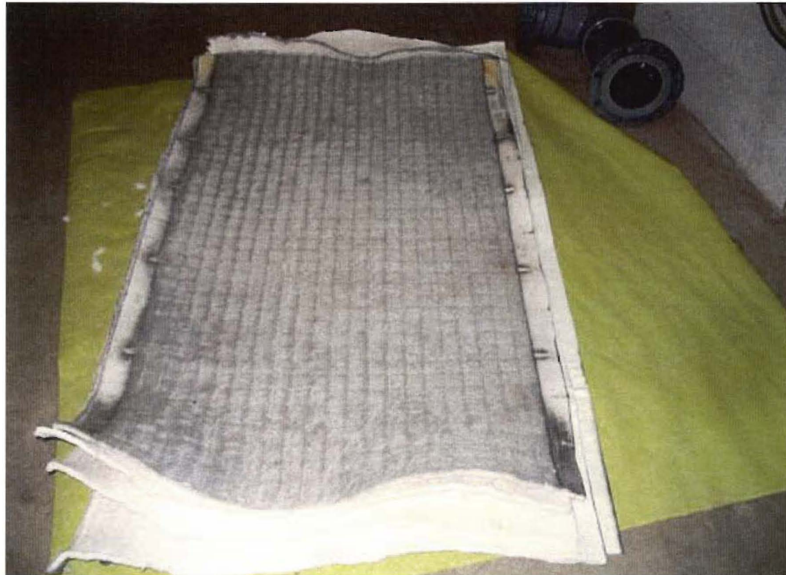
Figure 5.93. View of the inner surface of HEME 2 filter media after Test 2A.
