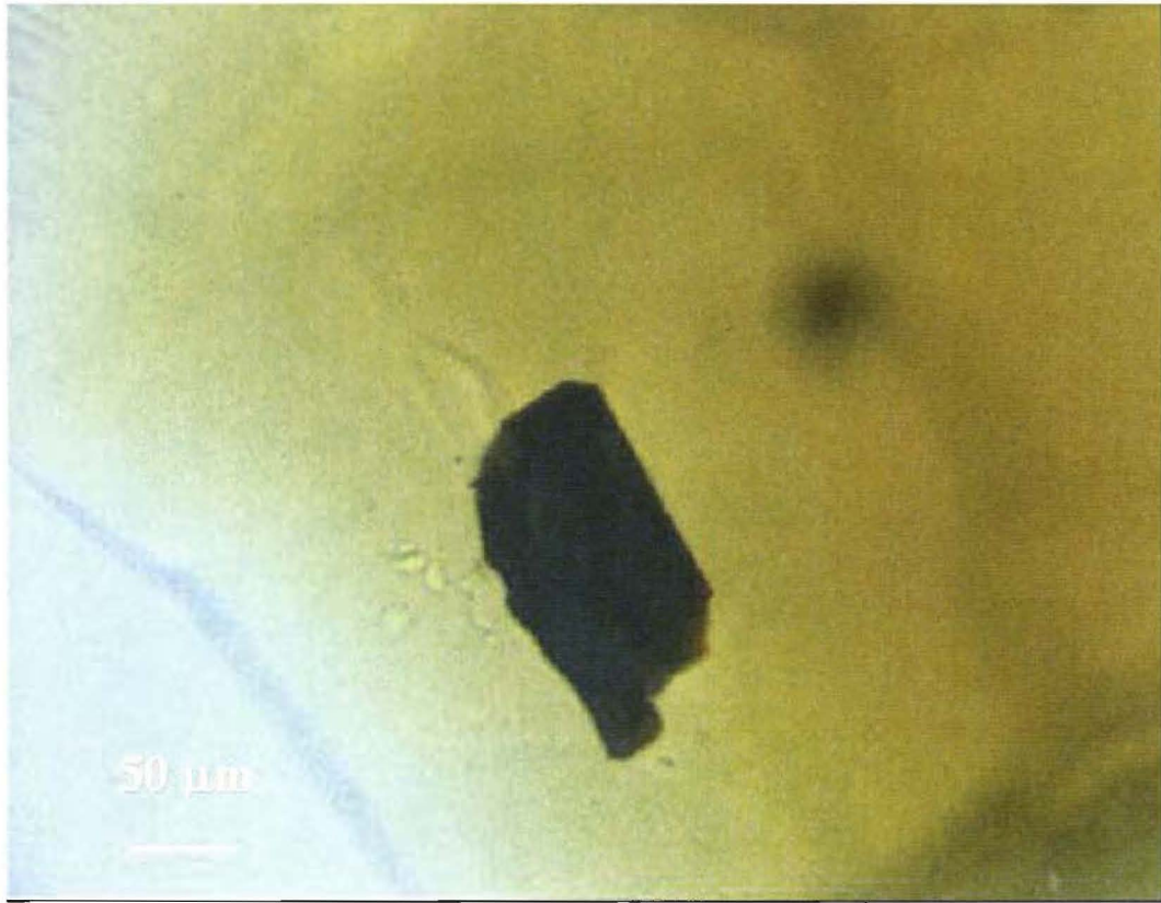
Figure 3.16. Optical micrograph of spinel crystals in glass (BLK-O-41A) from the DM100 riser after 177 days of idling.
