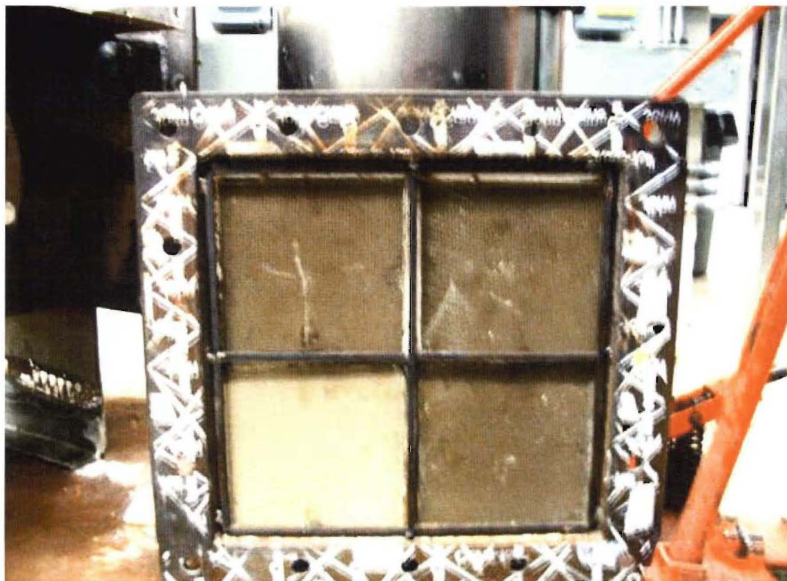
Figure 5.79. View of the inlet of TCO catalyst (Engelhard Corp. VOC CAT 300S 200 CPSI) section #2 before Test 2B.
