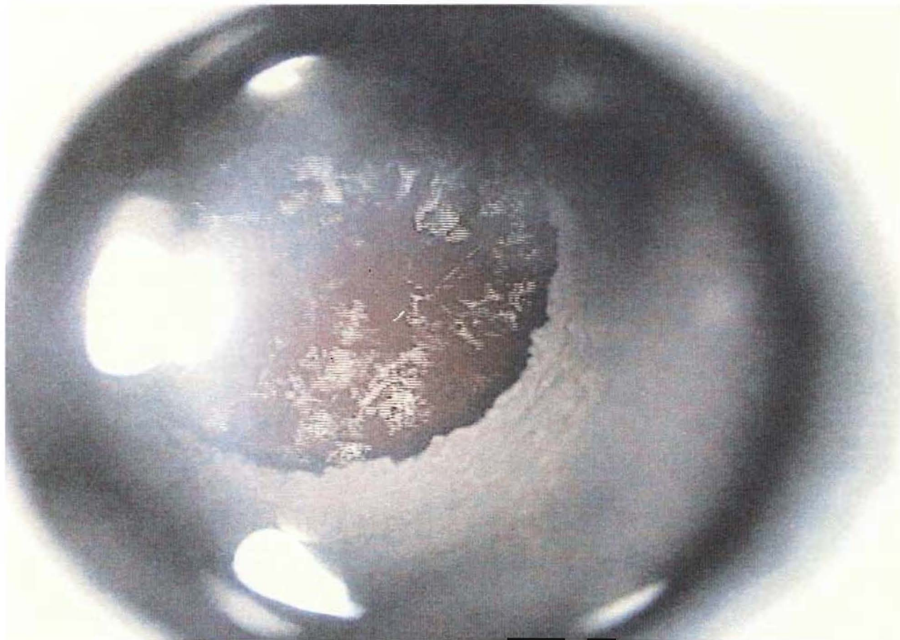
Figure 5.21. View from the inside of the bottom of the SBS downcomer at 192 hours.
