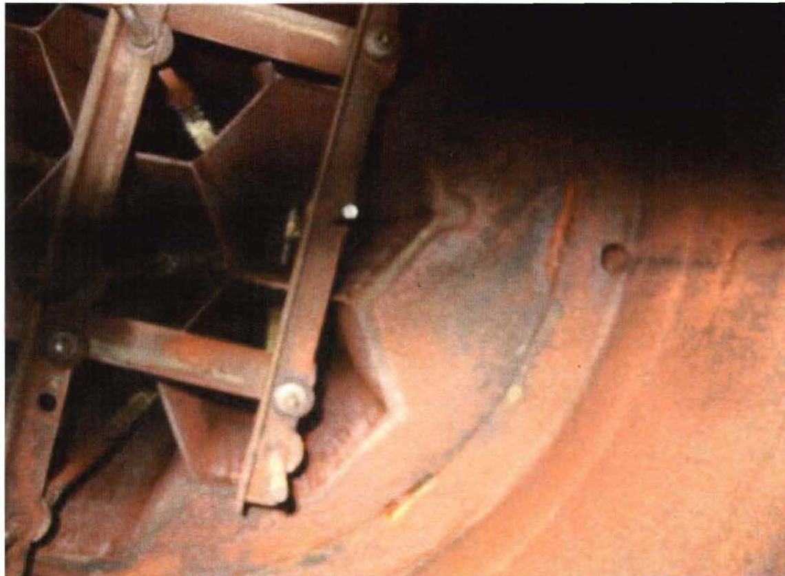
Figure 5.50. Pre-deluge view of WESP rod and collector plate after Test 2A.
