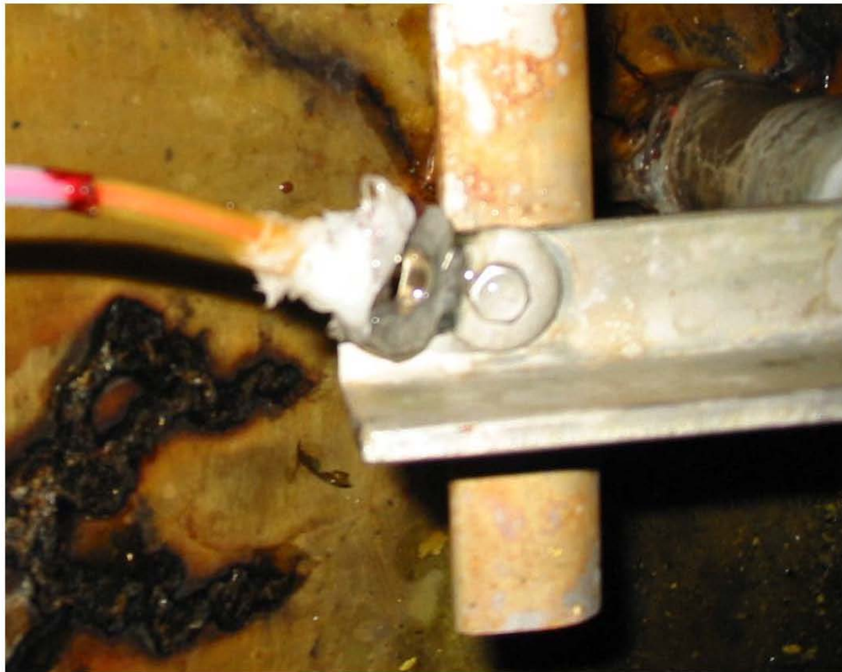
Figure 5.95. WESP power supply wire connection after Test 6.
