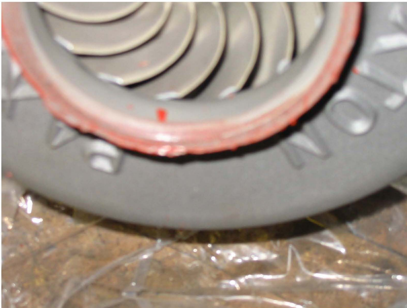
Figure 5.113. View of the blower 701 intake impeller with mushroomed edges due to friction after Test 3.
