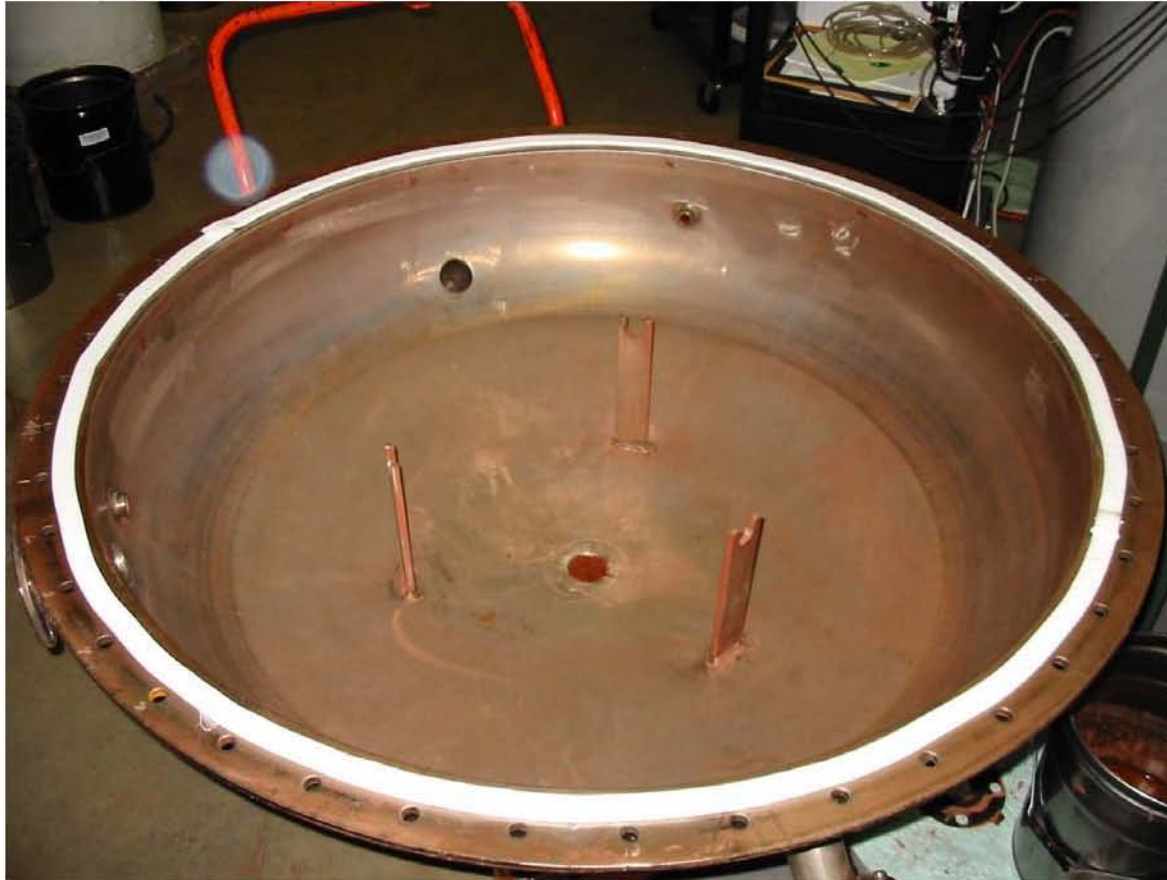
Figure 5.64. SBS bowl after cleaning after Test 5.
