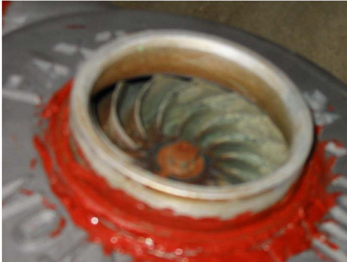
Figure 5.110. Post failure view of the blower 701 inlet port after 121.2 hours of operation during Test 1.
