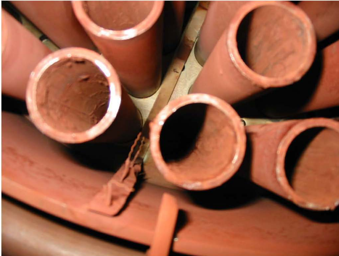
Figure 5.34. Additional view of weir tubes at various locations following cleaning after Tests 1 and 2.
