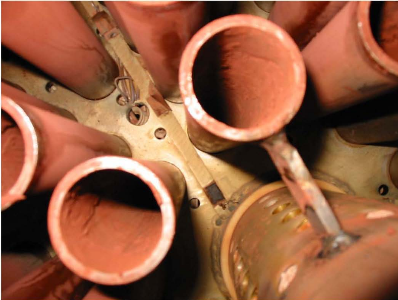
Figure 5.33. View of weir tubes at various locations following cleaning after Tests 1 and 2.
