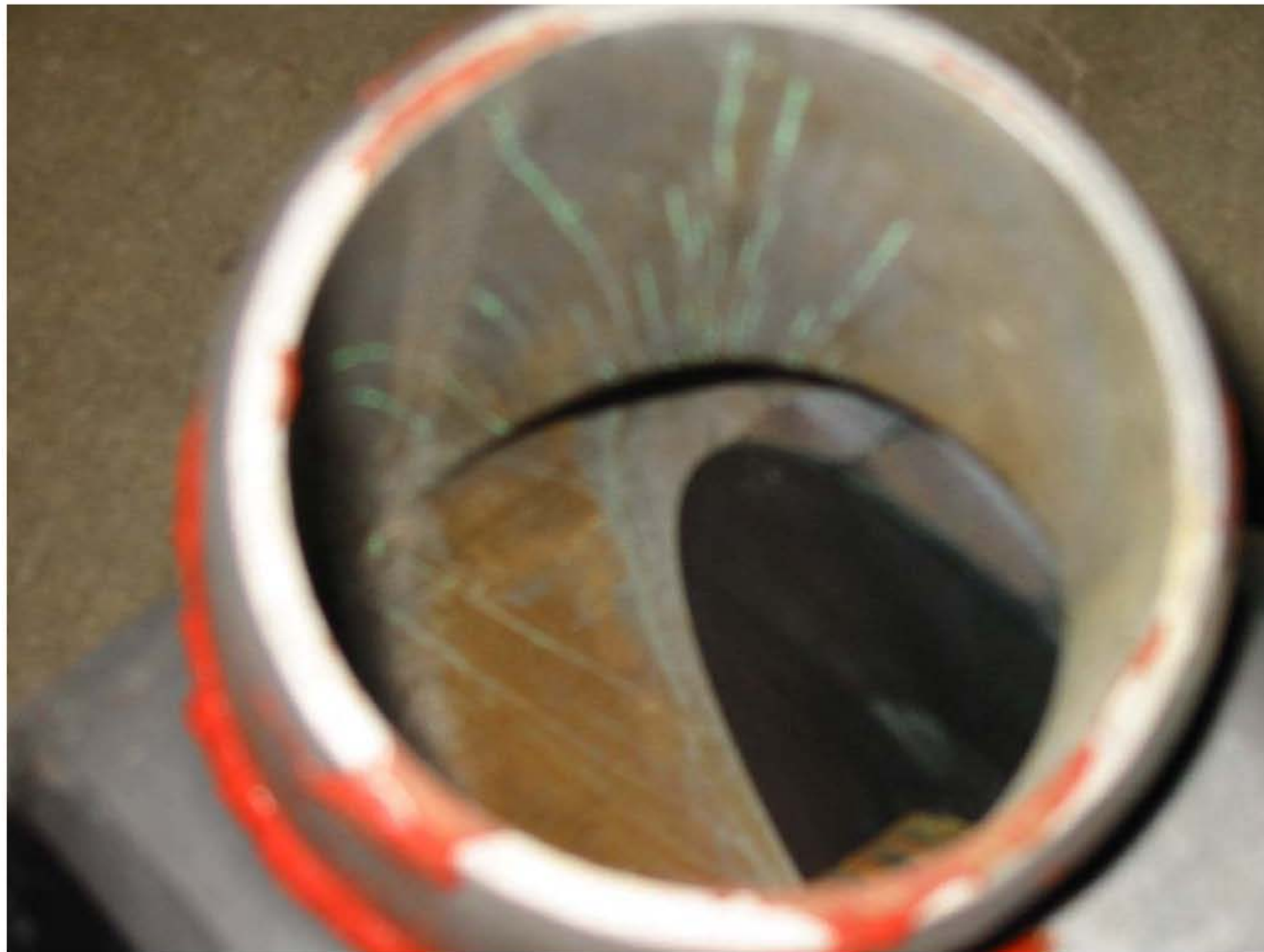
Figure 5.111. Post failure view of the blower 701 outlet port after 121.2 hours of operation during Test 1.
