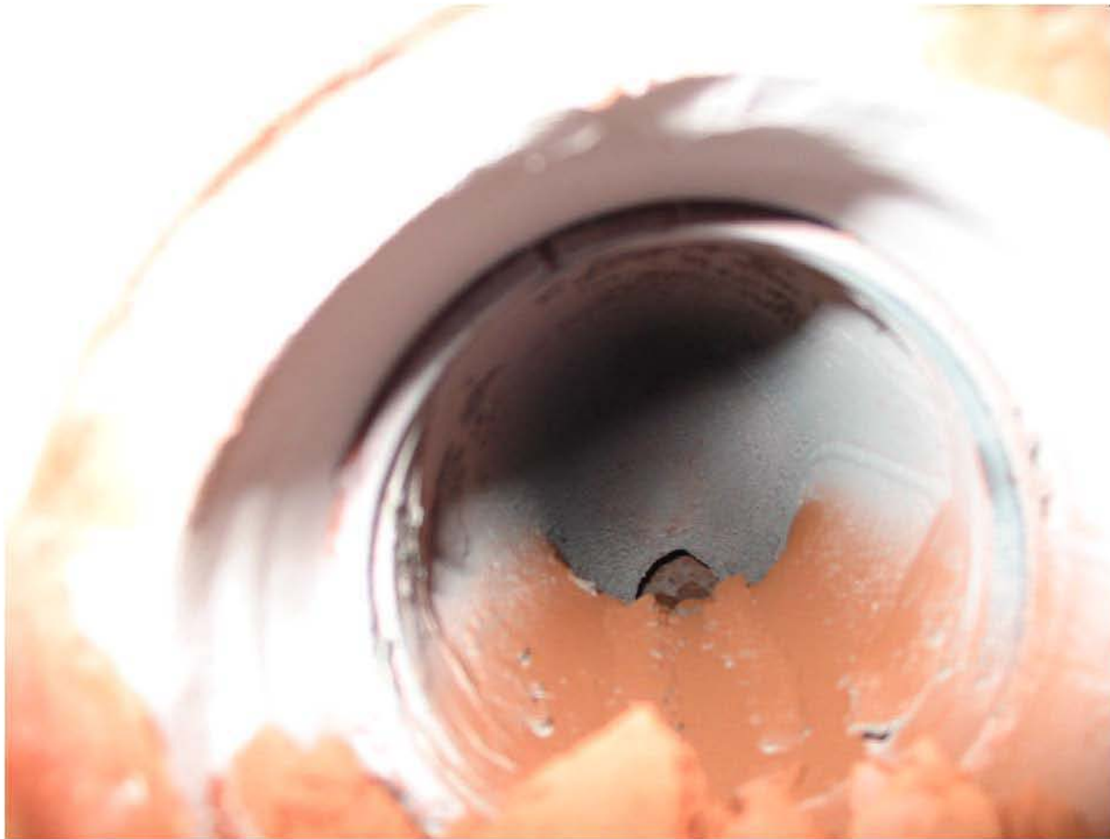
Figure 5.16. Another view of the deposited solids in the transition line outlet on SBS side after Test 5.
