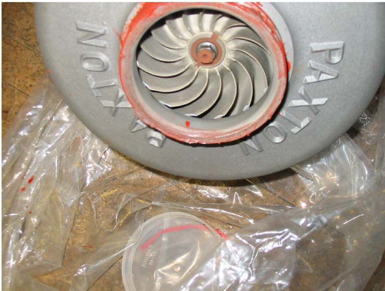
Figure 5.114. Another view of the blower 701 intake impeller with mushroomed edges due to friction after Test 3.
