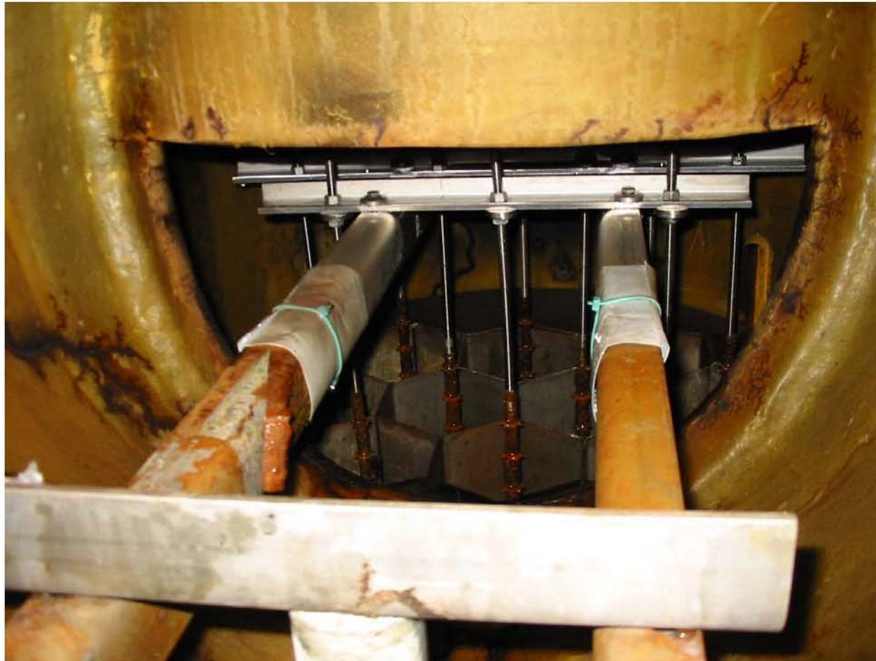
Figure 5.94. WESP overall view of grid after Test 6.
