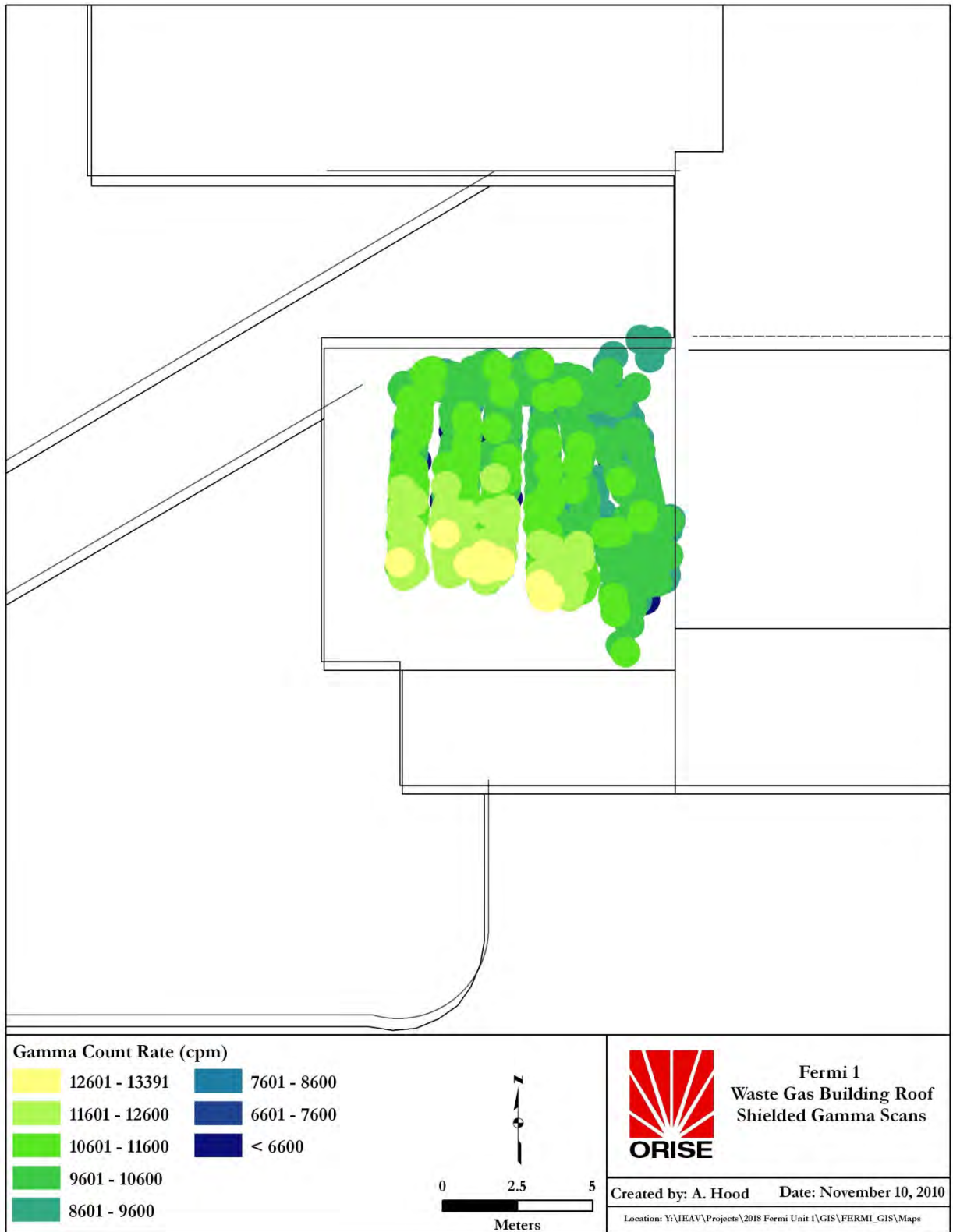
Figure A-13: Waste Gas Building Roof—Shielded Gamma Scans
