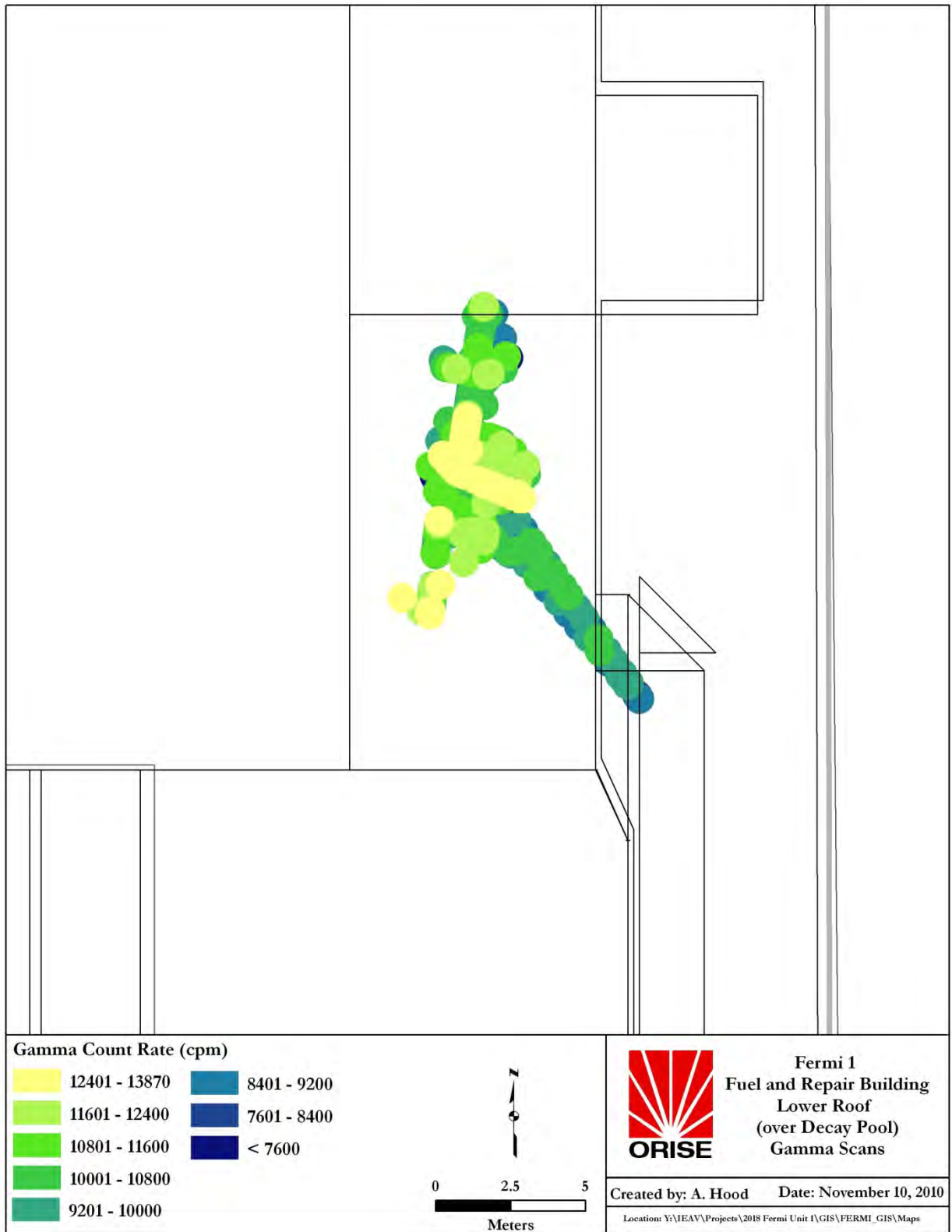
Figure A-9: Fuel and Repair Building, Lower Roof Over Decay Pool—Gamma Scans
