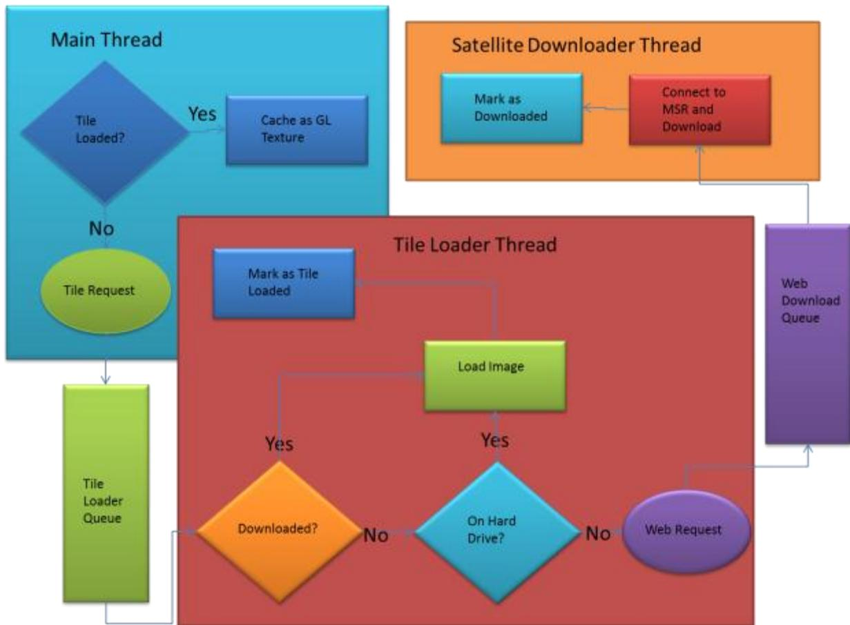
Figure 13.3: Satellite Loading Algorithm
