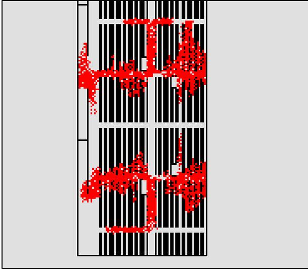
Figure 8.22: High density of entities next to exits in the simulation in Legion
