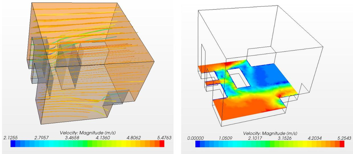
Figure 10.5. Urban Air Flow Predicted by the Model: Boundary Condition: (East, Top, North, South = pressure outlet)
