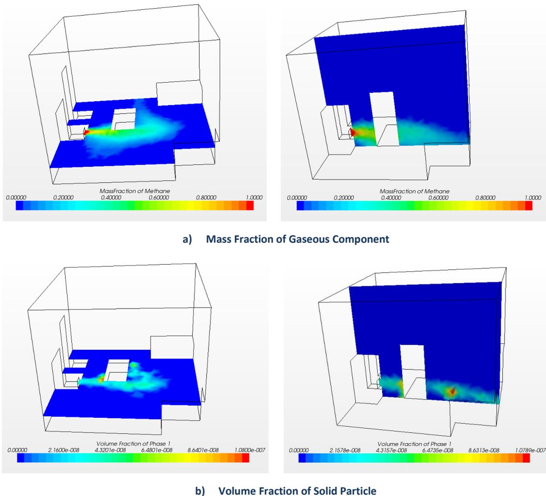
Figure 10.9. Steady State Plume Dispersion upon Gravity Effect (particle size: 100  $\mu\text{m}$ )
