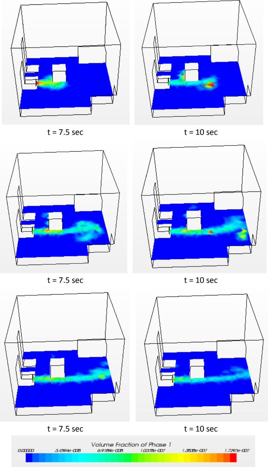
Figure 10.8. Transient Plume Dispersion (Mass Fraction of Methane) Predicted by Multi-Component, Multi-Phase Flow Model
