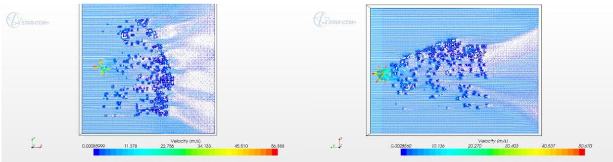
Figure 5.28: Comparison of Block plume inlet (left) and Cylinder plume inlet (right). The block inlet injects the plume at 90 degree angles. The cylinder injects the plume radially.
