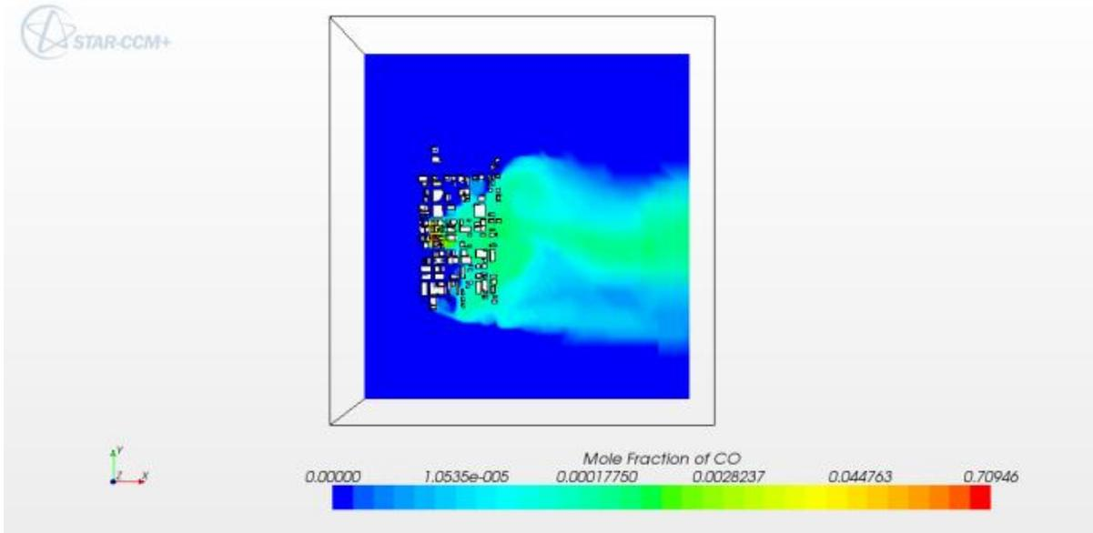
Figure 10.20: Steady state plume in 145 building model.
