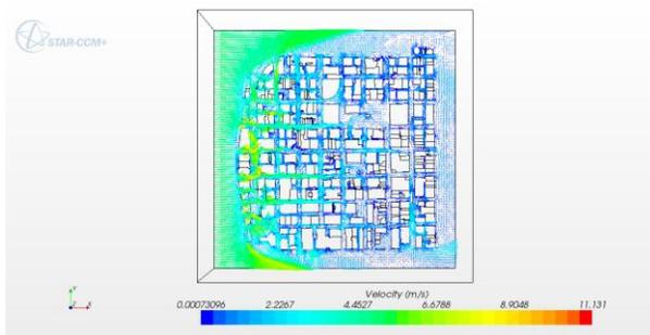
Figure 10.23: Vector field through Loop geometry.
