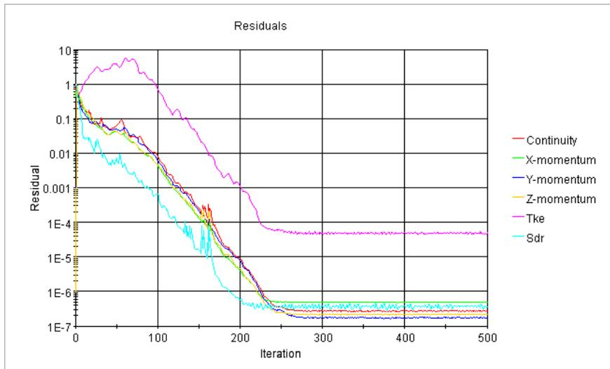
**Figure 10.4. Residual Plot Showing Convergence of the Steady Air Flow Solution**
