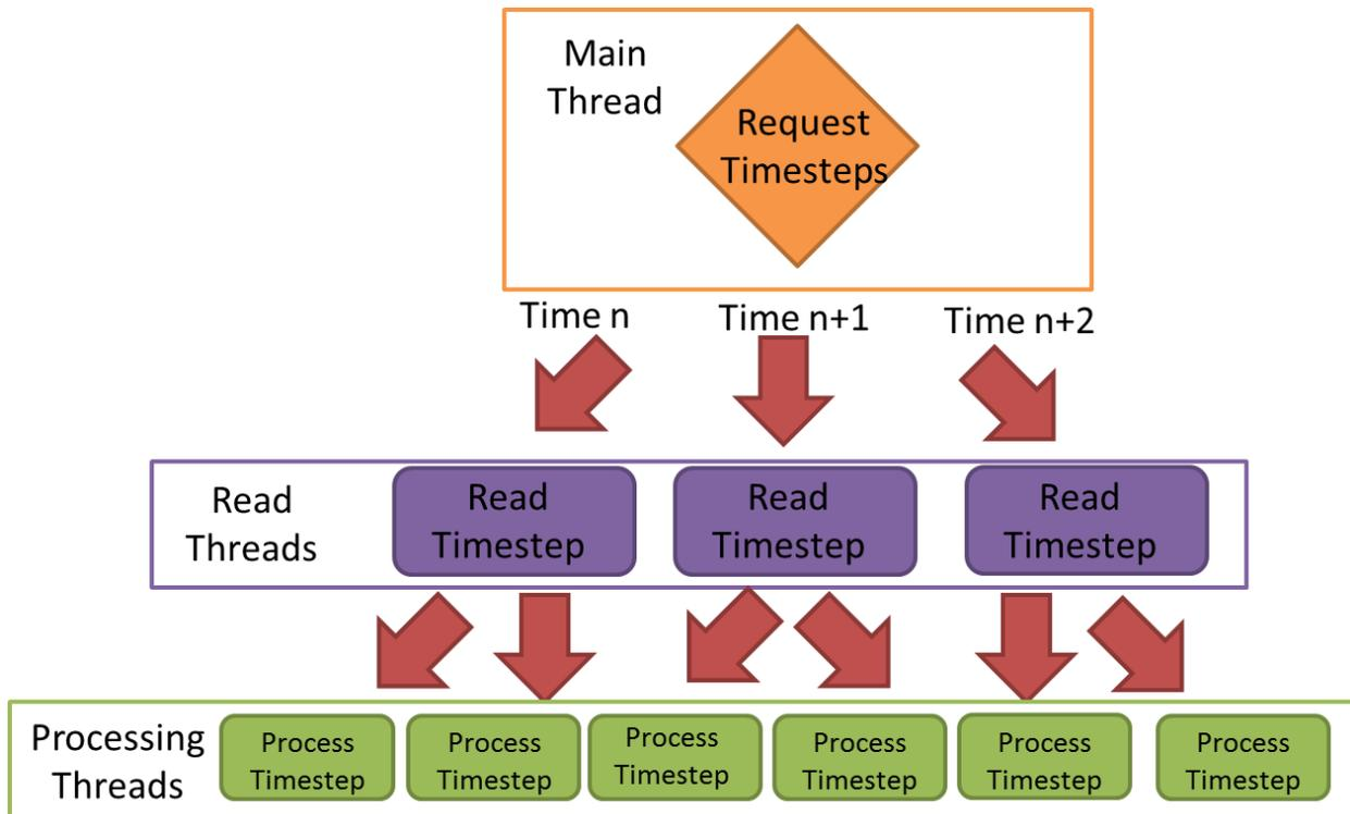
Figure 13.11: Regional Snapshot Reading Pipeline
