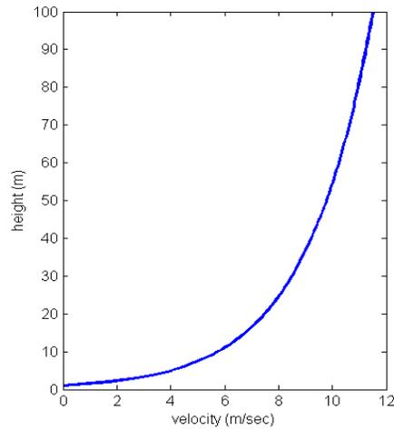
Figure 10.11. Inlet Air Velocity Profile
