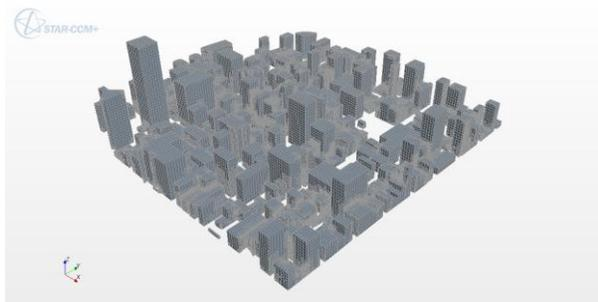
Figure 10.22: Surface mesh after surface wrapper.
