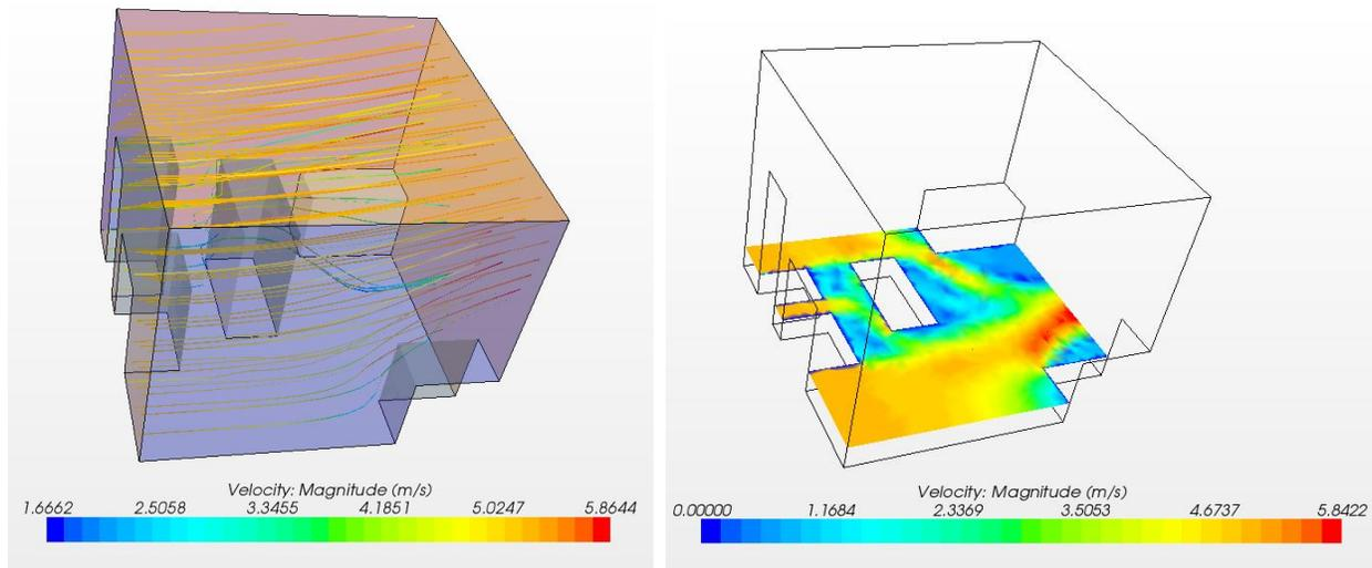
**Figure 10.3. Urban Air Flow Predicted by the Model: Boundary Condition: (East, Top = pressure outlet, North, South = symmetry outlet)**
