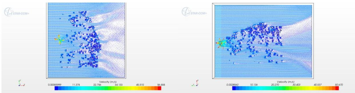
Figure 10.25: Comparison of Block plume inlet (left) and Cylinder plume inlet (right). The block inlet injects the plume at 90 degree angles. The cylinder injects the plume radially.
