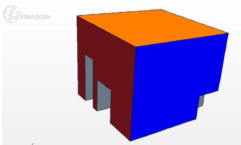
Figure 10.2. Bounding faces of the fluid continuum: west (red), south (blue), top (orange)
