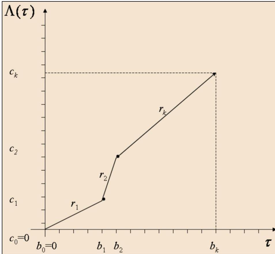
Figure 8.2: Cumulative functions for a NSPP
