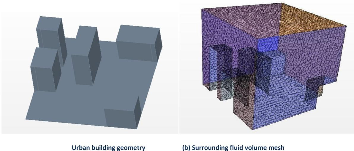
**Figure 10.1. Geometry of a Small-scale Urban Area**
