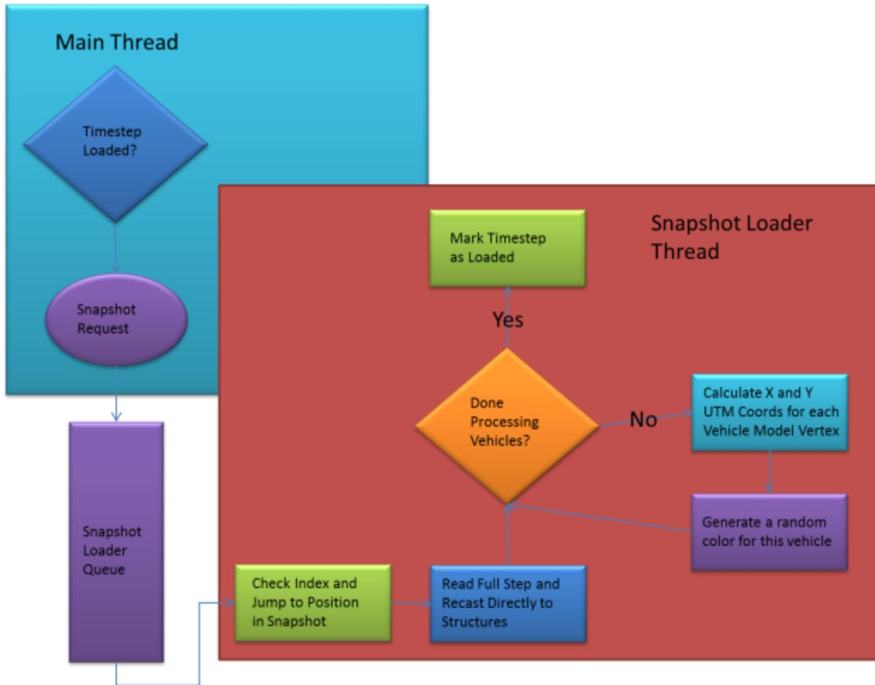
Figure 13.7: Vehicle Loading Algorithm
