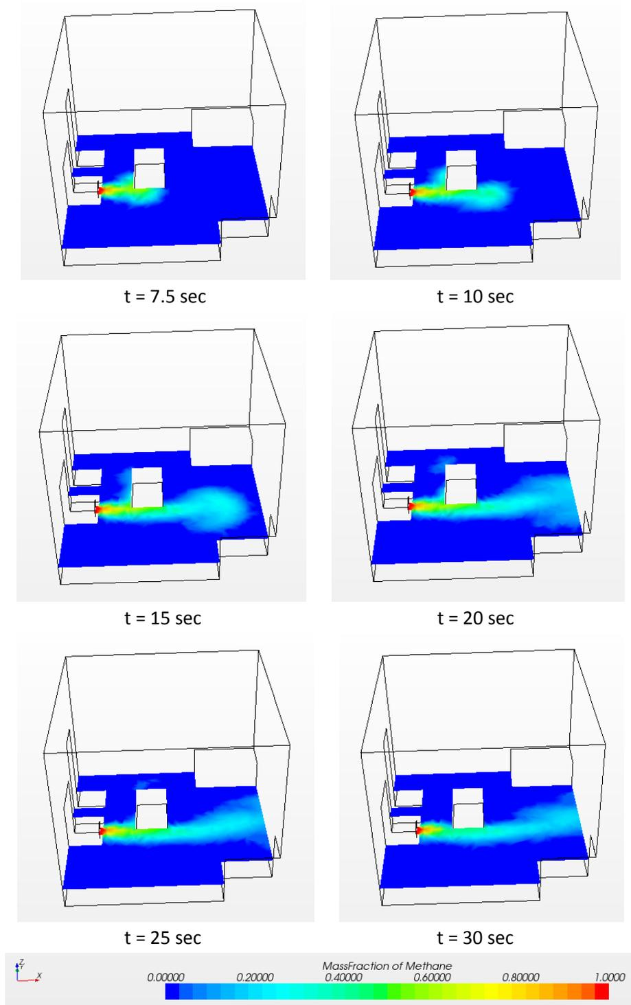
Figure 10.7. Transient Plume Dispersion (Mass Fraction of Methane) Predicted by Multi-Component Flow Model (Plume discharge starts 50 m/sec at t=5 sec, and decreases to 10 m/sec at t=30 sec)
