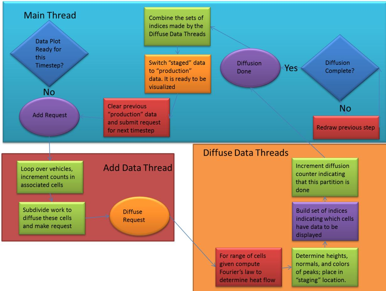
Figure 13.8: Data Plot Algorithm
