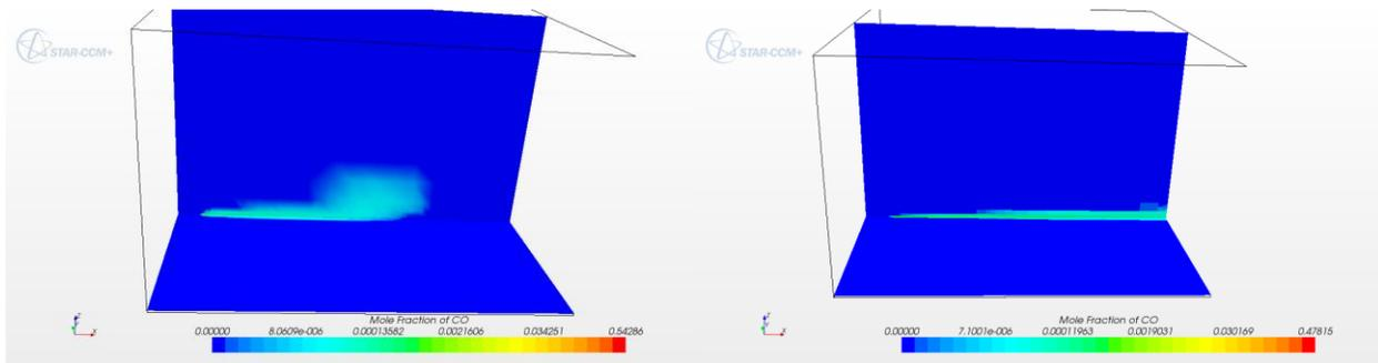
Figure 10.27: Comparison of ground level inlet with 2000 kg TNT. 5 m/s wind (left) and 20 m/s wind (right).
