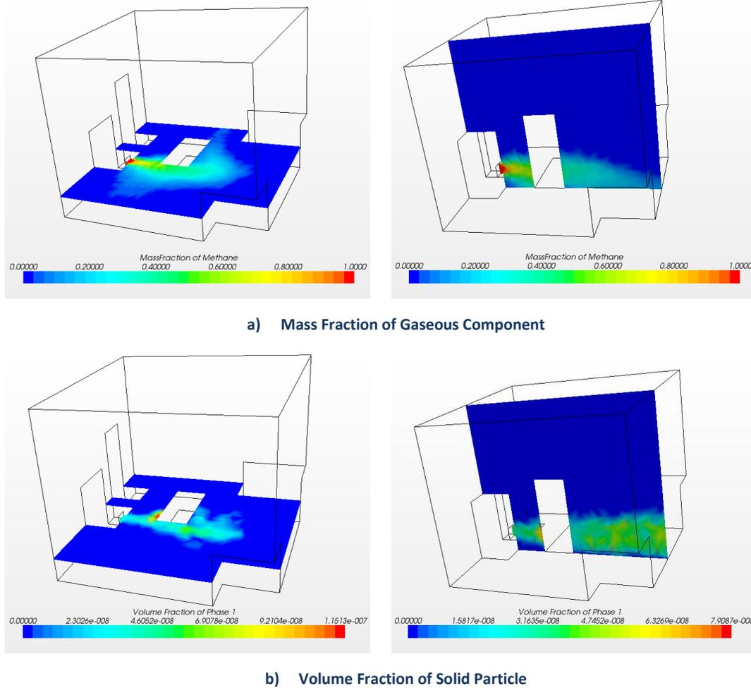
**Figure 10.10. Steady State Plume Dispersion upon Gravity Effect (particle size: 40  $\mu\text{m}$ )**
