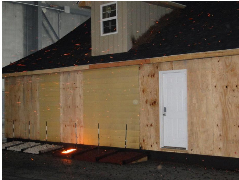
Figure 7. Ember-started ignition in the recycled rubber mulch bed.
