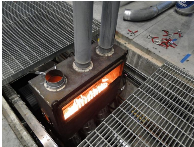
Figure 1. Flames from gas burner at the bottom of the combustion chamber (without mulch mixture).
