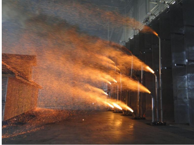
Figure 2. Ember generators discharging during test.
