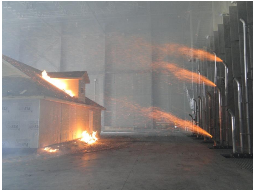
Figure 9. Burning pine needle mulch (center) and bark mulch (left). Pine needle debris next to the roof dormer also ignited.
