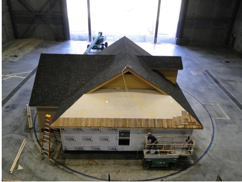
Figure 5. A view of the WUI test building showing the Dutch-hip design.
