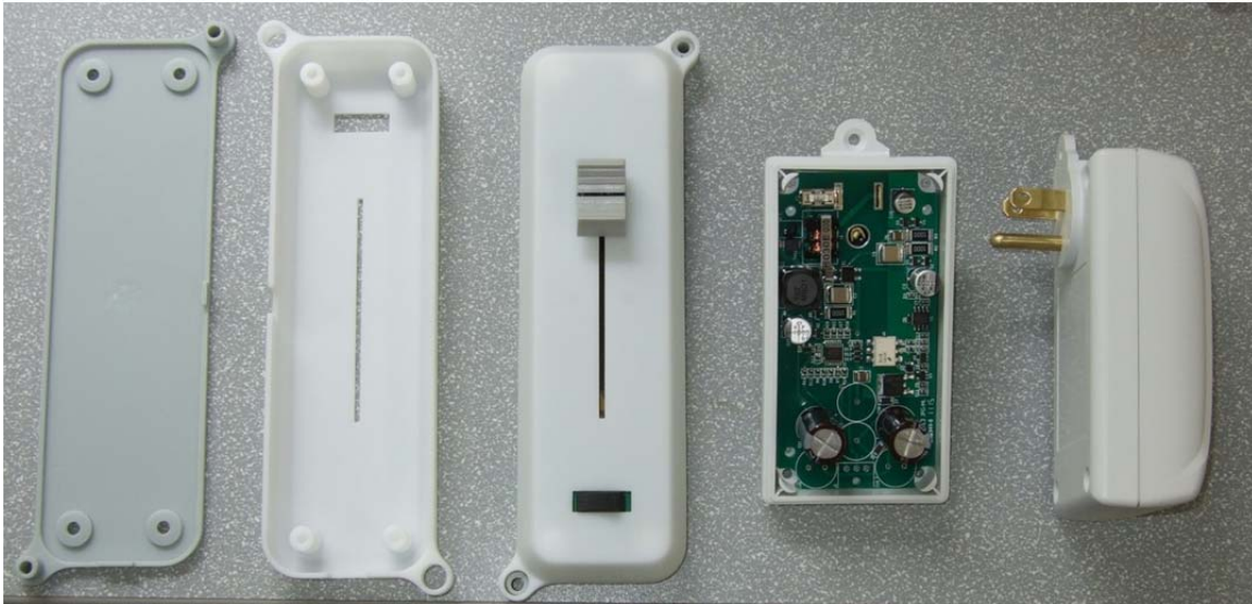
Figure 21: Picture of the control module and power supply; from left to right: Bottom piece of the control module with holes for mounting; back side of the control module top; assembled control module with the power switch and the slide for dimming; power supply printed circuit board mounted inside the AC plug assembly; assembled AC plug.
