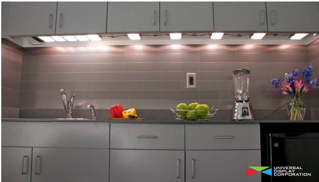
Figure 26: OLED under-cabinet lighting system. Each under-cabinet lighting system is comprised of ten 15cm x 7.5cm lighting modules mounted in outcoupling enhancement lenses and a control module.
