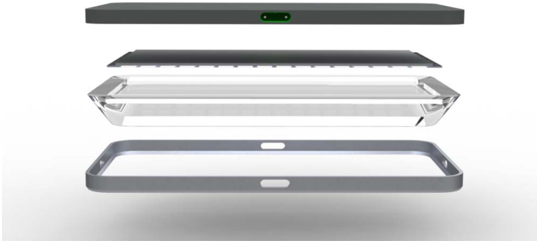
Figure 8: The components of the light module. From top to bottom: backing plate, OLED panel, outcoupling lens, aluminum frame.
