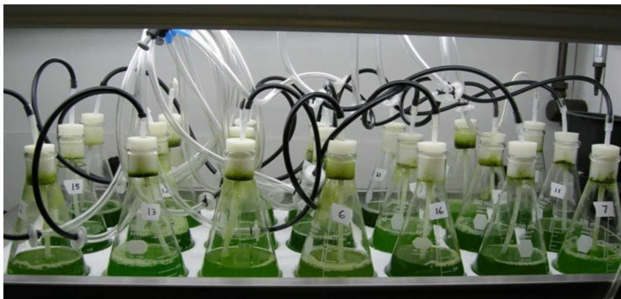
Figure 1. Algae culture system for use with simulated flue gas.
