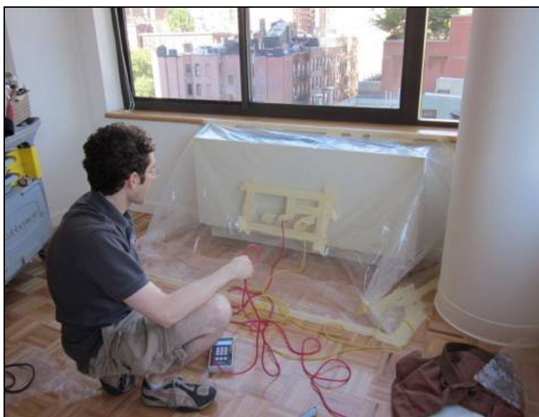
Air Infiltration Testing of a Packaged Terminal Unit
