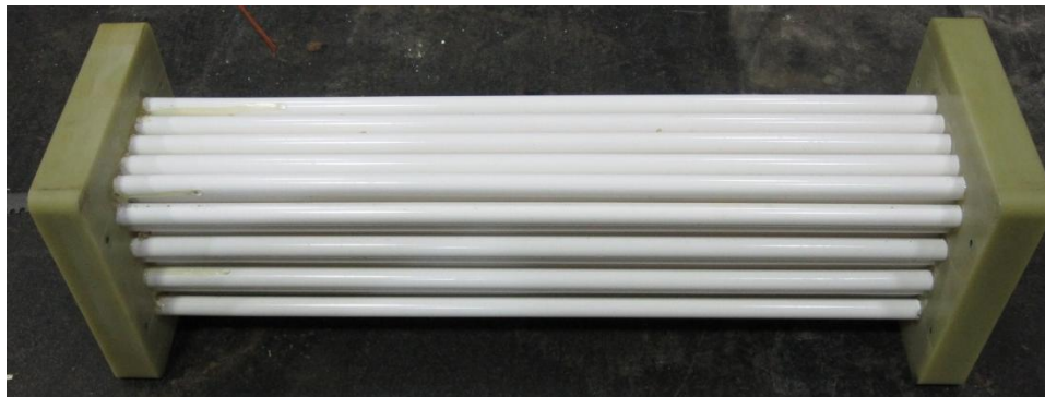
Figure 34: Photo of all ceramic module (0.5-inch-OD ceramic membrane tubes)
