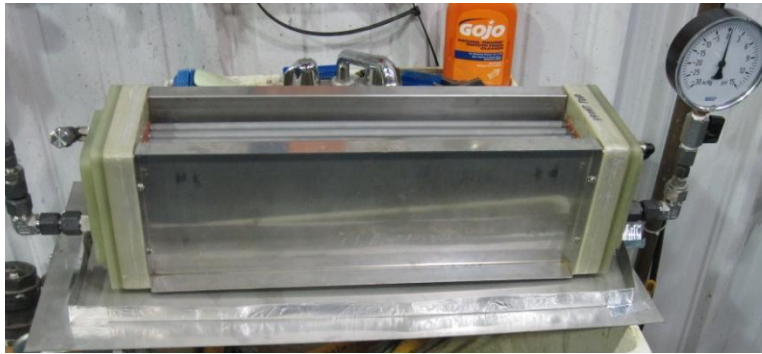
Figure 36: Metallic membrane tube module water transport testing setup
