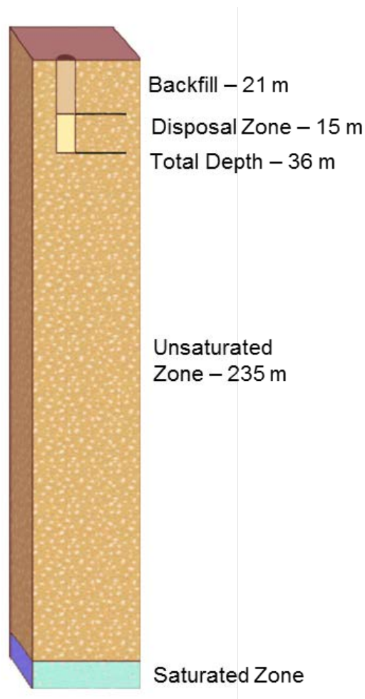
Figure 53. Schematic illustration of Greater Confinement Disposal boreholes
