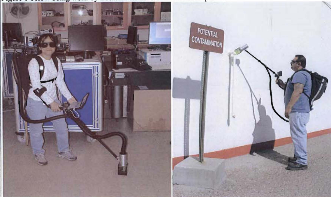
Figure1. Pictures of the LIBS backpack system.
