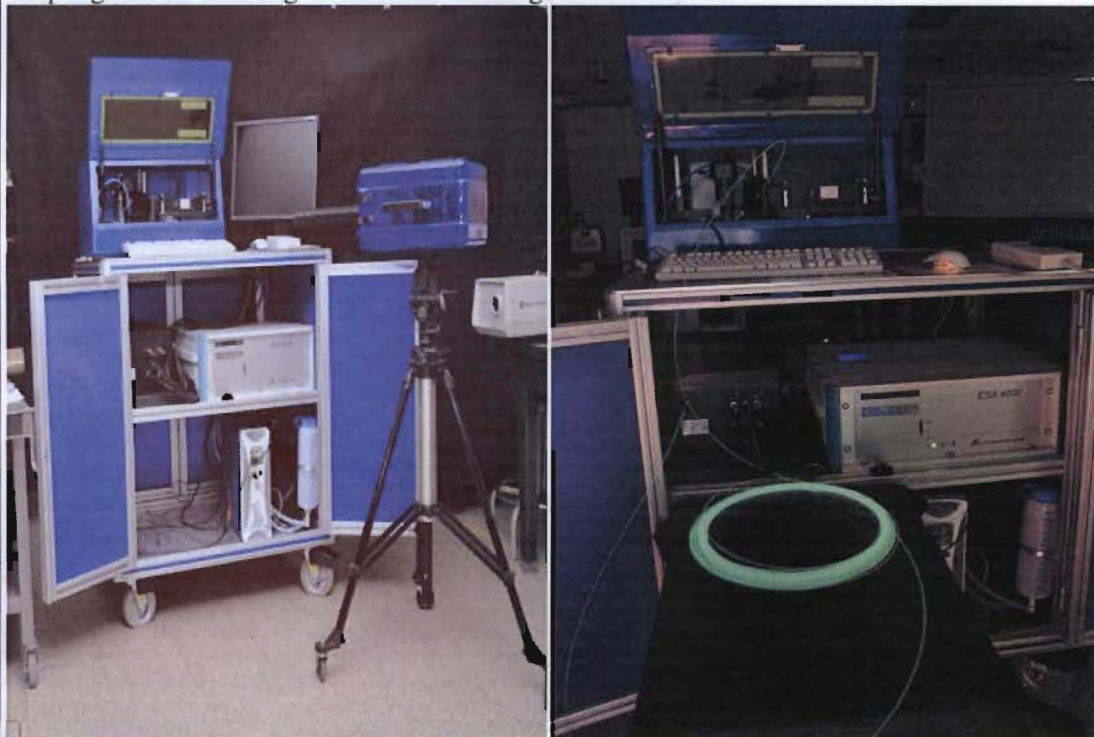
Figure2. Shown are pictures of cart / rack mounted LIBS system.
