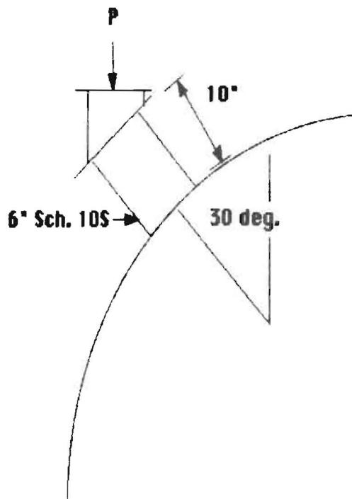
$$\text{Max. bending stress in nozzle neck} = Mc/I$$
