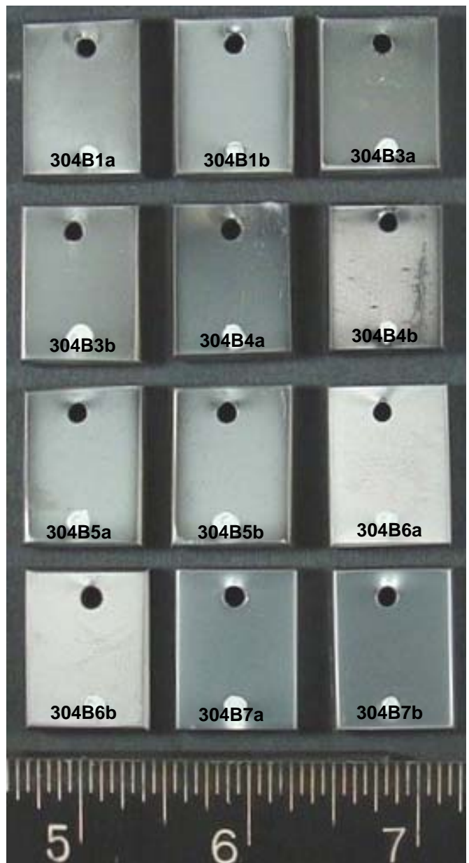
FIGURE 4-2 Representative Photograph Showing the Nanocoating and Uncoated Control Samples in the As-supplied Condition, Prior to Performing the Screening Test under Synthetic Superheater/Reheater Conditions.
