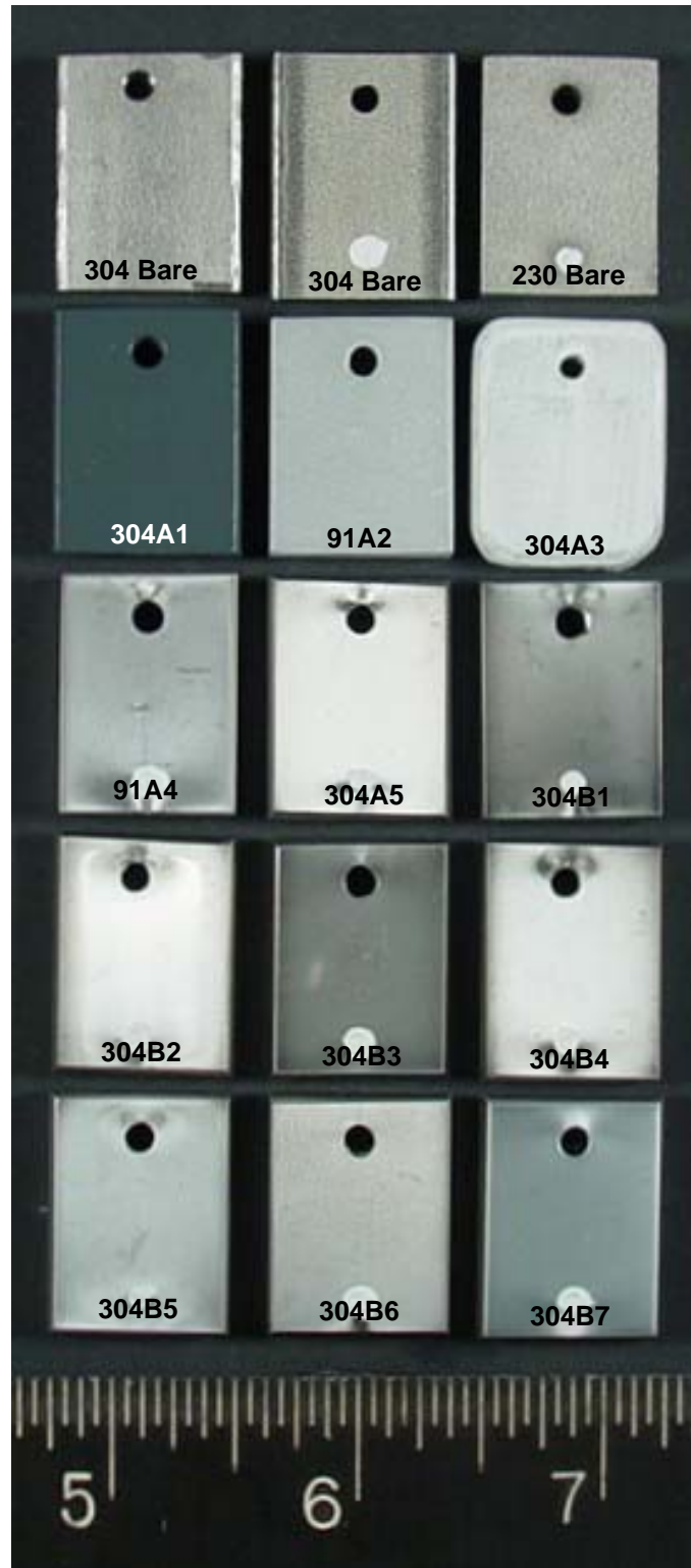
FIGURE A-15 Nanocoating Samples Prior to Testing at 815°C (1500°F) for Superheater/Reheater Conditions (Board 1). The Coupons are Labeled with the Substrate Material Followed by the Coating Designation
