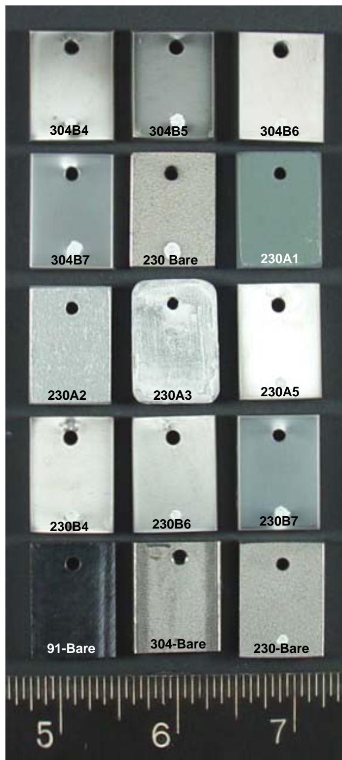
FIGURE A-9 Nanocoating Samples Prior to Testing at 595°C (1100°F) for Superheater/Reheater Conditions (Board 2). The Coupons are Labeled with the Substrate Material Followed by the Coating Designation
