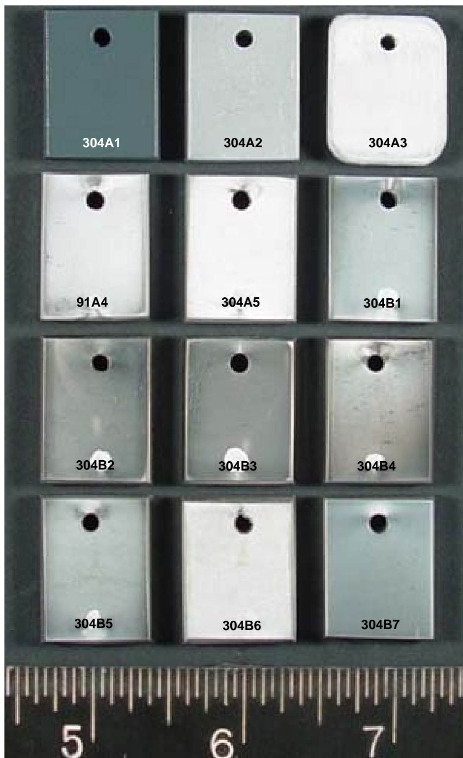
FIGURE 2-1 Representative Photograph of the Nanocoating Samples in the As-Supplied Condition on a 304 Substrate Coupon (A4 is on a 91 Substrate).
