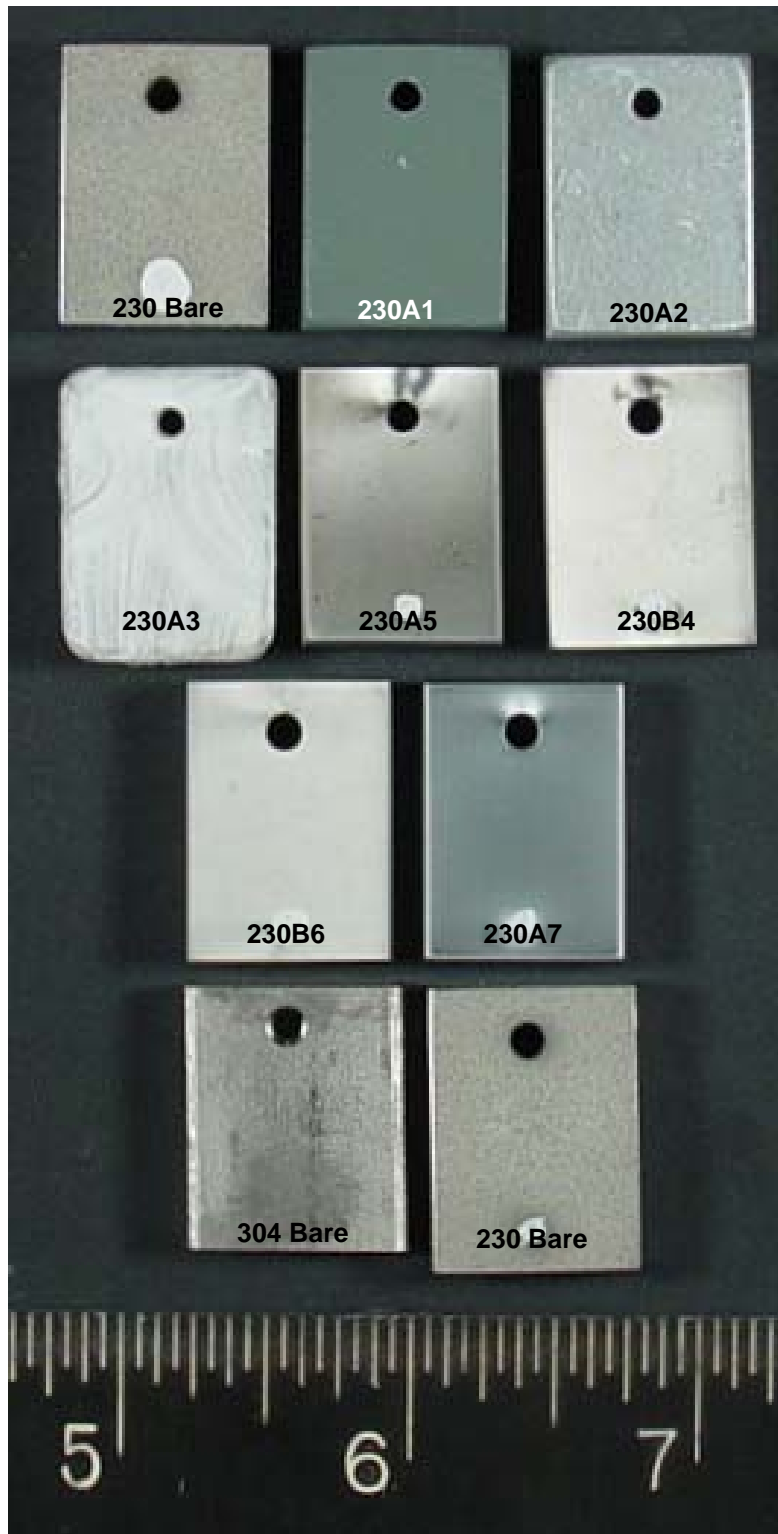
FIGURE A-13 Nanocoating Samples Prior to Testing at 705°C (1300°F) for Superheater/Reheater Conditions (Board 2). The Coupons are Labeled with the Substrate Material Followed by the Coating Designation
