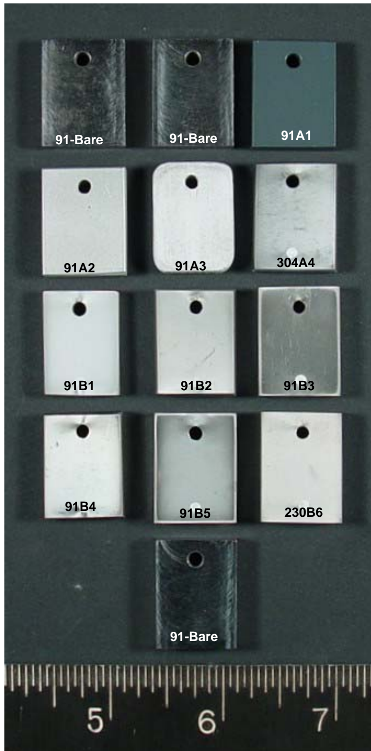
FIGURE A-1 Nanocoating Samples Prior to Testing at 455°C (850°F) for Waterwall Conditions. The Coupons are Labeled with the Substrate Material Followed by the Coating Designation.
