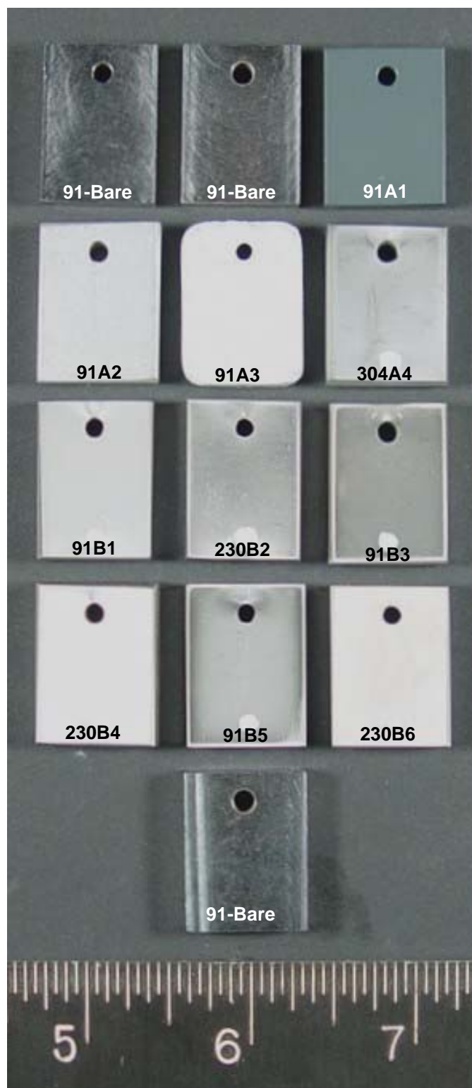
FIGURE A-5 Nanocoating Samples Prior to Testing at 595°C (1100°F) for Waterwall Conditions. The Coupons are Labeled with the Substrate Material Followed by the Coating Designation.
