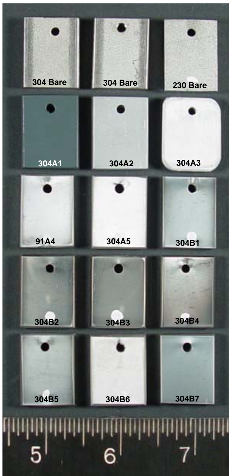
FIGURE A-11 Nanocoating Samples Prior to Testing at 705°C (1300°F) for Superheater/Reheater Conditions (Board 1). The Coupons are Labeled with the Substrate Material Followed by the Coating Designation
