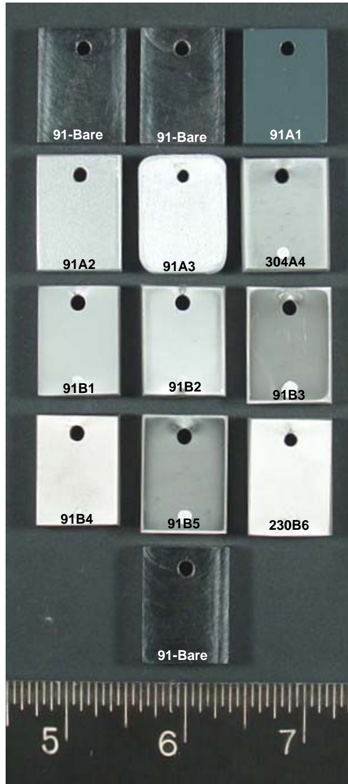
FIGURE A-3 Nanocoating Samples Prior to Testing at 525°C (975°F) for Waterwall Conditions. The Coupons are Labeled with the Substrate Material Followed by the Coating Designation.
