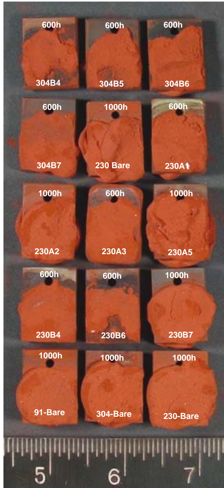
FIGURE A-10 Nanocoating Samples after Testing at 595°C (1100°F) for Superheater/Reheater Conditions (Board 2). The Exposure Times are Indicated at the Top of Each Coupon
