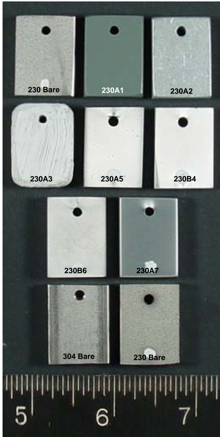
FIGURE A-17 Nanocoating Samples Prior to Testing at 815°C (1500°F) for Superheater/Reheater Conditions (Board 2). The Coupons are Labeled with the Substrate Material Followed by the Coating Designation
