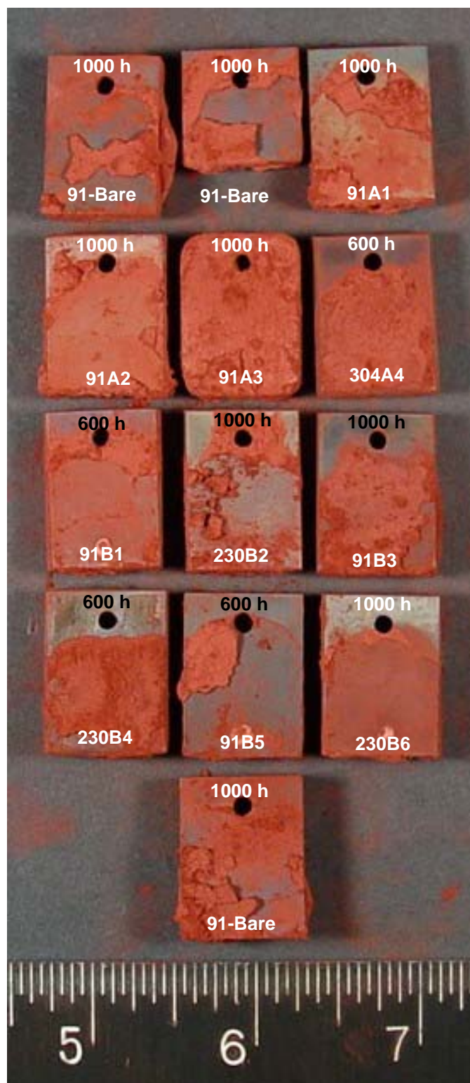
FIGURE A-6 Nanocoating Samples after Testing at 595°C (1100°F) Under Waterwall Conditions. The Exposure Times are Indicated at the Top of Each Coupon
