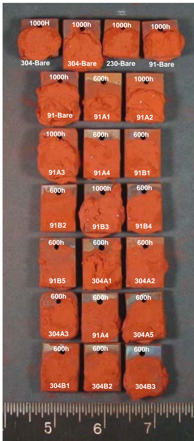
FIGURE A-8 Nanocoating Samples after Testing at 595°C (1100°F) for Superheater/Reheater Conditions (Board 1). The Exposure Times are Indicated at the Top of Each Coupon.
