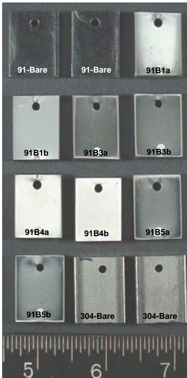
FIGURE 4-2 Representative Photograph Showing the Nanocoating and Uncoated Control Samples in the As-supplied Condition, Prior to Performing the Screening Test under Synthetic Superheater/Reheater Conditions.
