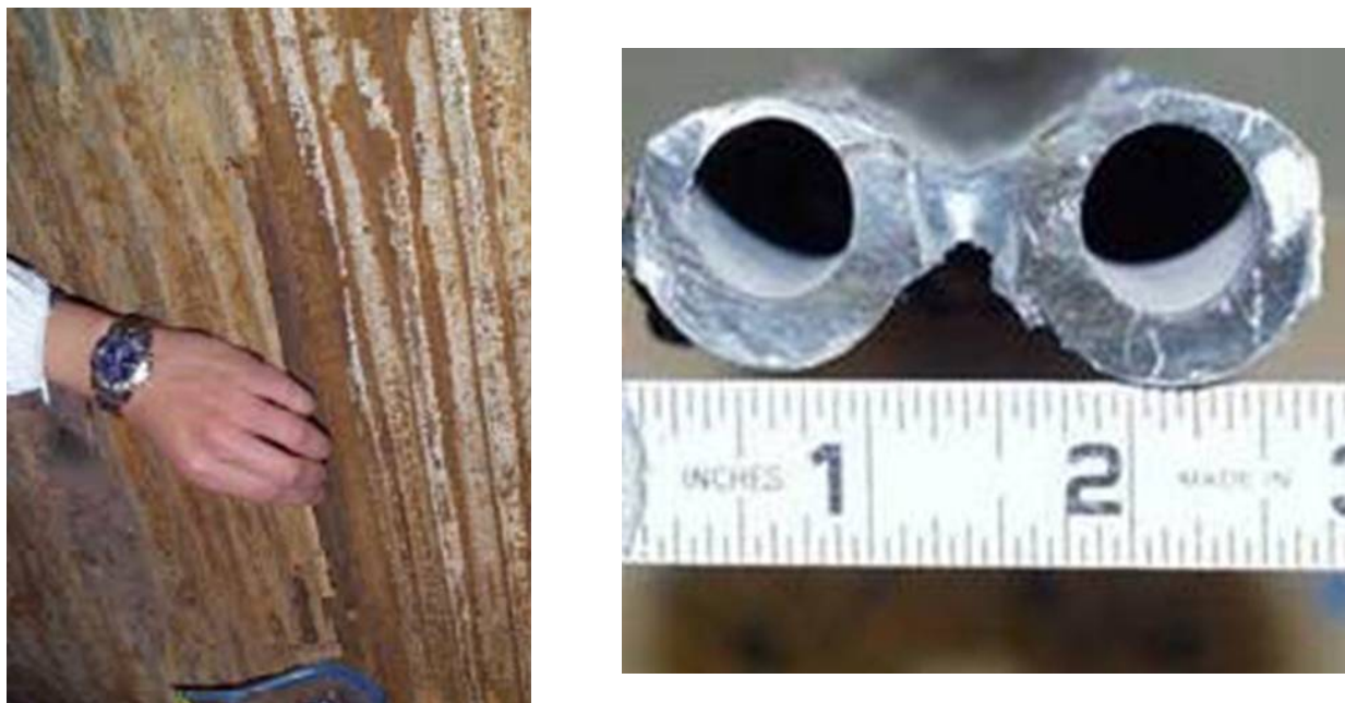
Figure 1 Photographs of waterwall and a cross section of tubes showing the extent of corrosion and wall-thickness wastage.
