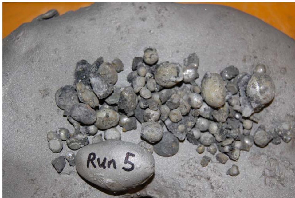
Figure 7 - Uncoalesced aluminum beads from Run 5 obtained from thorough electrolyte dissolution with water. The beads are sitting atop the solidified cathode aluminum pad
