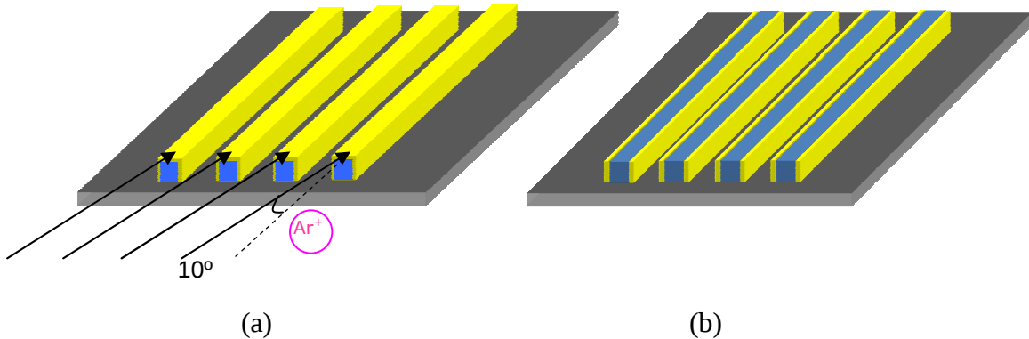
Figure 36: Schematics of structure (a) before and (c) after low angle argon ion milling
