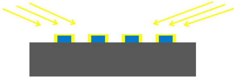
Figure 62: Schematic for the lower angle metal deposition at 14°
