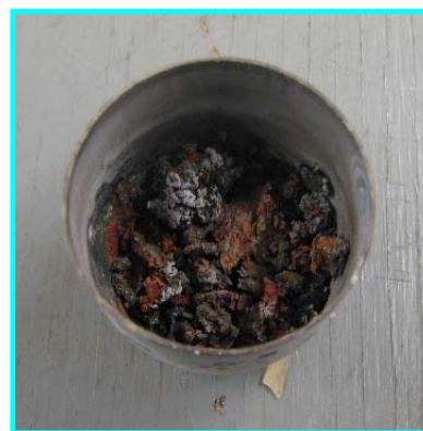
Fig. 13. Li,Zn,P material reacted in an open tantalum crucible inside the high temperature glove box under Ar atmosphere.
