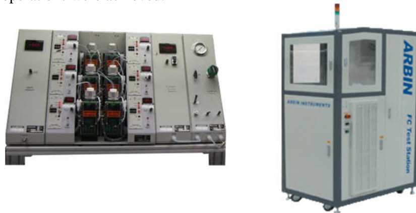
Figure 4.3.1-1: Picture of the KinTek calibration gas generator (left image) that is connected to fuel cell testing station (right image)
