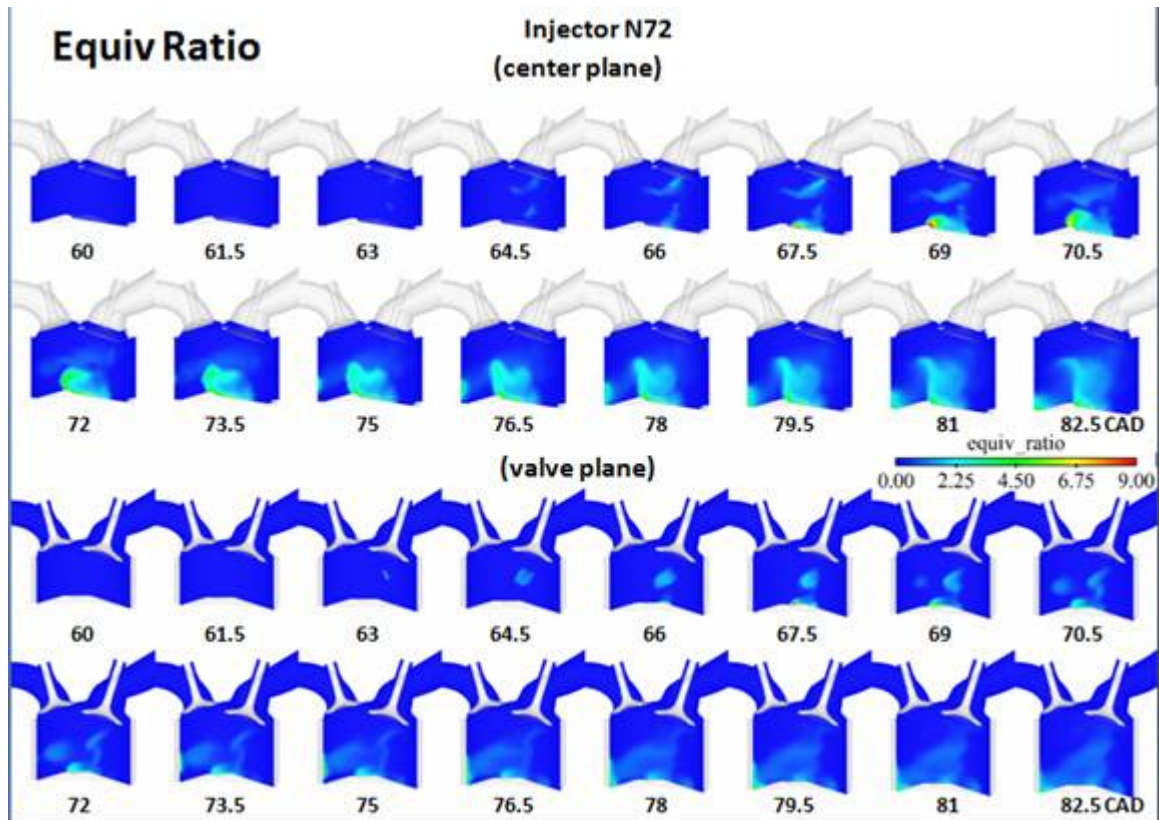
Figure 17) Fuel-Air mixing simulation for early injection case (SOI at 60° ATDC, 1000 rpm 20 mg)
