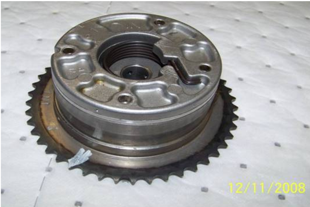
Figure 13: Delphi increased authority cam phaser for optimized E85 project
