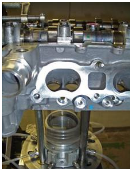
Figure 8) Optical engine setup for E85 project
