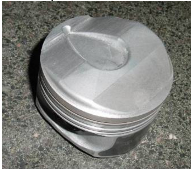
Figure 15: Piston designed for the E85 optimized project
