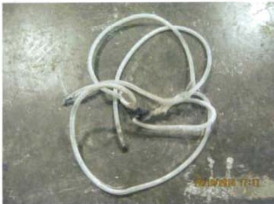
Test #5 flame damage to Tygon tubing
