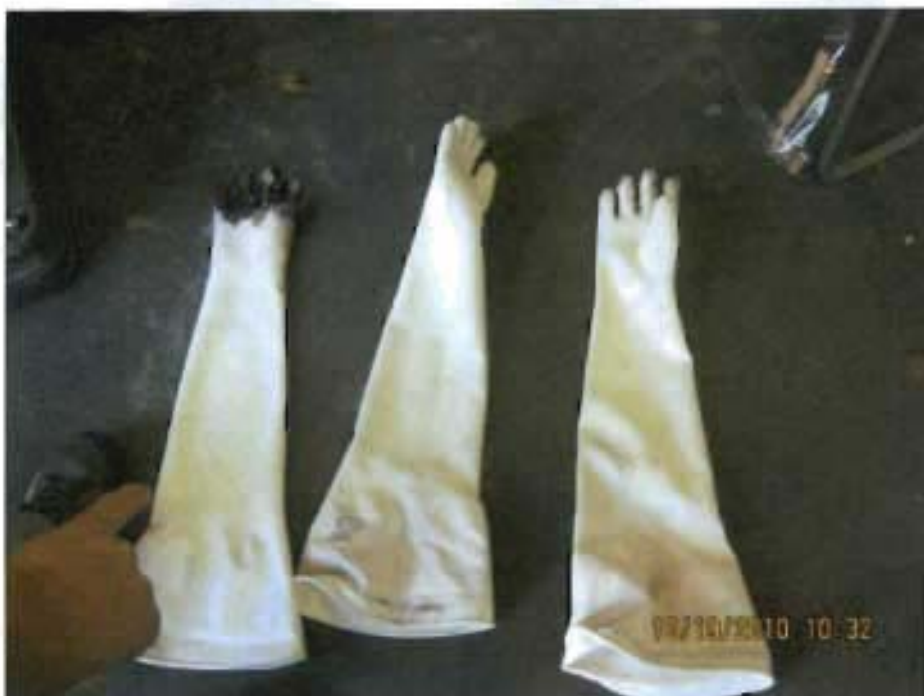
Test #1 damage to gloves impinged by flames
