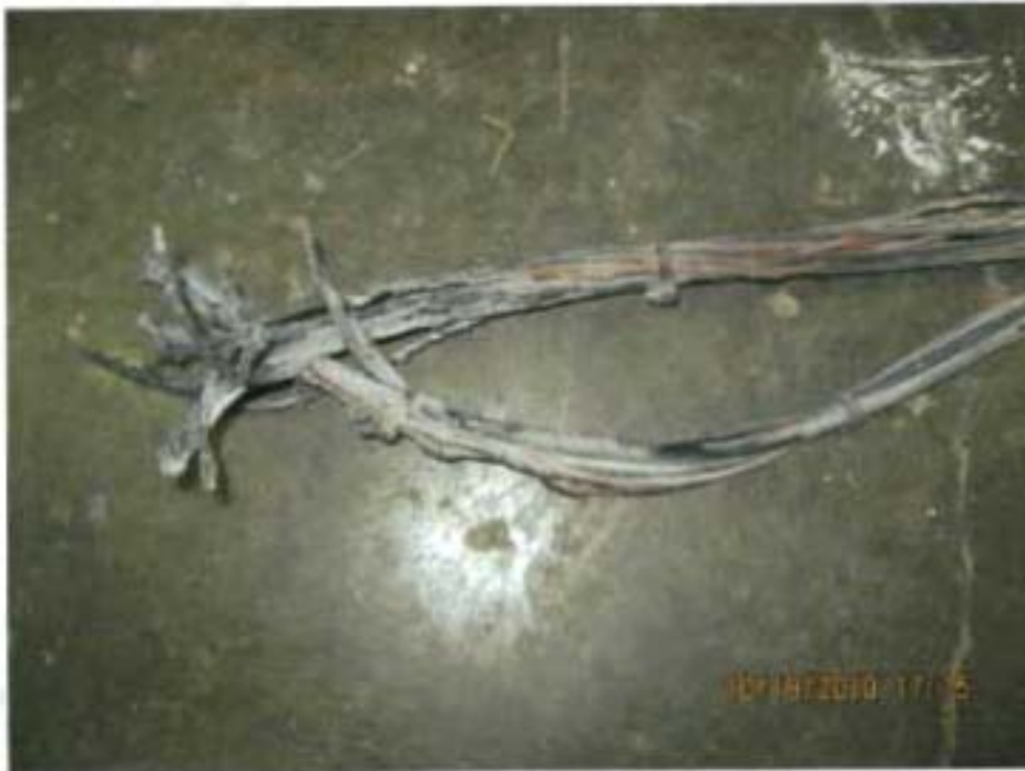
Test #5 flame damage to wire bundle
