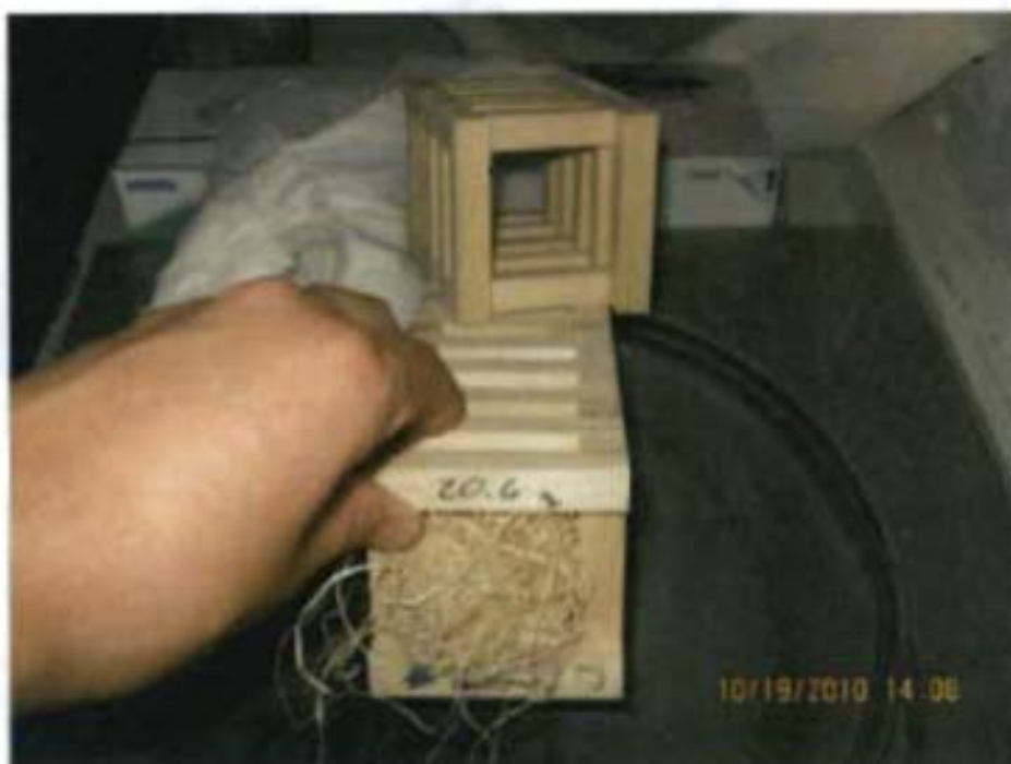
Test #3 wood crib
