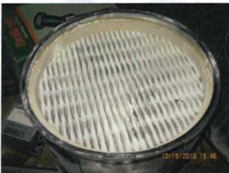
Test #4 HEPA filter post fire
