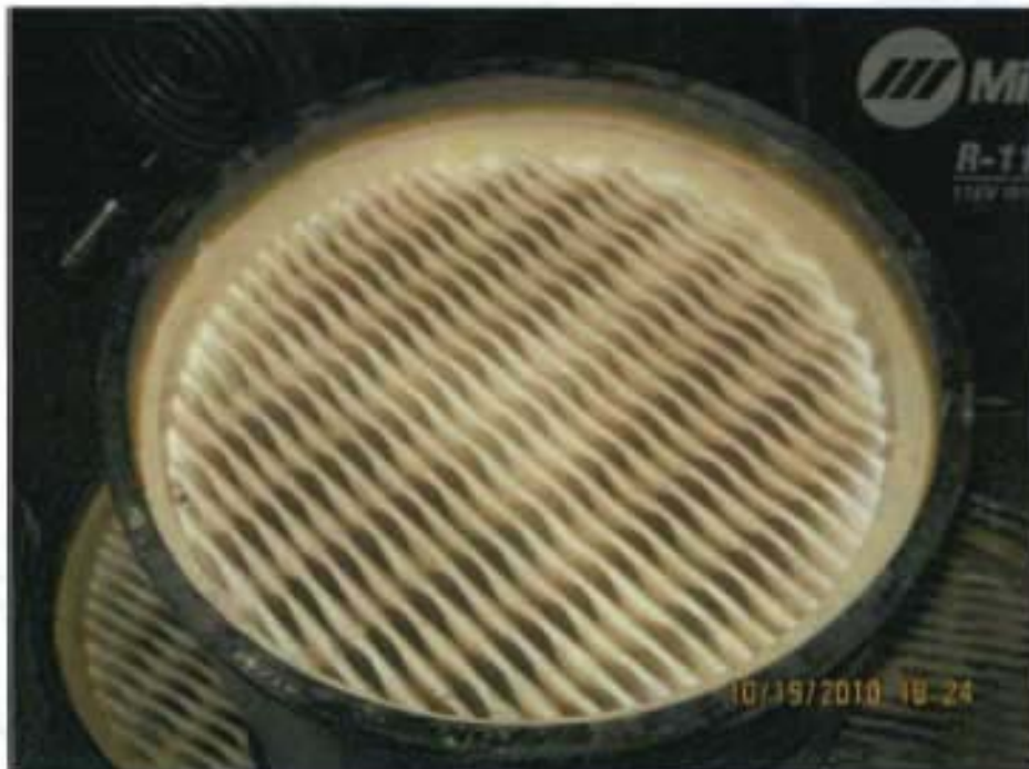
Test #6 HEPA filter post-fire
