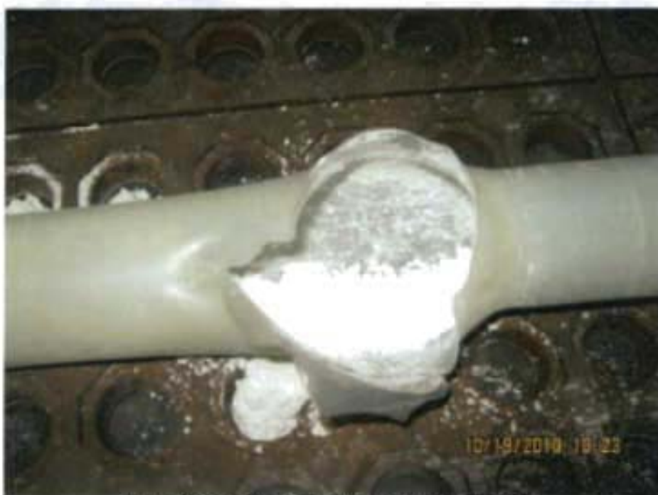
Test #6 activated Fire Foe™ tube, post-fire
