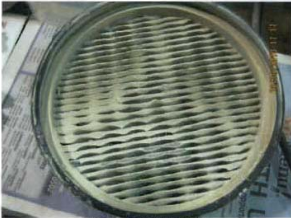
Test #5 HEPA filter post fire
