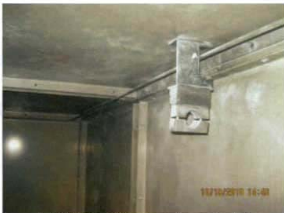
Test #3 Fire Foe™ tube damaged support brackets
