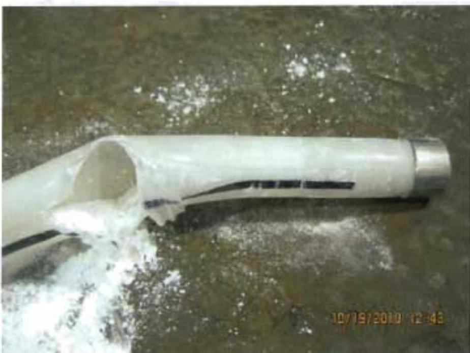
Test #1 Fire Foe™ tube discharge point
