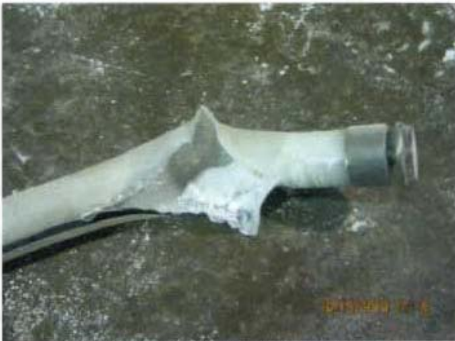
Test #5 Fire Foe™ tube activation section, post-fire
