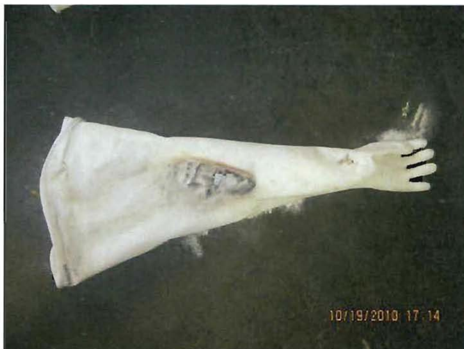
Test #5 damage to glove impinged by flame
