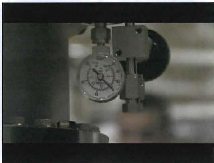
FIG. 6: VACUUM/PRESSURE GAGE AT ZERO DOCUMENTING OPEN VALVE.
