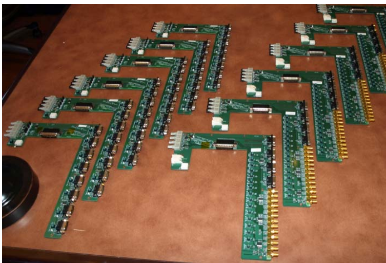
Figure 21. Each cart requires one “Box 3 Elbow Arc Detector Interface”, which comprises two custom boards and two DSQUIRT fiber optic transceivers. The boards are physically constructed to “wrap around” the DSQUIRTS to fit a stacked assembly in a compact box
