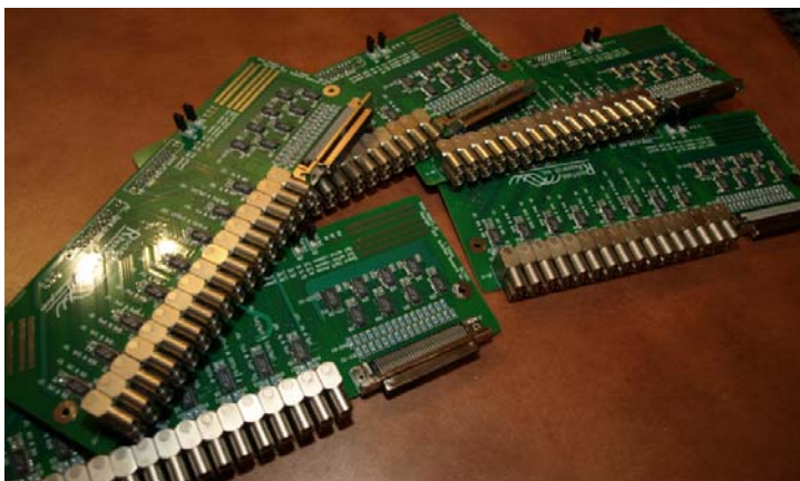
Figure 5. Five of the analog repeater boards (the third, or top board of the front assembly) are shown above. Analog signals, scaled and buffered are brought onto this board via board-board connectors, repeated via on-board buffers separately to single-pin LEMO test points and to a SCSI68 connector to mate with fast digitizer.
