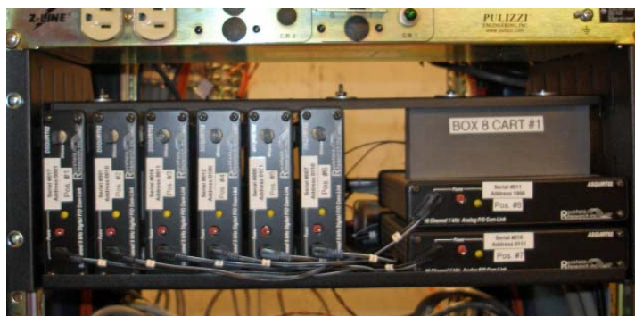
Figure 25. The Box 8 interface is primarily a rack mount housing for six DSQUIRT and two ASQUIRT modules.....
