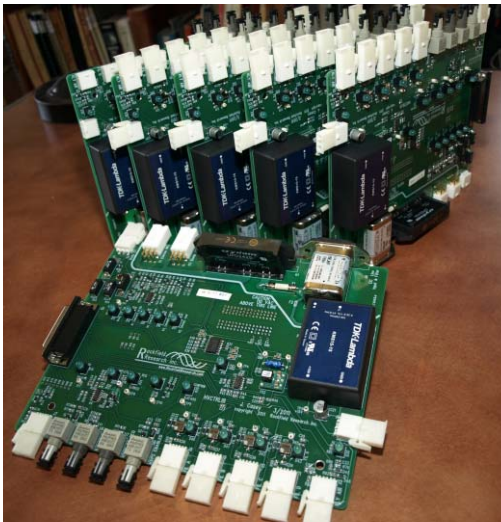
Figure 18. Six “box 1 HV control” units assembled and tested at Rockfield Research facility. Each of these boards interfaces to a DSQUIRT digital multiplexed fiber-optic I/O transceiver, and controls hardware in the HV area of the four-klystron cart.
