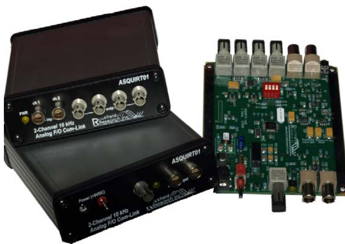
Figure 26. The “ASQUIRT01” 2 channel 10 kHz analog F/O communications link, a sub-unit of the Alcator C-Mod TPS.
