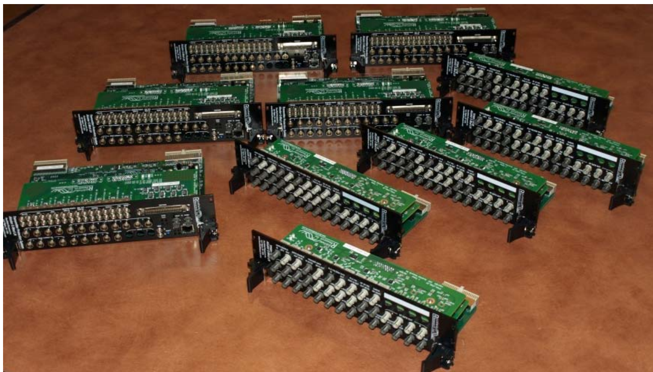
Figure 1. The suite of five complete TPS core units (front assemblies and rear transition module assemblies) on the test bench after final testing, ready to ship to MIT.
