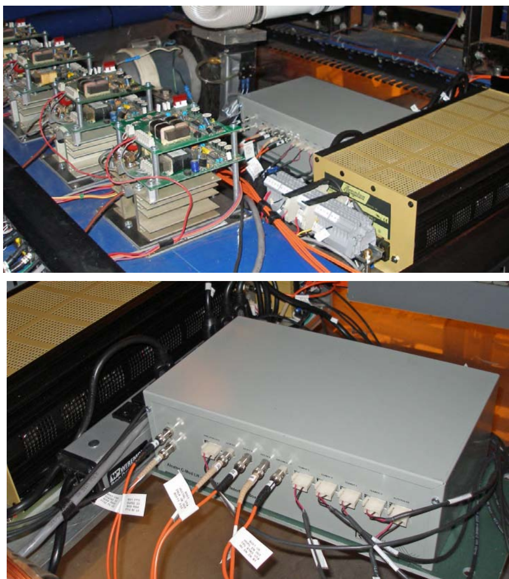
Figure 19. One of the “box 1 HV control” units is shown installed in the HV area of the cart, adjacent to the legacy filament power supplies, and underneath the klystron sockets.
