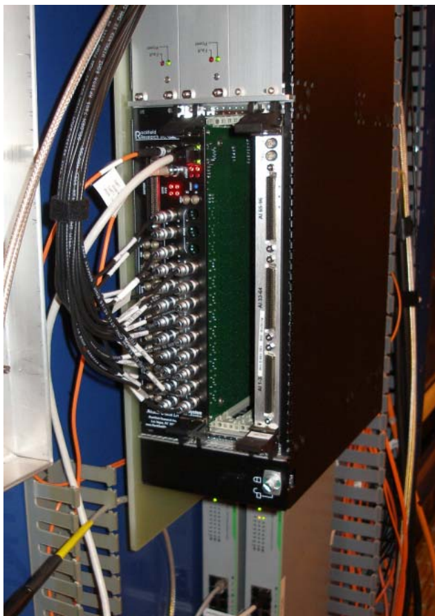
Figure 17. One of the TPS assemblies, installed in cPCI crate and installed on the side of klystron cart on the Alcator C-Mod LH facility.
