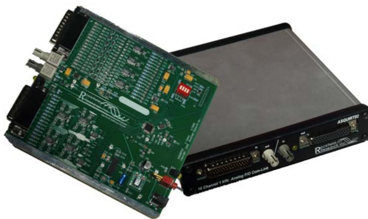
Figure 27. The “ASQUIRT02” 16 channel 1 kHz analog F/O communications link, a sub-unit of the Alcator C-Mod TPS.
