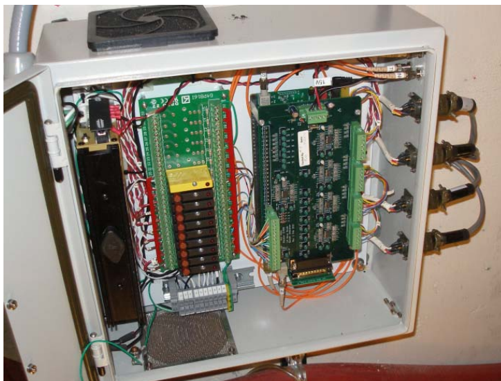
Figure 20. Each cart has a “box 2 – Waveguide Switch Box”, shown here installed in the C-Mod Cell. Opto-22 interface modules on the left, and a custom interface board at right interface to a DSQUIRT I/O board, mounted underneath at right.
