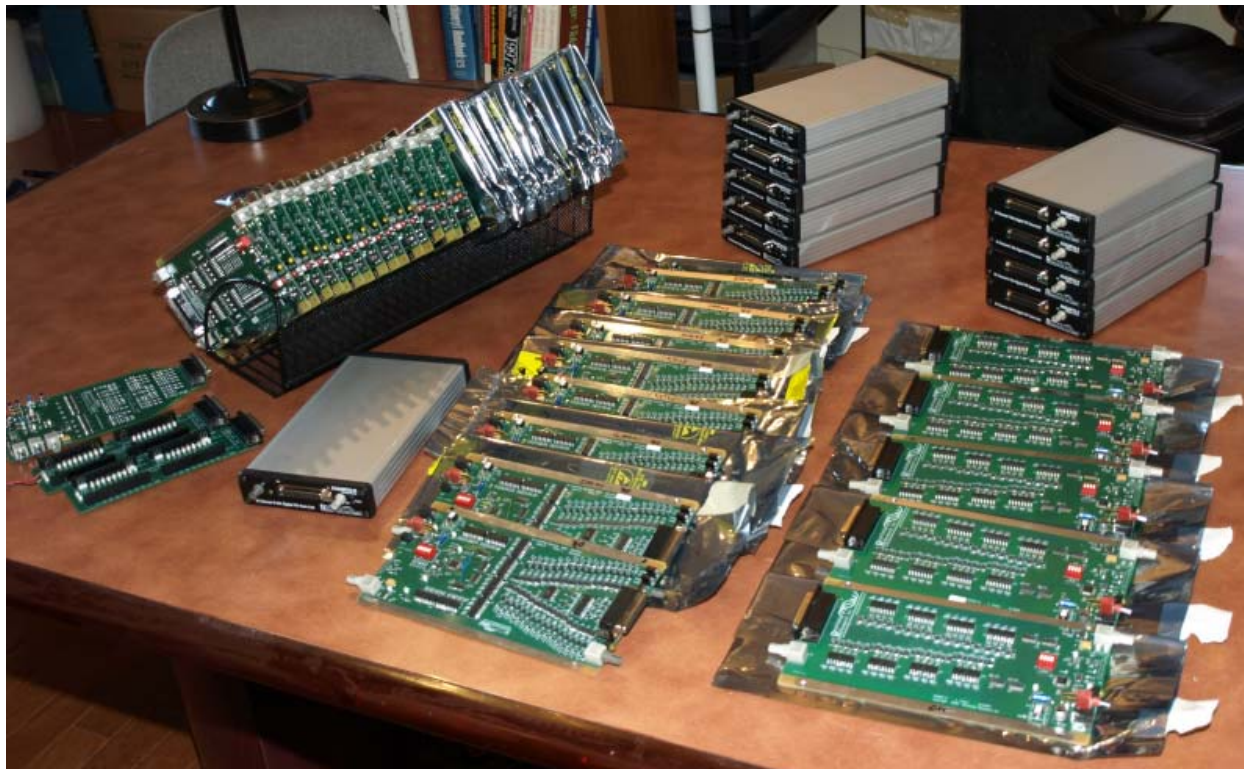
Figure 29. The entire suite of DSQUIRT02 boards – II, OO, and IO varieties – are shown after testing. Some are installed in the extruded aluminum chassis for standalone installation, some remain bare boards for embedding within other assemblies.
