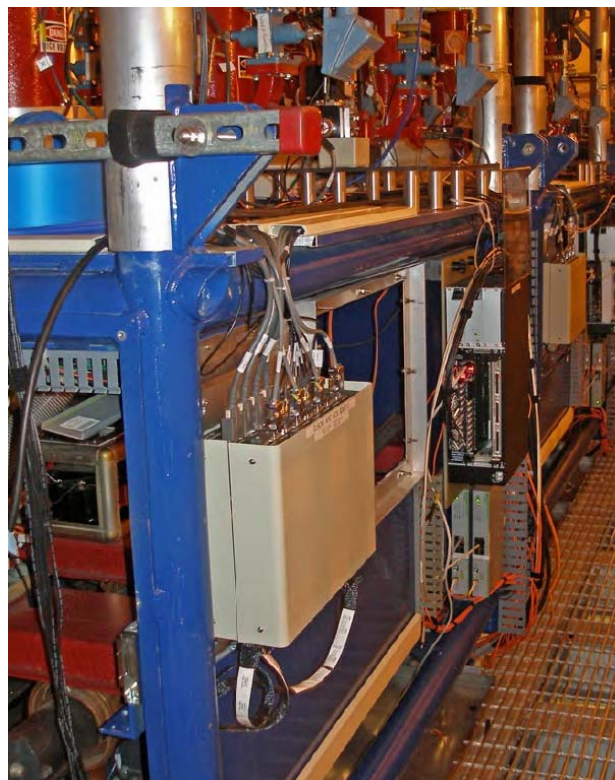
Figure 22. One of the Elbow Arc interface boards is shown on the testbench, plugged into its embedded DSQUIRT interface (above). One of the Elbow Arc units is shown mounted on the side of a cart, installed at MIT (right).
