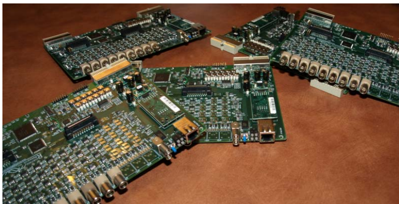
Figure 3. Five of the main boards are shown above. Each of these boards services 12 analog channels (eight body currents, 1 ground current, and 3spares). In addition, there is a repeater port for MDSplus start and clock signals, an Ethernet port, and reset button and LED status display. Both the master CPU and Event Logger CPU, in addition to the programmable fault logic matrix are resident here.
