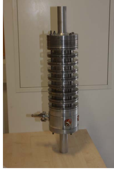
Figure 1. Aluminum prototype 9 cell crab cavity with HOM and power couplers.
