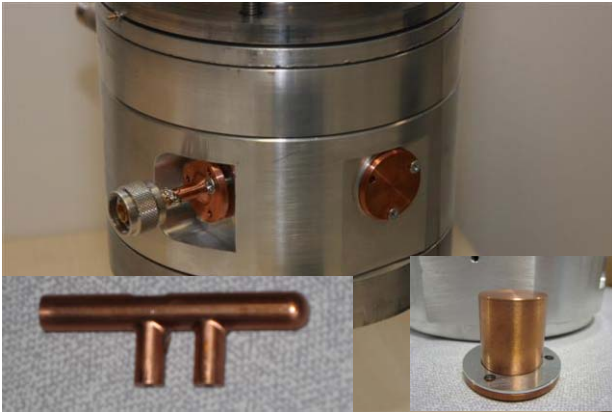
Figure 3. The prototype HOM coupler, with F-probe (inset left) and adjustable can lid (inset right).
