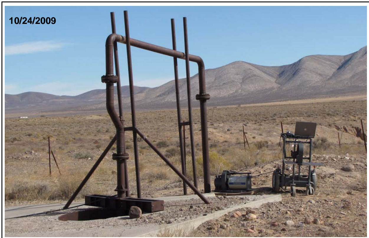
Figure 2-1 ISOCS Survey of Pipe Assembly at U2ag Mullet
