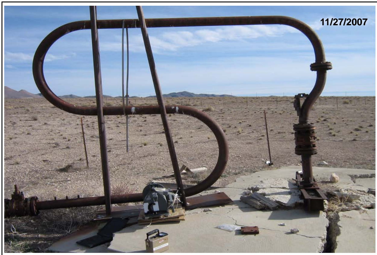
Figure 2-2 ISOCS Survey of Expansion Joint at U9cc Player
