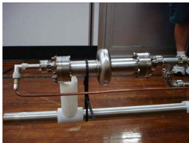
Figure 9. A single cell crab cavity read for insertion into the vertical cryostat
