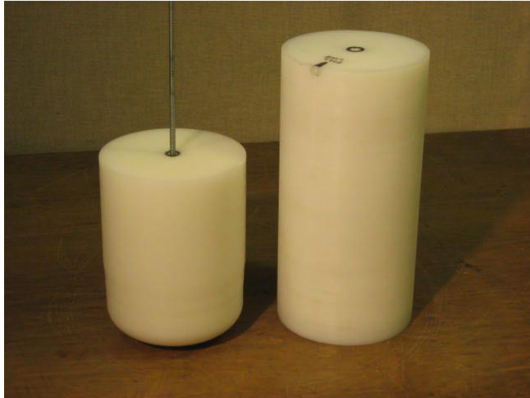
Figure 41. Resonator fillers. The lower filler on the left is machined with the inner contour of the pressure vessel head. The upper filler on the right rests upon the lower filler. It has a very close fit to the inner resonator wall (to a few thousandths of an inch).
