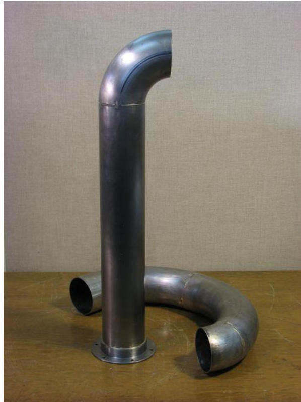
Figure 46. Steel components cut and brazed together of the trombone (upright) and tuba (laying flat) acoustic ducts.
