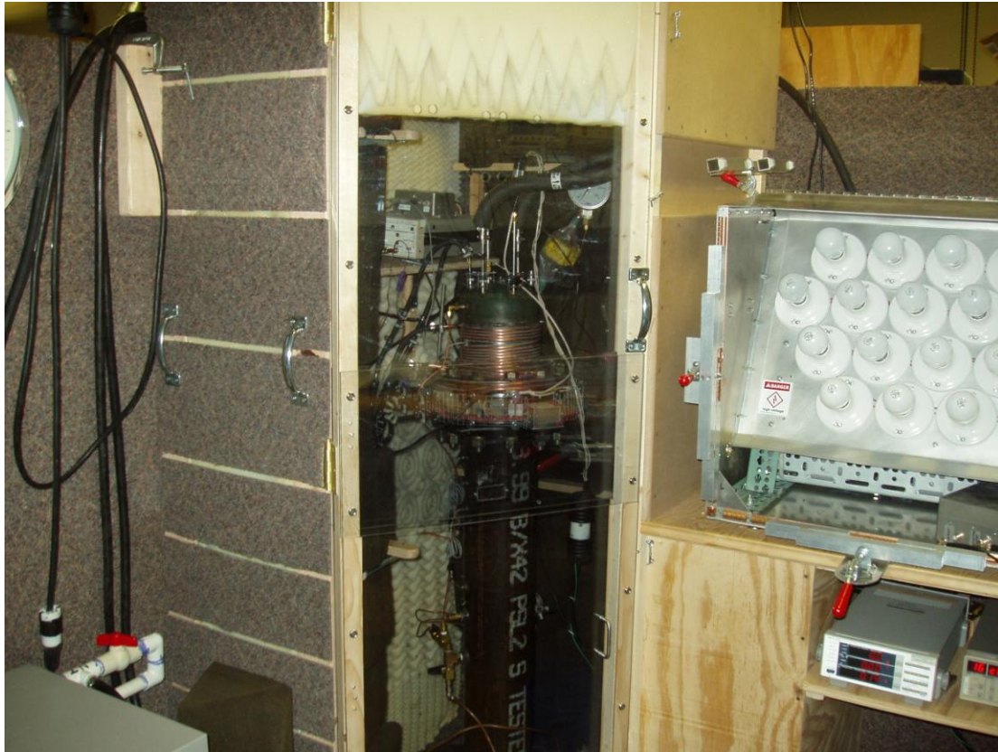
Figure 3. Demonstrator in its closed booth. The back end of the water chiller used to pull heat out of the ambient heat exchanger can be seen in the lower left. A second water chiller is behind the left wall and used to pull heat out of the oscillator plates, the copper tubes wrapped around the pressure vessel, and an internal heat exchanger known as the secondary heat exchanger.
