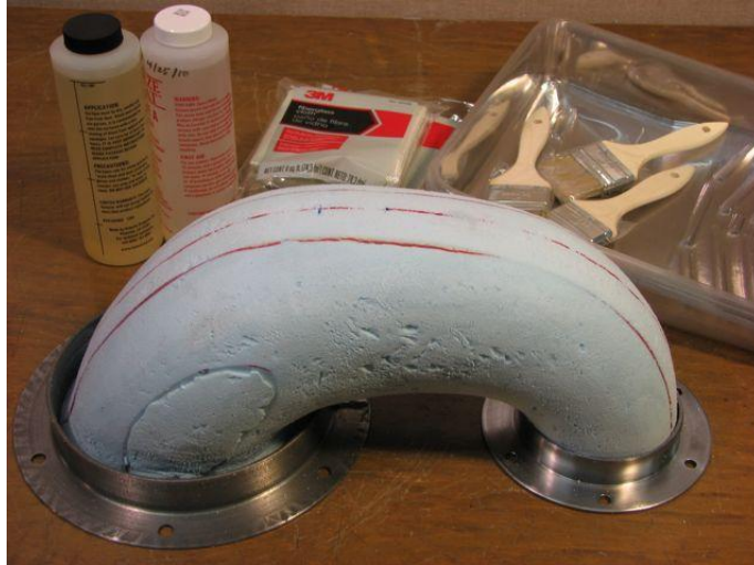
Figure 48. Trombone entry horn foam core before the application of modeling clay.
