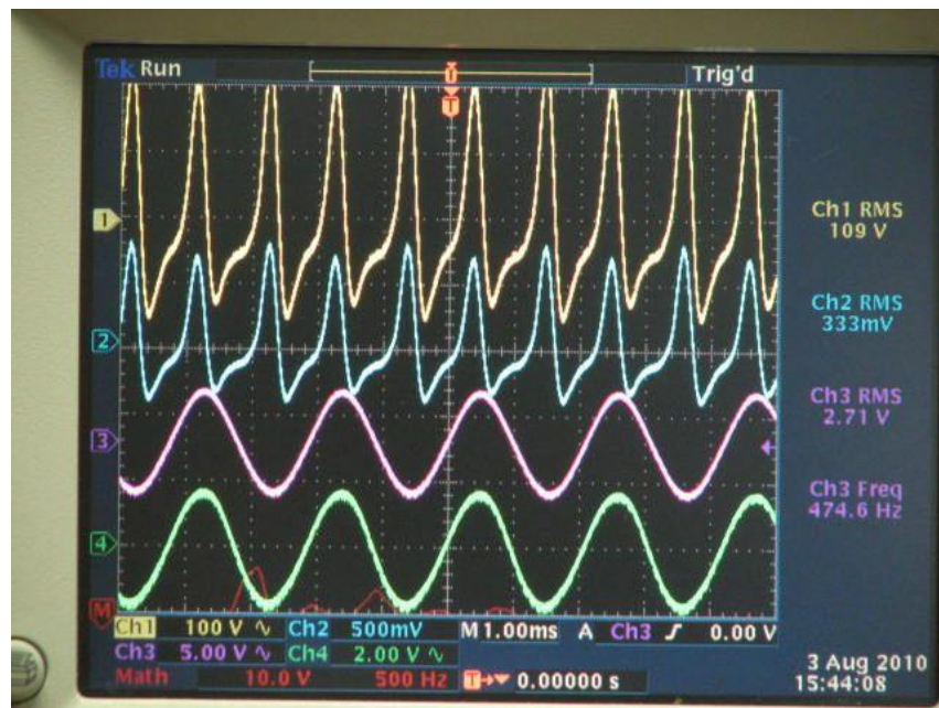
Figure 40. Waveforms at slightly lower power than shown in Figure 39. From top to bottom, the output voltage, output current (1 amp per volt), acoustic pressure in the engine above the alternator, acoustic pressure well below the alternator.
