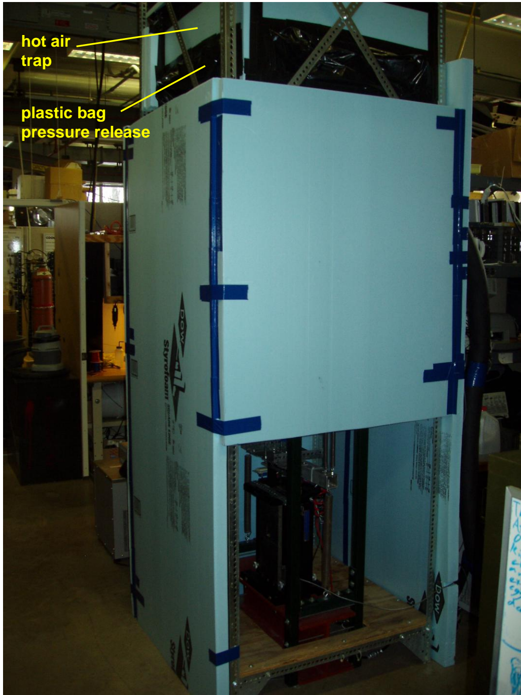
Figure 3. Improved insulation. The heat exchanger tubes and the ducts are encased in a solid block of foam insulation sheets. Layout of the hot and cold plumbing is cleaned up and insulated. Hot and cold fluid plumbing lines are better segregated. Air in the hot duct is no longer driven by an upper piston, but is instead at atmospheric pressure. The structure at the top of the apparatus is an inverted U-shaped hot air trap and pressure release boundary condition for the hot duct. Black plastic bags flex as the oscillating flow is driven, allowing the hot duct pressure to be at atmospheric without mixing in cold air from the laboratory.
