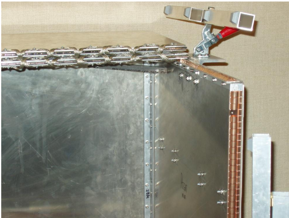
Figure 3. Close up of RF shielding gaskets, lid hinges, and lid clamp.
