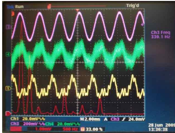
Figure 5. Strong harmonics of f , 2f and 6f in the stack voltage signal, fourth run, at 1.5 kPa acoustic pressure, 689 kPa mean pressure.
