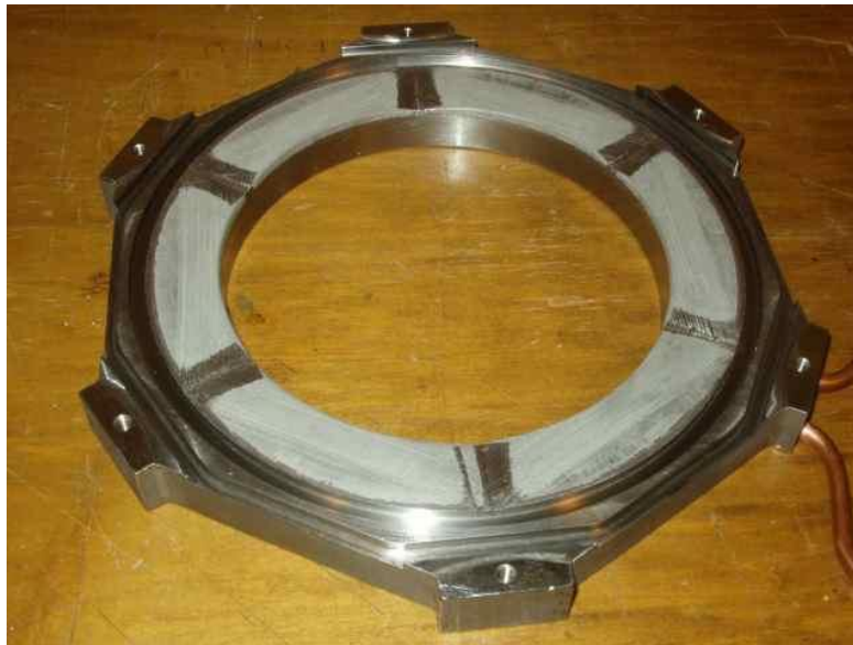
Figure 13. Osculator plate with the surface facing the diaphragm machined into six cylindrical segments. A thin (.002") layer of clear tape is on the machined surface to protect the diaphragm from contacting the bare metal of the plate at high oscillation amplitude.
