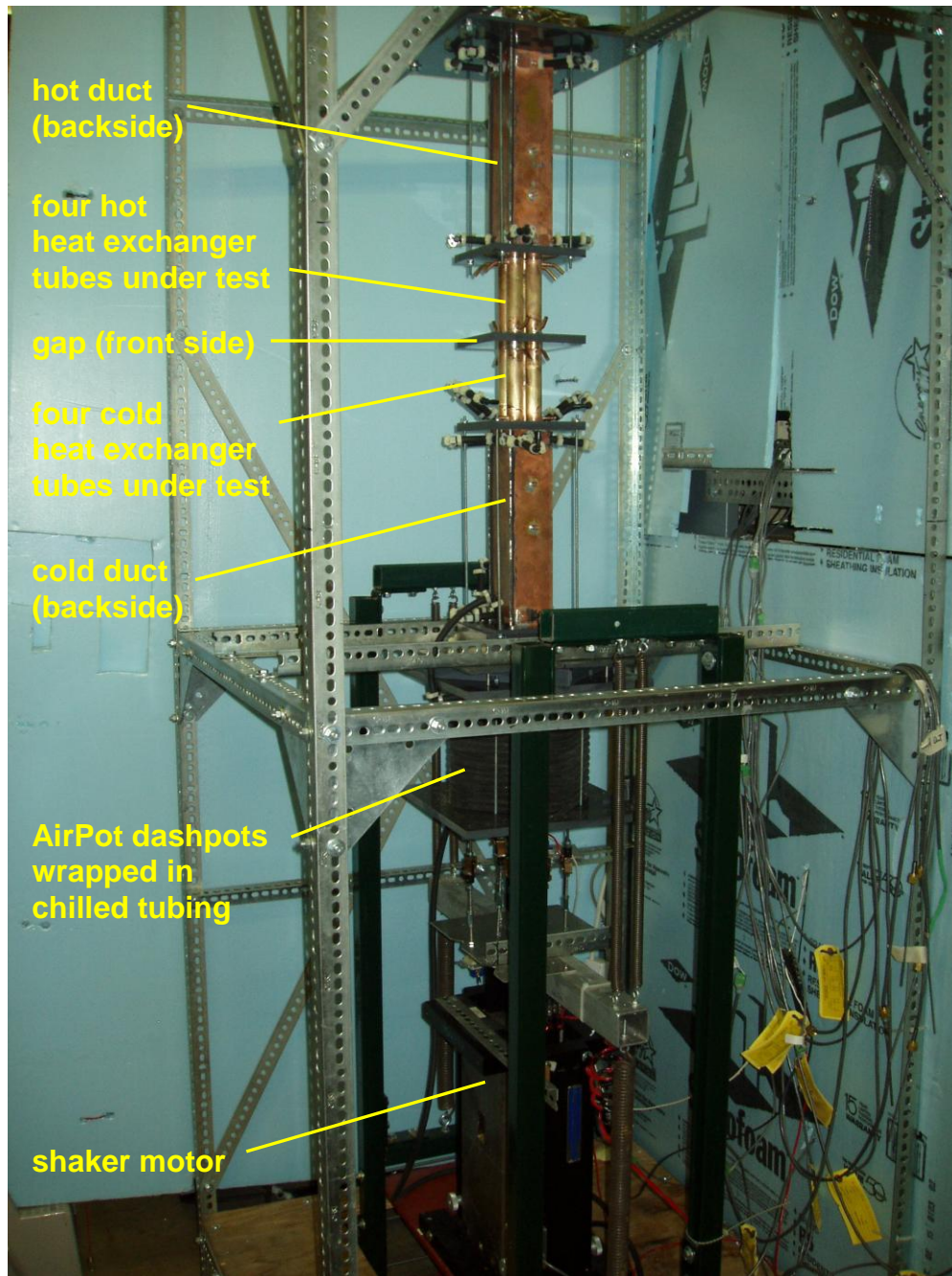
Figure 1. Overall layout of the oscillating flow heat exchange experiment. The shaker motor and AirPot dashpots drive oscillating air flow between four hot and four cold heat exchanger tubes under test. The heat transfer coefficient is obtained from the heat transfer and temperature difference between the hot and cold heat exchanger tubes, which contain hot or cold water flowing through periphery of their double walled construction. Hot and cold ducts, on the backsides of the heat exchanger tubes away from the gap, are also hollowed wall and temperature controlled to explore the heat transfer coming from the backsides of the heat exchanger tubes.
