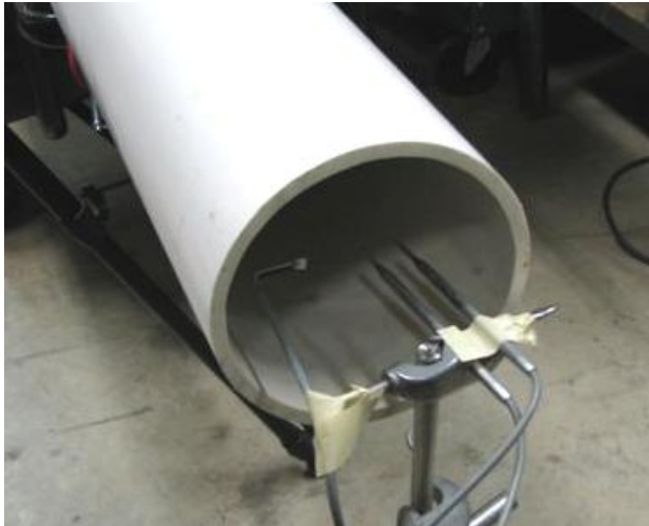
Figure 50. Small surface mount piezoresistive silicon pressure sensor (Intersema MS5412) at the end of a shock wave tube, on the left side of the tube on the end of a bent gray cable, along with a pair of high frequency lab-grade Bruel & Kjaer 1/8" condenser microphones on the right side of the tube.
