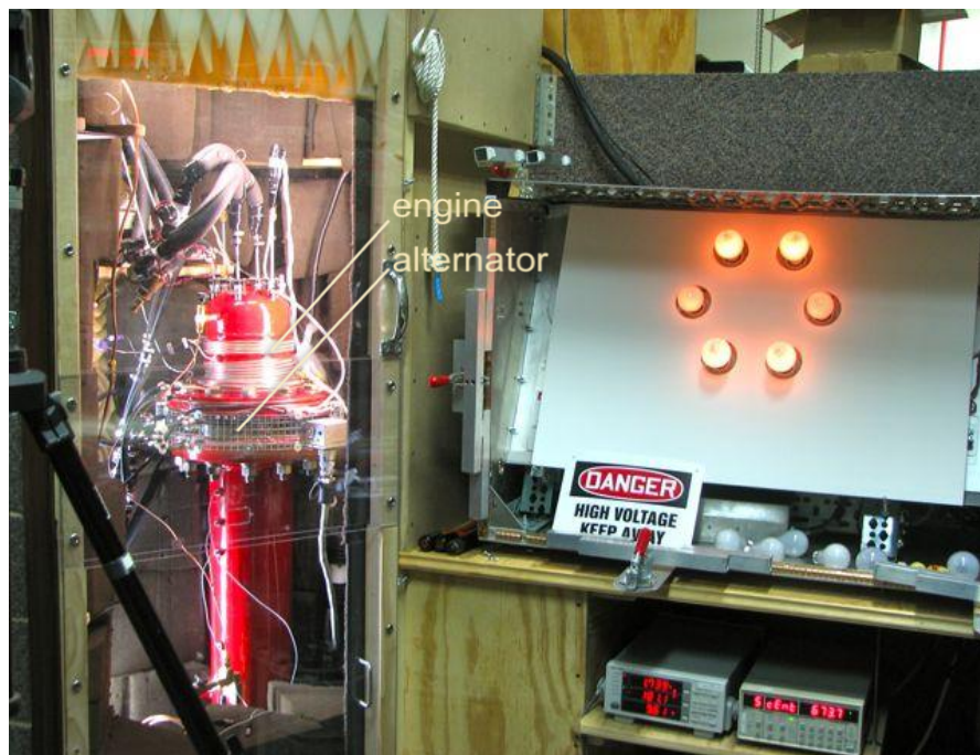
Figure 1. Laboratory prototype engine and alternator, on the left, generating electricity to light the six bulbs on the right.
