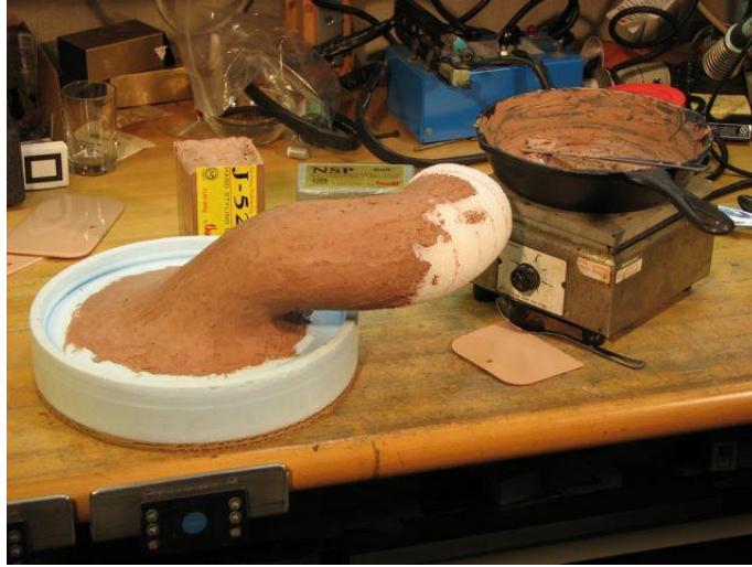
Figure 52. Trombone exit horn foam core in the process of receiving a professional hard modeling clay. A hot plate melts the clay. The blue foam was machined in a lathe to form a 10" flange with an O-ring groove.
