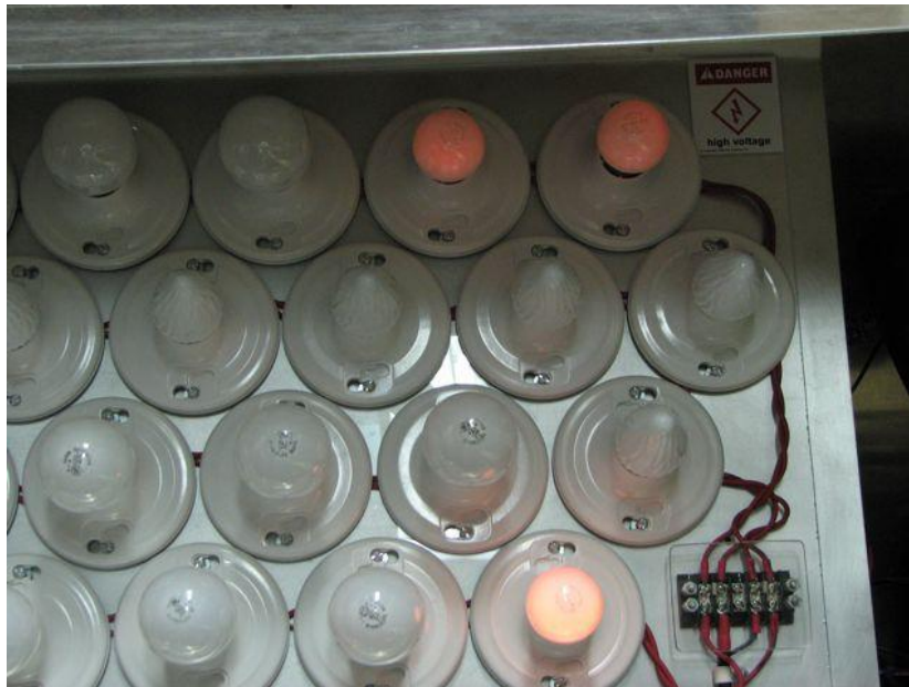
Figure 27. Glowing bulbs from 7 W of generated electricity, at 16.8 kPa acoustic amplitude. The maximum power generated for this run was 10 W at 19.1 kPa.
