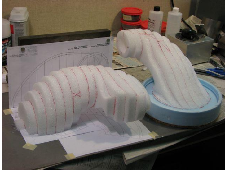
Figure 55. Foam cores for the tuba entry horn and tuba exit horn, before smoothing and the application of clay.
