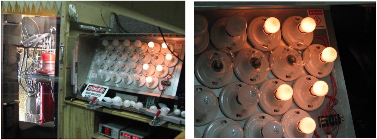
Figure 39. Lighting six 15 W 120 V bulbs with 37 W at 106 V. Three pairs of 15 W bulbs are each in series with higher wattage (lower resistance) bulbs, the three series strings connected in parallel. The 15 W bulbs therefore receive most of the output power.
