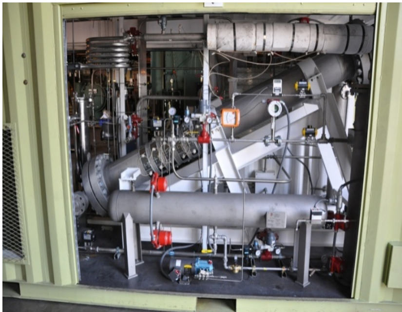
Figure 57 – The PRFC Process Development Unit (PDU) for the Conversion of Syngas to Synthetic Diesel Fuel
