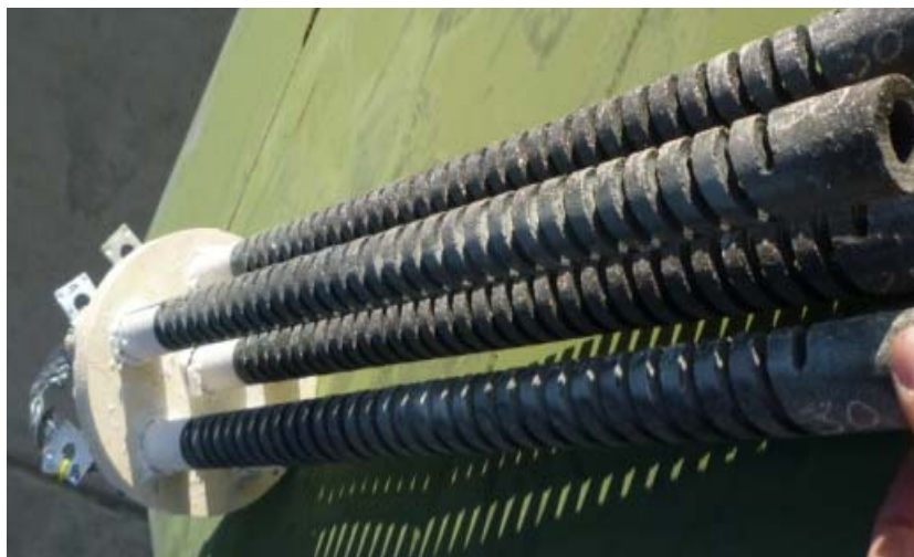
Figure 9 – Sunexus SRI Heater constructed of six Starbar® elements
