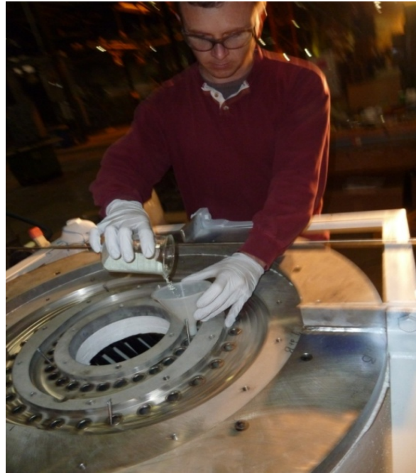
Figure 18 – Catalyst Loading into the Sunexus Reformer SR1
