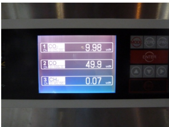
Figure 25 – Infrared Detector (real time CO 2 , CO, CH 4 )
