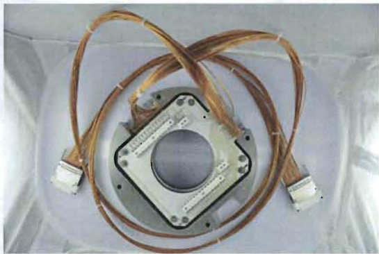
Figure 7. This picture shows the harp mounted in its instrument carrier prior to its installation on the bottom of the insert.
