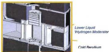
Fig. 2. Schematic design of the new lower tier hydrogen cold source part of the new Lujan target moderator assembly.
