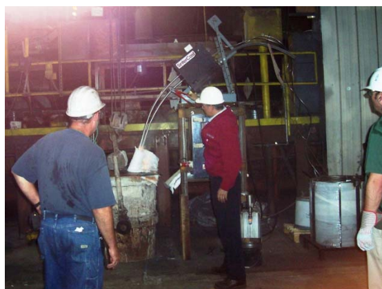
Figure 5.1.3.4 - SinterCast System in the Foundry with Wire Feeder.
