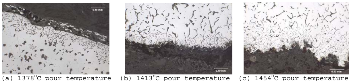
Figure 5.1.3.8 - Typical unetched microstructures of the surfaces of the thick sections from the cast CG iron cylinder blocks poured by different temperatures showing a very thin "skin" that increased in thickness with increasing pouring temperature.
