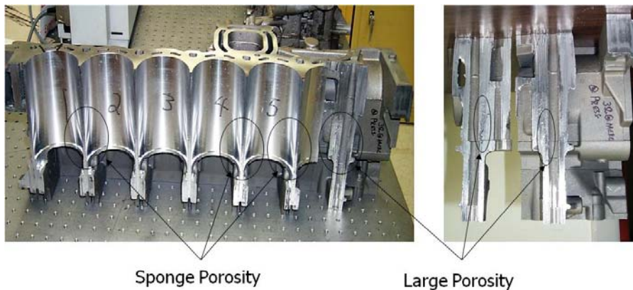
Figure 4.1.5 - Inspection of sectioned Block
