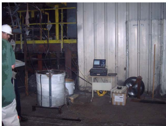
Figure 5.1.3.4 - SinterCast System in the Foundry with Wire Feeder.
