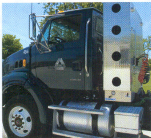
SWACO had one of its fleet trucks retrofitted with a dual-fuel system powered by CNG and biodiesel. The 300 cfm CO 2 wash system being installed in Phase I will produce up to 650 gallons/day of diesel equivalent energy content CNG.
