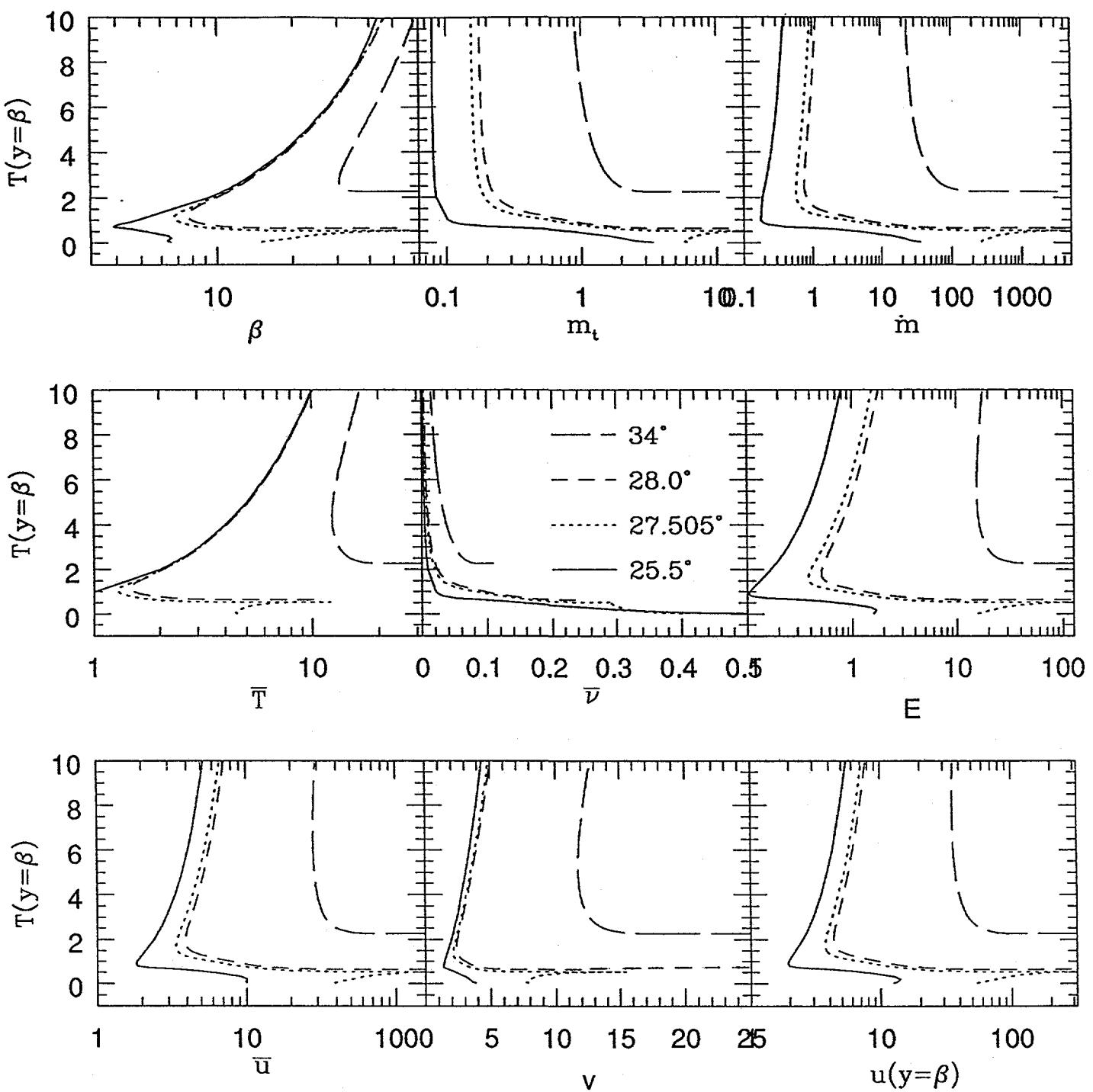
Figure 2: The variations of  $\beta$ ,  $m_t$ ,  $\bar{m}$ ,  $\bar{T}$ ,  $\bar{v}$ ,  $E$ ,  $\bar{u}$ ,  $v$ , and  $u(y=\beta)$  with  $T(y=\beta)$  for  $\phi=25.5^\circ, 27.505^\circ, 28^\circ$  and  $34^\circ$  when  $r=1$ ,  $e=e_w=.5$ , and  $\Delta=.414$ .
