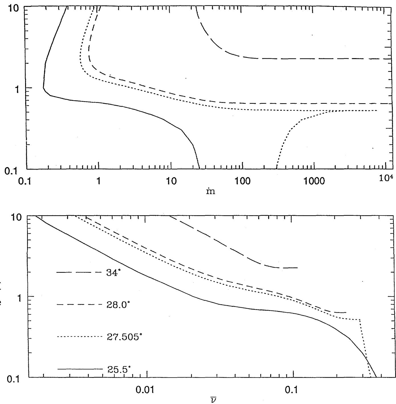
Figure 3: The variations of  $\dot{m}$ , and  $\bar{v}$  with  $T(y=\beta)$  for  $\phi=25.5^\circ, 27.505^\circ, 28^\circ$  and  $34^\circ$  when  $r=1$ ,  $e=e_w=.5$ , and  $\Delta=.414$ .
