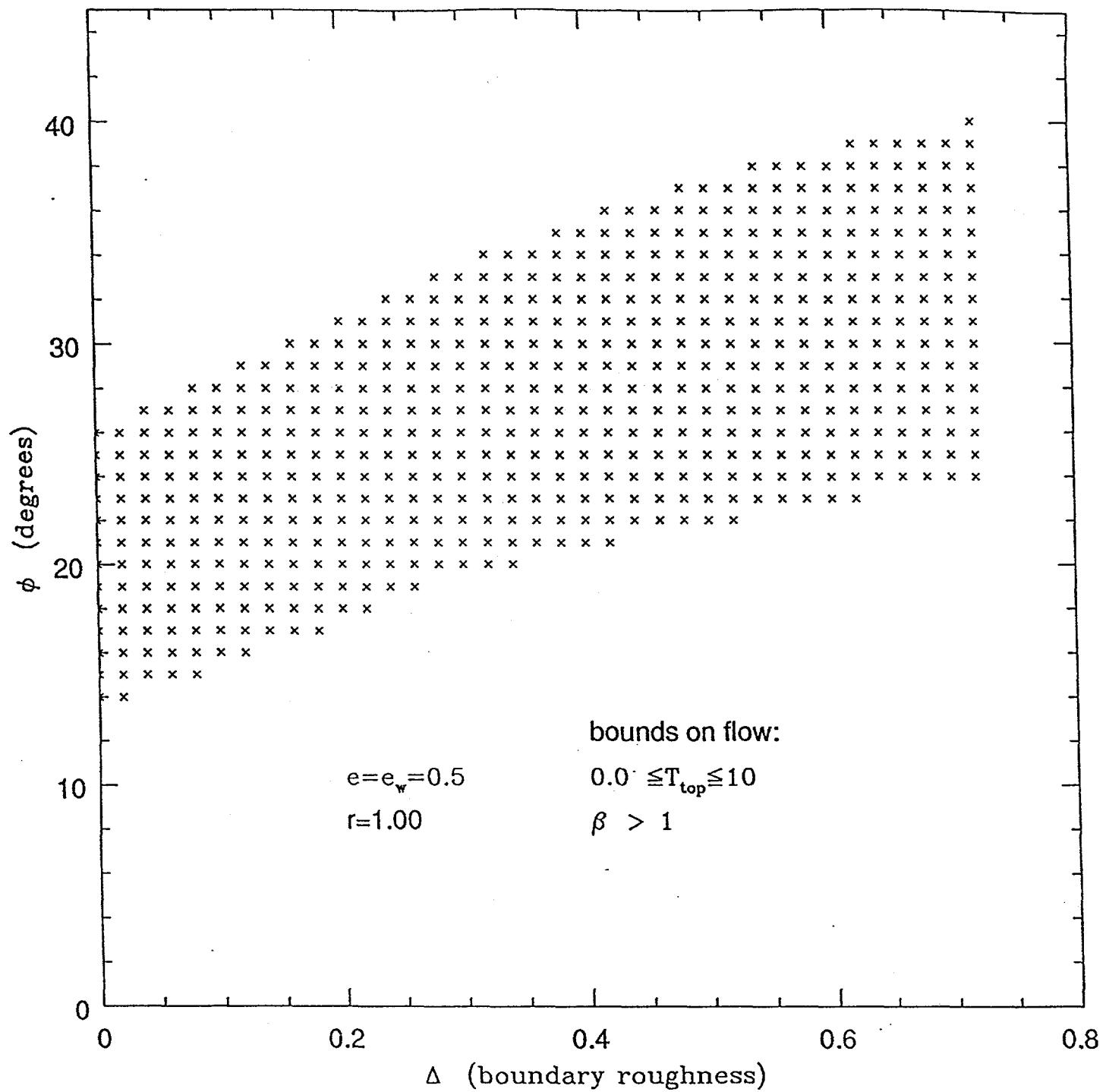
Figure 1: The area in the  $\phi$ - $\Delta$  plane in which steady, fully developed, gravity driven flows are possible when  $r=1$ ,  $e=e_w=.5$ , and  $0 < \Delta < .732$ .
