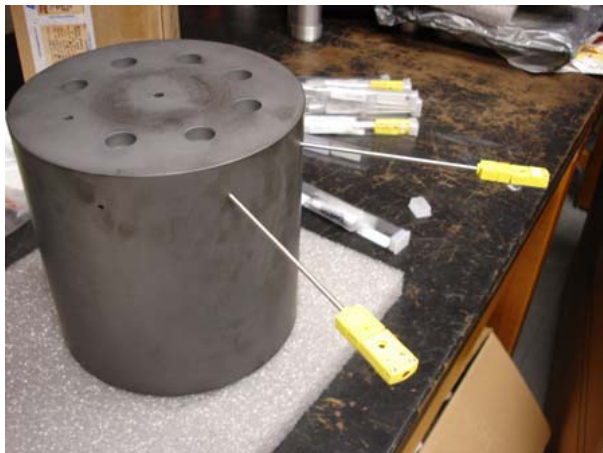
Figure 15. Photograph of the silicon carbide block showing sample and blackbody cavities and two of eight thermocouples inserted.
