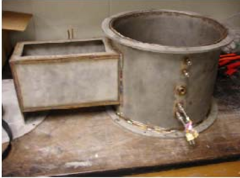
Figure 21. External view of optics chamber with installed thermocouple and stepper motor feed-throughs.
