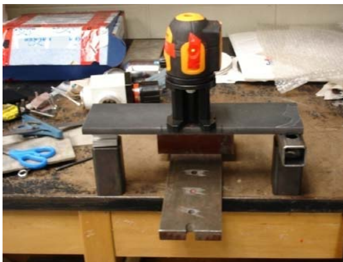
Figure 30. Laser installation for aligning the rotating platform.
