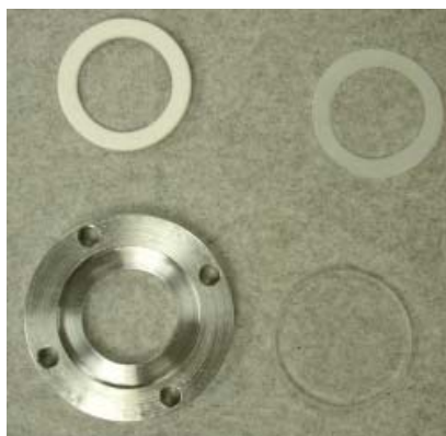
Figure 18. CaF 2 window, aluminum window holder, and Teflon rings.
