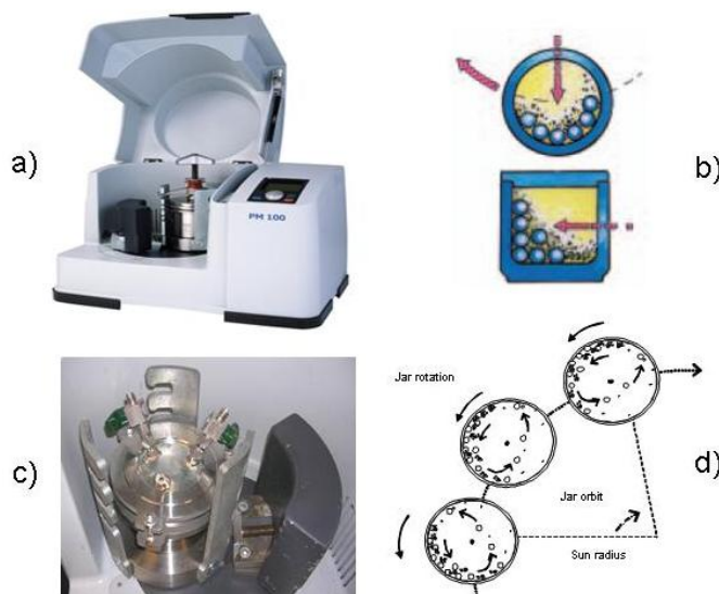
Figure 3.4.1. (a) Jar shown mounted on disc with counter weight (b) Representation of motion within the jar (c) Planetary ball mill jar (reactor) mounted on sun disc (d) Motion of balls and powder in the moving jar.
