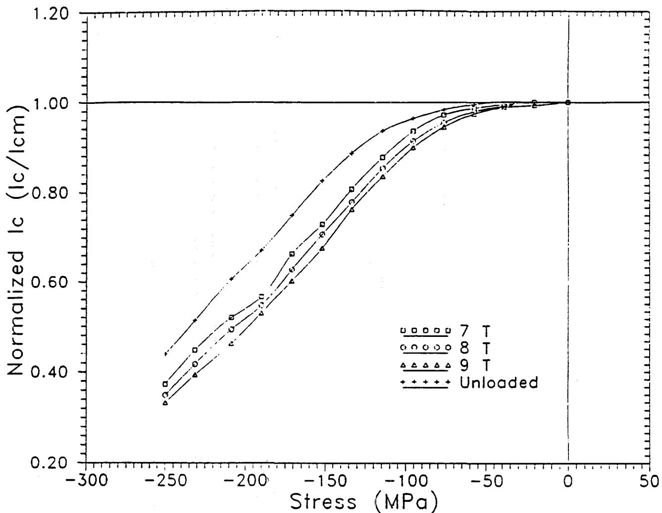
Fig. 2. Internal tin process  $\text{Nb}_3\text{Sn}$   $I_c$ -vs-stress curves at 7, 8, and 9 T. The critical current has been normalized by its maximum value,  $I_{cm}$ . The "Unloaded" data points indicate the measured  $I_c$  at 9 T after unloading the sample from the indicated stress level.
