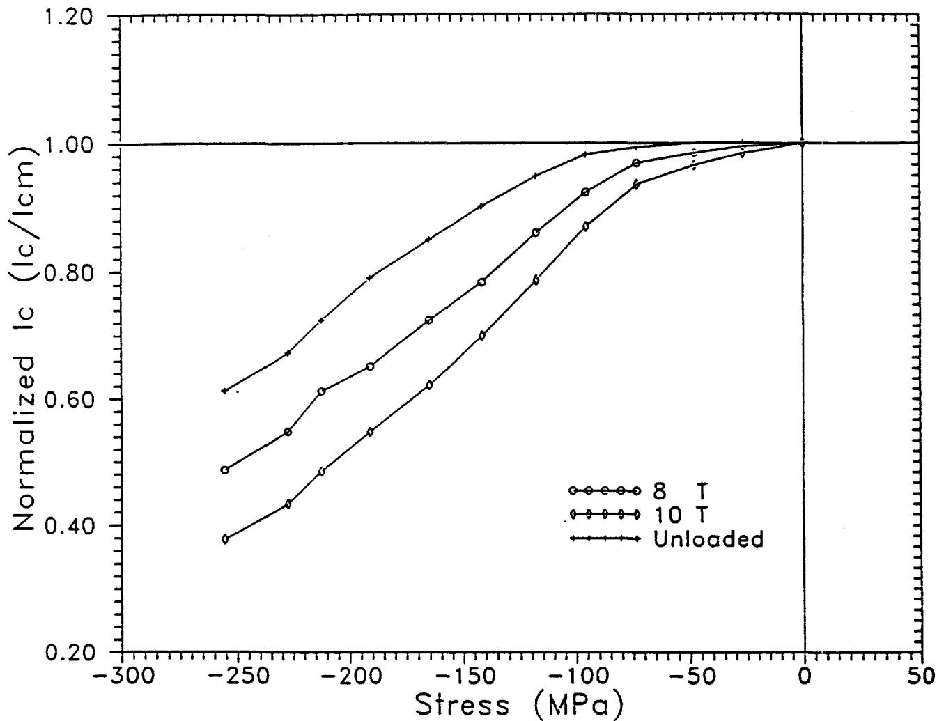
Fig. 1. Bronze process  $\text{Nb}_3\text{Sn}$   $I_c$ -vs-stress curves at 8 and 10 T. The critical current has been normalized by its maximum value,  $I_{cm}$ . The "Unloaded" data points indicate the measured  $I_c$  at 10 T after unloading the sample from the indicated stress level.
