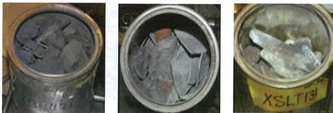
Figure 6. Material Unacceptable for Cementation
