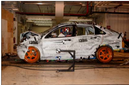
90° 30 MPH Front Fixed Barrier Impact
