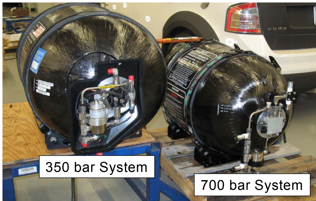
Figure TDV9-2: TDV9 700 Bar Tank Compared to 350 bar Tank
