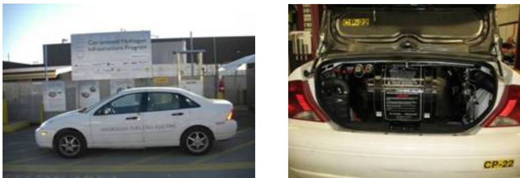
Figure TDV9-1: TDV9 700 bar Fuel System Demonstrator
