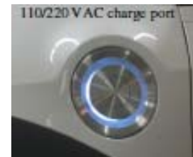
Fig. TDV7-2: 110/220 VAC Charge Port
