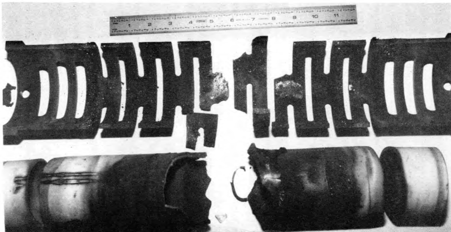
Fig. 4. Failed aluminum oxide muffle tube and damaged heating elements.
