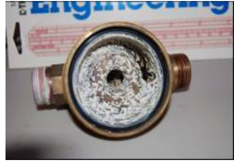
Figure 2-36: Pump impeller chamber
