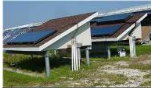
Figure 2-17: The solar collectors are mounted on a nearby roof mock up, with the ICS system in the rear top
