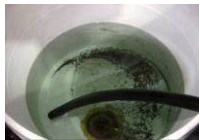
Figure 2-44: Effects of flushing with vinegar and the Residue of internal heat exchanger mineral deposits and corrosion
